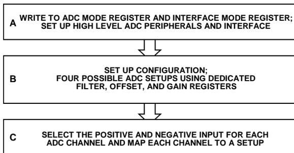
Figure 3. Configuration Flow
