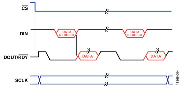
Figure 4. Continuous Conversion Mode
