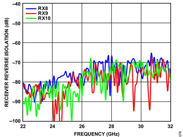
Figure 70. Receiver Reverse Isolation (RX8, RX9, and RX10) vs. Frequency
