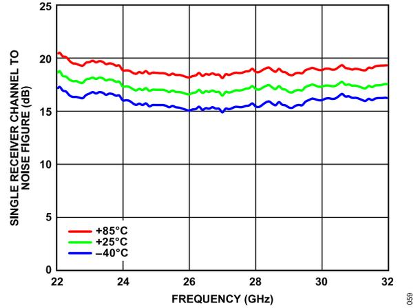
Figure 55. Single Receiver Channel to RF Noise Figure vs. Frequency at Various Temperatures at Maximum Gain, All 16 Channels Active
