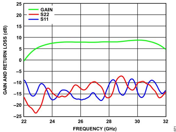
Figure 43. Single Channel Receiver to RF Gain and Return Loss vs. Frequency at Maximum Gain
