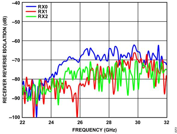
Figure 66. Receiver Reverse Isolation (RX0, RX1, and RX2) vs. Frequency
