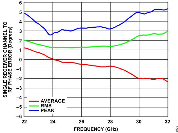
Figure 52. Single Receiver Channel to RF Phase Error vs. frequency for Peak, Average, and RMS Error
