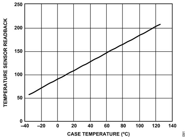
Figure 75. Temperature Sensor Readback vs. Case Temperature
