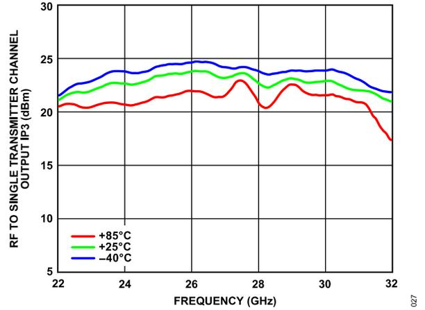
Figure 22. RF to Single Transmitter Channel Output IP3 (OIP3) vs. Frequency at Various Temperatures at Maximum Gain
