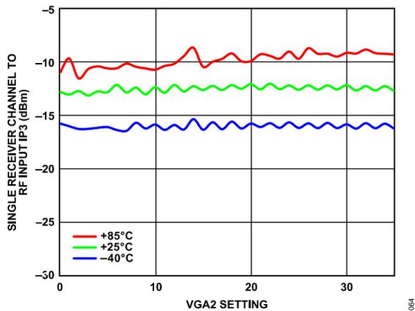
Figure 60. Single Receiver Channel to RF IIP3 vs. DVGA Setting from 0 to 35 over Various Temperatures at 27 GHz
