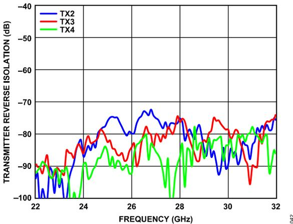
Figure 37. Transmitter Reverse Isolation (TX2, TX3, and TX4) vs. Frequency
