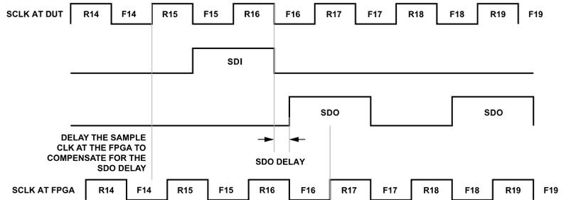
**Figure 81. Using a Delayed SCLK**
