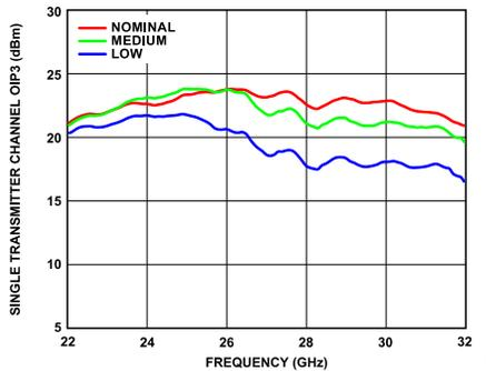
Figure 84. Single Transmitter Channel OIP3 vs. Frequency at Various Power Modes, Maximum Gain
