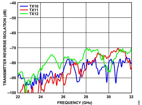
Figure 40. Transmitter Reverse Isolation (TX10, TX11, and TX12) vs. Frequency
