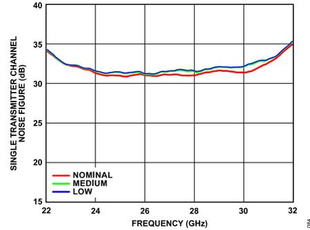
Figure 85. Single Transmitter Channel Noise Figure vs. Frequency at Various Power Modes, Maximum Gain
