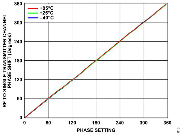
Figure 13. RF to Single Transmitter Channel Phase Shift vs. Phase Setting from 0 to 360 Degrees over Various Temperatures at 27 GHz, Set to Maximum Gain
