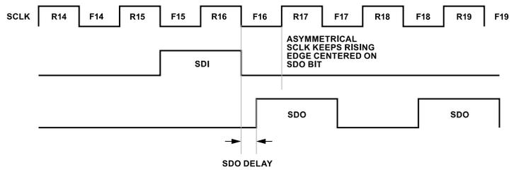
**Figure 80. Using Asymmetric Clock Pulses**
