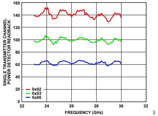
Figure 32. Single Transmitter Channel Power Detector Readback vs. Frequency at Various Detector Range Settings at 27 GHz, Set to Maximum Gain, Input Power = 5 dBm
