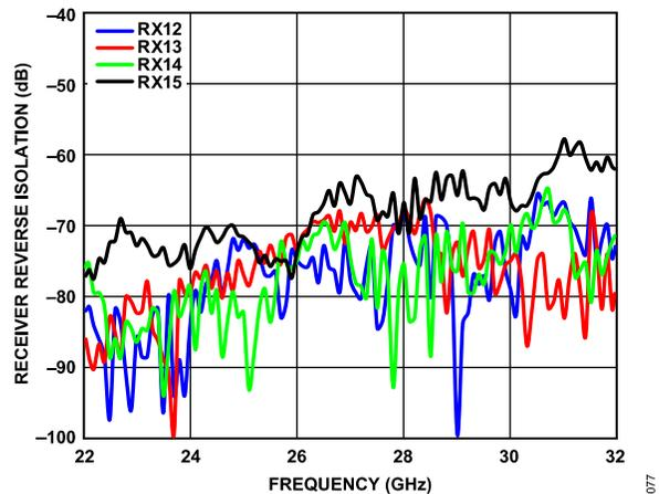
Figure 71. Receiver Reverse Isolation (RX12, RX13, RX14, and RX15) vs. Frequency
