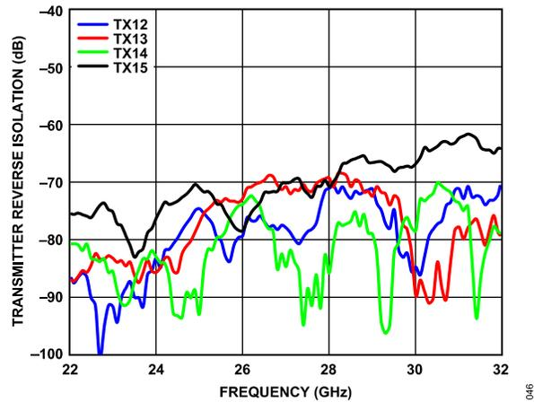
Figure 41. Transmitter Reverse Isolation (TX12, TX13, TX14, and TX15) vs. Frequency
