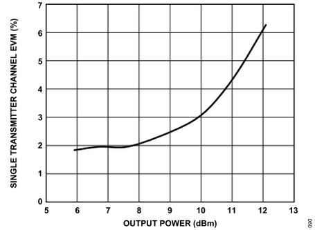
Figure 91. Single Transmitter Channel EVM vs. RF Output Power at Maximum Gain
