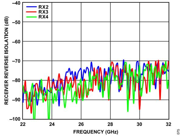
Figure 69. Receiver Reverse Isolation (RX2, RX3, and RX4) vs. Frequency
