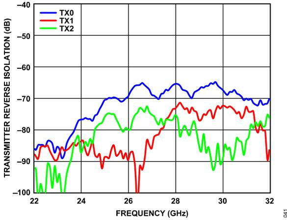
Figure 36. Transmitter Reverse Isolation (TX0, TX1, and TX2) vs. Frequency
