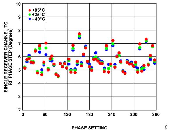
Figure 51. Single Receiver Channel to RF Phase Step vs. Phase Setting from 0 to 360 over Various Temperatures at 27 GHz, Set to Maximum Gain, Nominal Step = 5.625 Degrees
