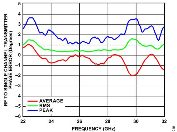
Figure 16. RF to Single Channel Transmitter Phase Error vs. Frequency for Peak, Average, and RMS Error
