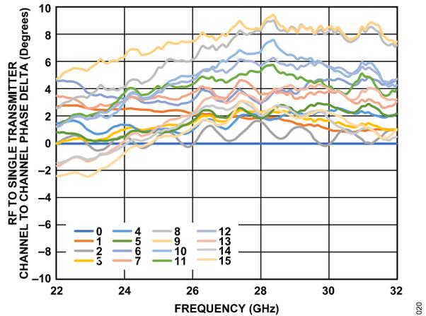
Figure 17. RF to Single Transmitter Channel to Channel Phase Delta vs. Frequency at Maximum Gain
