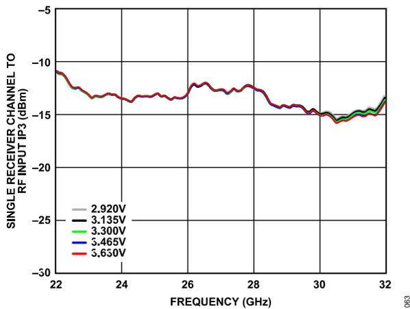
Figure 59. Single Receiver Channel to RF IIP3 vs. Frequency at Various Supply Voltages at Maximum Gain
