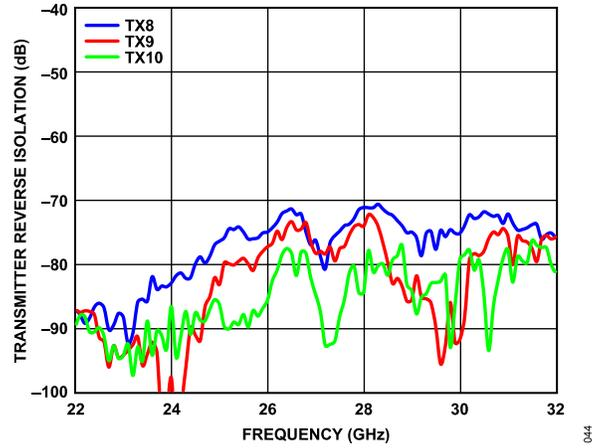
Figure 39. Transmitter Reverse Isolation (TX8, TX9, and TX10) vs. Frequency
