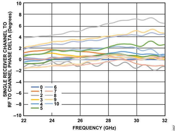
Figure 53. Single Receiver Channel to RF to Channel Phase Delta Frequency at Maximum Gain
