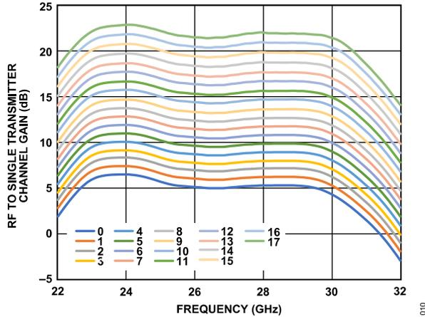
Figure 7. RF to Single Transmitter Channel Gain vs. Frequency at Various DVGA 2 Settings from 0 to 17
