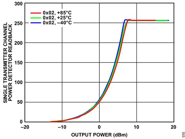
Figure 30. Single Transmitter Channel Power Detector Readback vs. Output Power at Various Temperatures at 27 GHz, Set to Maximum Gain, Detector Range Set to 0x02
