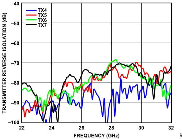
Figure 38. Transmitter Reverse Isolation (TX4, TX5, TX6, and TX7) vs. Frequency
