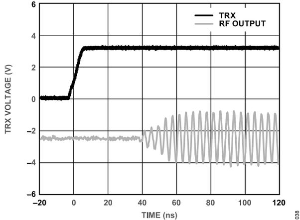
Figure 33. Receiver to Transmitter Mode Switching Time
