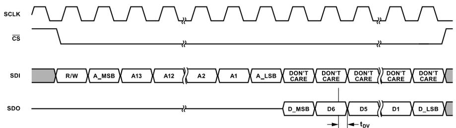
Figure 77. Timing Diagram for Analog Devices Standard SPI Register Read, 4-Wire Mode
