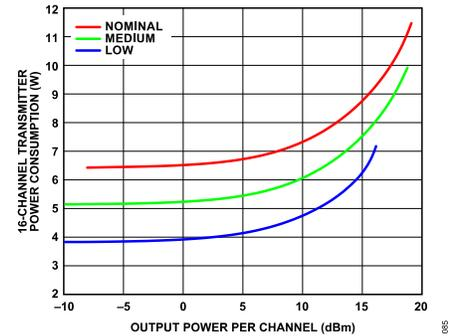
Figure 86. 16-Channel Transmitter Power Consumption vs. Output Power per Channel, Maximum Gain
