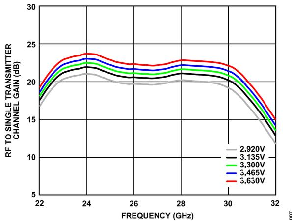
Figure 4. RF to Single Transmitter Channel Gain vs. Frequency at Various Supply Voltages at Maximum Gain
