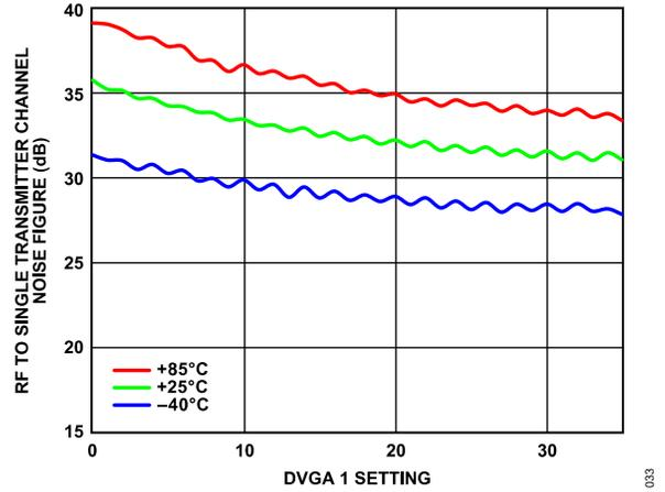
Figure 28. RF to Single Transmitter Channel Noise Figure vs. DVGA 1 Setting from 0 to 35 over Various Temperatures at 27 GHz
