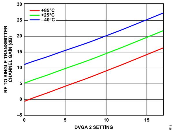
Figure 9. RF to Single Transmitter Channel Gain vs. DVGA 2 Setting from 0 to 17 over Various Temperatures at 27 GHz
