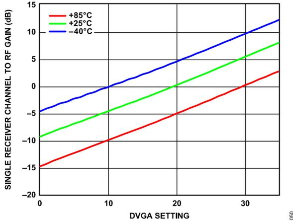
Figure 46. Single Receiver Channel to RF Gain vs. DVGA Setting from 0 to 35 over Various Temperatures at 27 GHz
