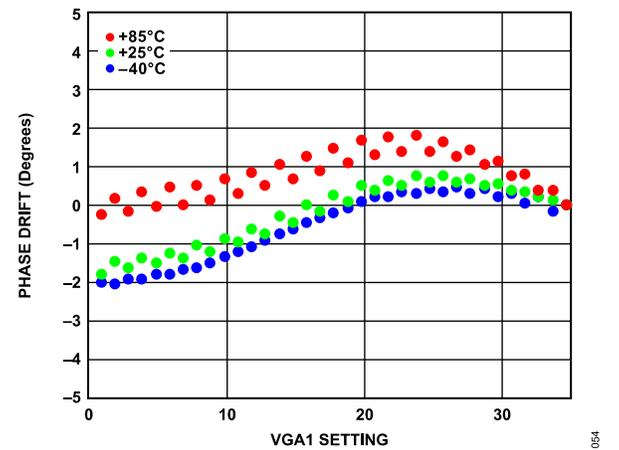
Figure 50. Single Receiver Channel to RF Phase Drift Setting from 0 to 35 over Various Temperatures at 27 GHz
