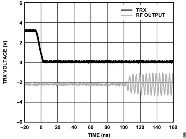
Figure 63. Transmitter to Receiver Mode Switching Time
