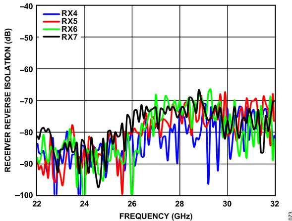
Figure 67. Receiver Reverse Isolation (RX4, RX5, RX6, and RX7) vs. Frequency
