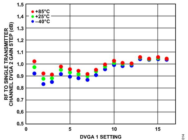
Figure 11. RF to Single Transmitter Channel DVGA 2 Gain Step vs. DVGA 2 Setting from 0 to 17 over Various Temperatures at 27 GHz
