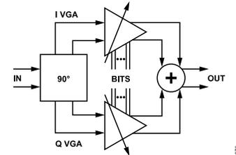
Figure 72. I/Q Vector Modulator Phase Shift Block Diagram
