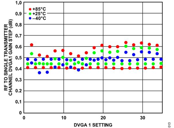
Figure 10. RF to Single Transmitter Channel DVGA1 Gain Step vs. DVGA 1 Setting from 0 to 35 over Various Temperatures at 27 GHz
