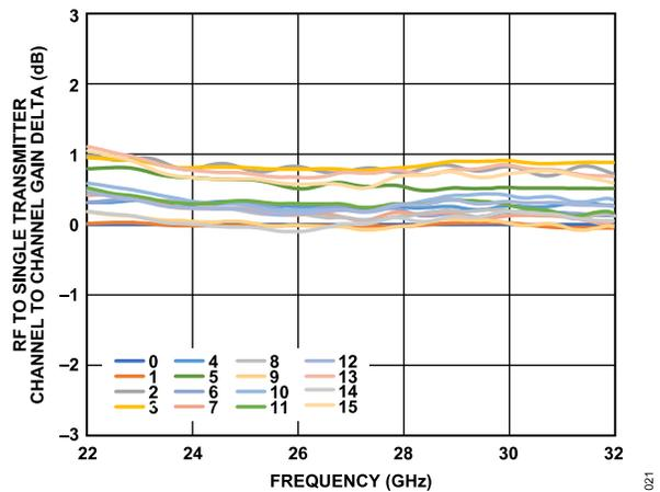
Figure 18. RF to Single Transmitter Channel to Channel Gain Delta vs. Frequency at Maximum Gain
