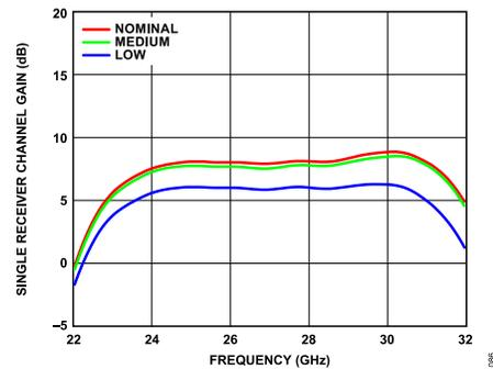
Figure 87. Single Receiver Channel Gain vs. Frequency at Various Temperatures, Maximum Gain
