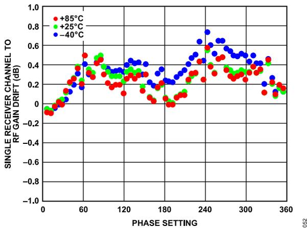
Figure 48. Single Receiver Channel to RF Gain Drift vs. Phase Setting from 0 to 360 Degrees over Temperature at 27 GHz, Set to Maximum Gain
