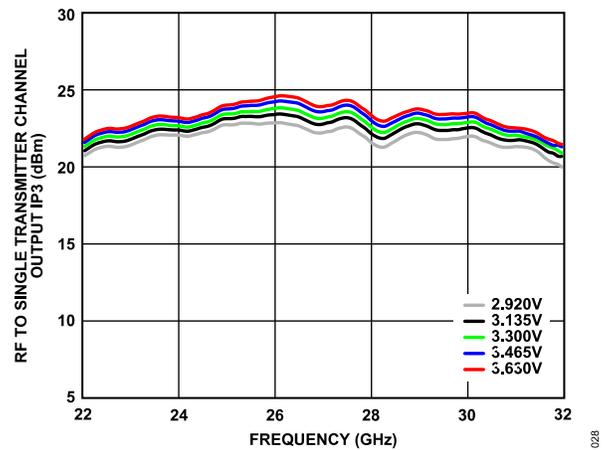
Figure 23. RF to Single Transmitter Channel OIP3 vs. Frequency at Various Supply Voltages at Maximum Gain
