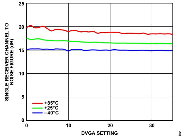
Figure 57. Single Receiver Channel to RF Noise Figure vs. DVGA Setting from 0 to 35 over Various Temperatures at 27 GHz, All 16 Channels Active
