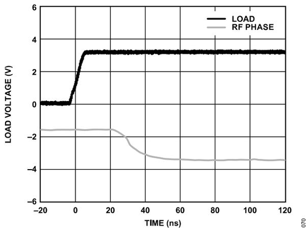
Figure 65. Phase Settling Time
