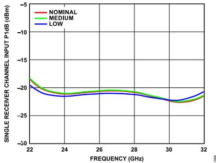
Figure 89. Single Receiver Channel Input P1dB vs. Frequency at Various Temperatures, Maximum Gain
