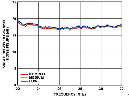
Figure 88. Single Receiver Channel Noise Figure vs. Frequency at Various Temperatures, Maximum Gain
