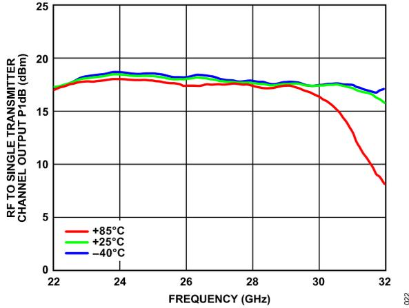
Figure 19. RF to Single Transmitter Channel Output P1dB vs. Frequency at Various Temperatures at Maximum Gain
