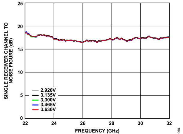
Figure 56. Single Receiver Channel to RF Noise Figure vs. Frequency at Various Supply Voltages at Maximum Gain, All 16 Channels Active
