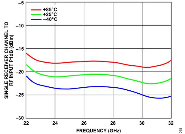
Figure 61. Single Receiver Channel to RF Input P1dB vs. Frequency at Various Temperatures at Maximum Gain
