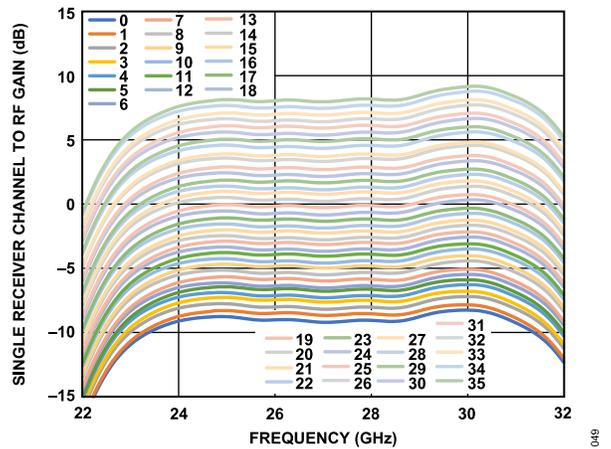
Figure 45. Single Receiver Channel to RF Gain vs. Frequency at Various DVGA Settings from 0 to 35
