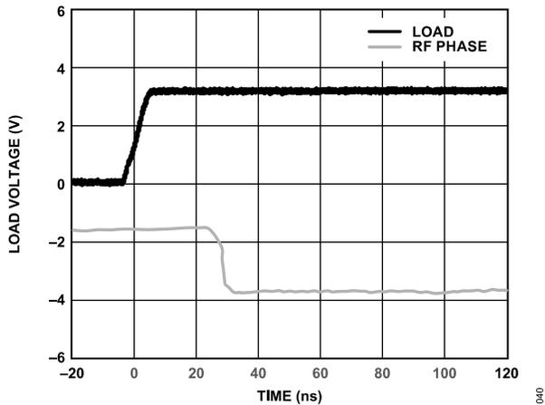
Figure 35. Phase Settling Time
