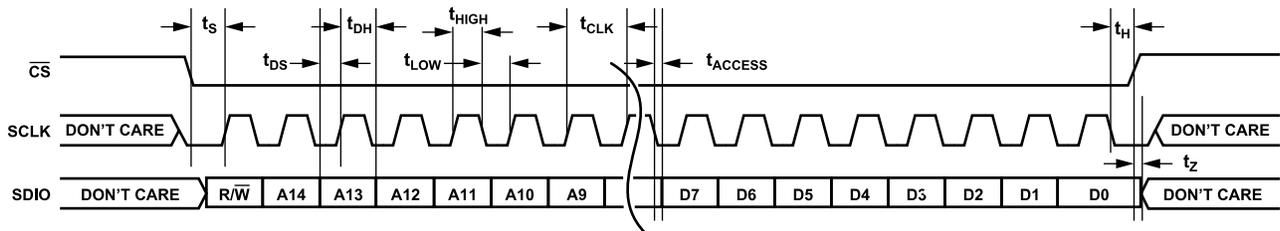
Figure 76. SPI Register Timing Diagram for Analog Devices Standard SPI, MSB First
