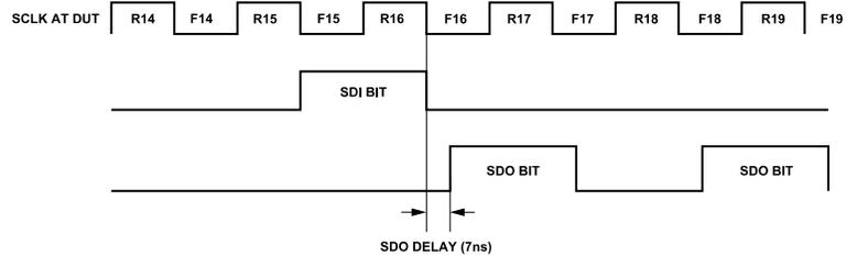
**Figure 79. SDO Delay Timing Diagram**
