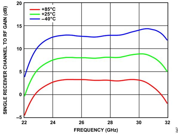
Figure 42. Single Receiver Channel to RF Gain vs. Frequency at Various Temperatures at Maximum Gain
