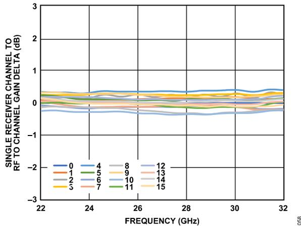
Figure 54. Single Receiver Channel to RF to Channel Gain Delta vs. Frequency at Maximum Gain
