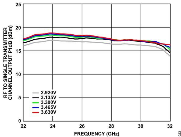
Figure 20. RF to Single Transmitter Channel Output P1dB vs. Frequency at Various Supply Voltages at Maximum Gain
