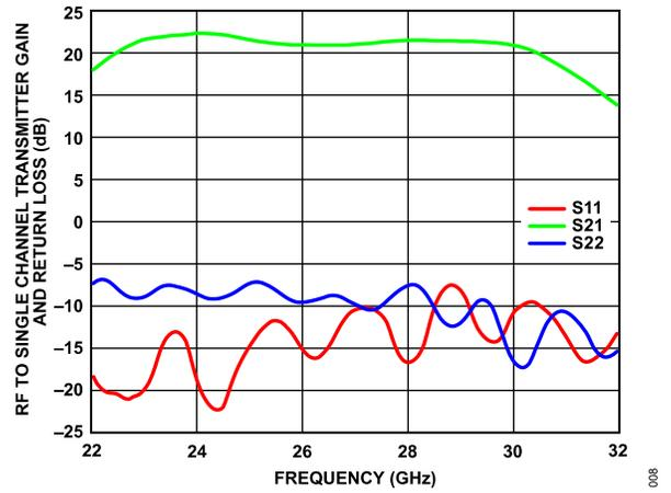
Figure 5. RF to Single Channel Transmitter Gain and Return Loss vs. Frequency at Maximum Gain
