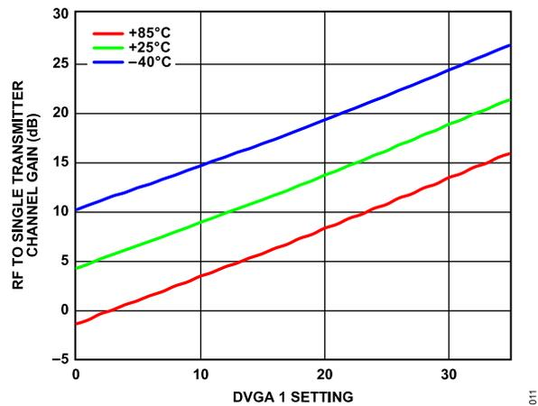
Figure 8. RF to Single Transmitter Channel Gain vs. DVGA 1 Setting from 0 to 35 over Various Temperatures at 27 GHz
