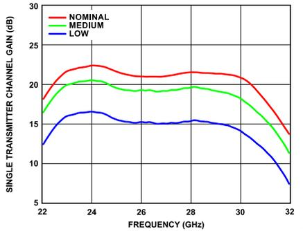
Figure 82. Single Transmitter Channel Gain vs. Frequency at Various Power Modes, Maximum Gain
