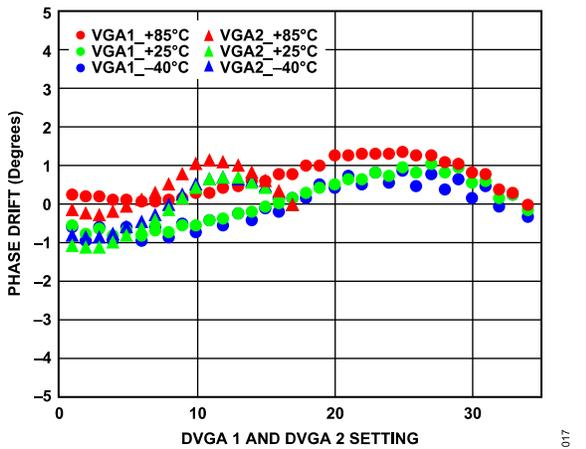
Figure 14. RF to Single Transmitter Channel Phase Drift vs. DVGA 1 and DVGA 2 Setting from 0 to 35 and 0 to 17, over Various Temperatures at 27 GHz
