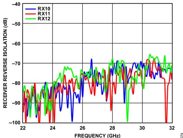
Figure 68. Receiver Reverse Isolation (RX10, RX11, and RX12) vs. Frequency
