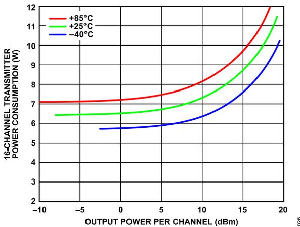
Figure 21. 16-Channel Transmitter Power Consumption vs. Output Power per Channel at Maximum Gain
