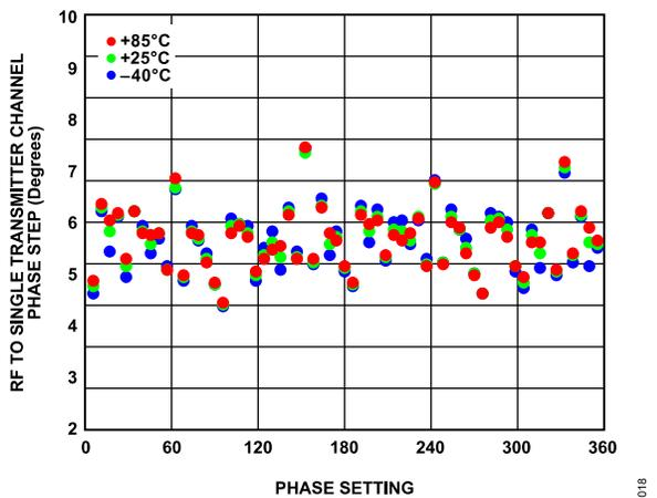
Figure 15. RF to Single Transmitter Channel Phase Step vs. Phase Setting from 0 to 360 over Various Temperatures at 27 GHz, Set to Maximum Gain, Nominal Step 5.625 Degrees
