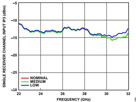
Figure 90. Single Receiver Channel Input IP3 vs. Frequency at Various Temperatures, Maximum Gain
