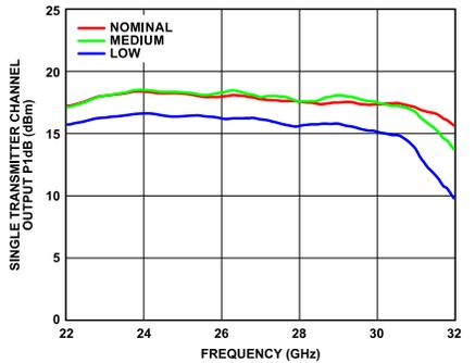
Figure 83. Single Transmitter Channel Output P1dB vs. Frequency at Various Power Modes, Maximum Gain
