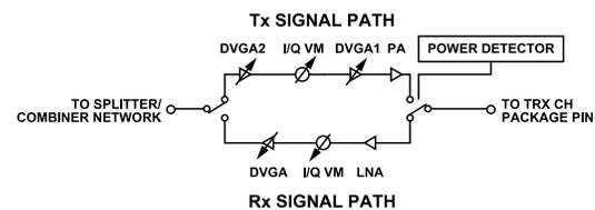
Figure 73. Transmit and Receive Channel Functional Block Diagram
