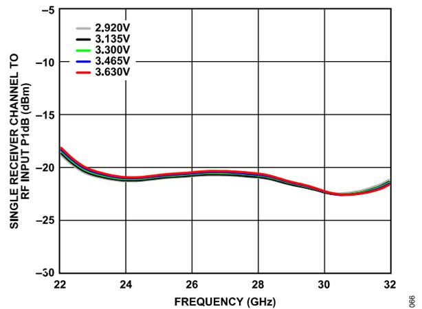
Figure 62. Single Receiver Channel to RF Input P1dB vs. Frequency at Various Supply Voltages at Maximum Gain
