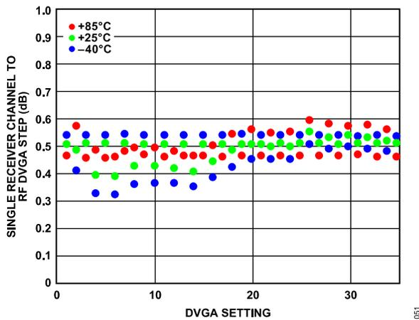
Figure 47. Single Receiver Channel to RF DVGA Step vs. DVGA Setting from 0 to 35 over Various Temperatures at 27 GHz
