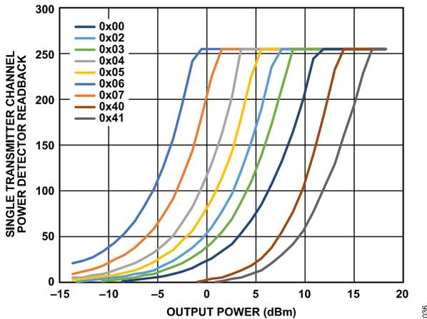
Figure 31. Single Transmitter Channel Power Detector Readback vs. Output Power at Various Detector Range Settings at 27 GHz, Set to Maximum Gain
