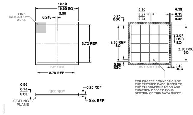
Figure 92. 72-Terminal Land Grid Array [LGA]
