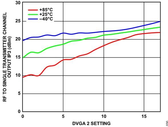
Figure 25. RF to Single Transmitter Channel OIP3 vs. DVGA 2 Setting from 0 to 17 over Various Temperatures at 27 GHz
