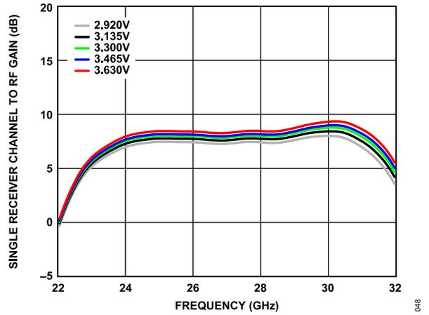
Figure 44. Single Receiver Channel to RF Gain vs. Frequency at Various Supply Voltages at Maximum Gain
