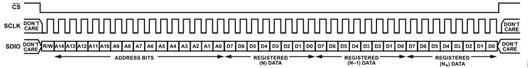
Figure 78. Streaming Mode Write Timing Diagram, MSB First, Address Descending
