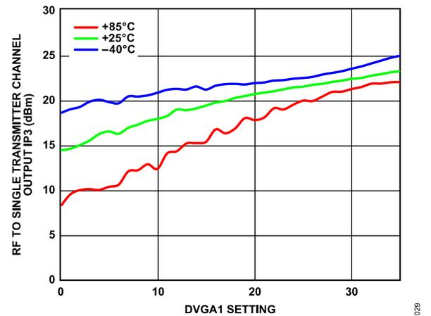
Figure 24. RF to Single Transmitter Channel OIP3 vs. DVGA 1 Setting from 0 to 35 over Various Temperatures at 27 GHz
