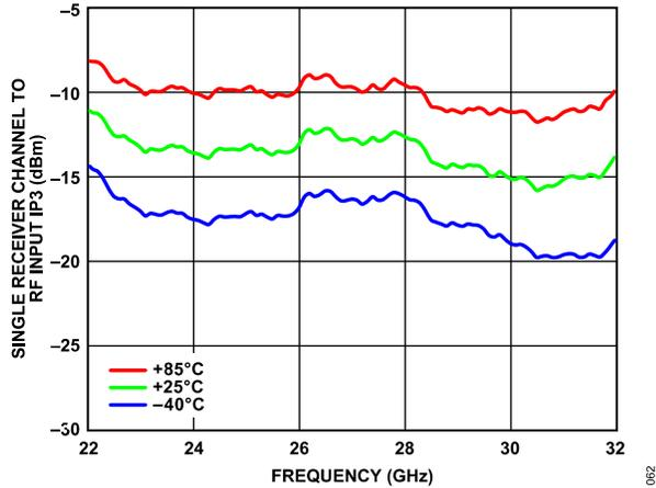
Figure 58. Single Receiver Channel to RF Input IP3 (IIP3) vs. Frequency at Various Temperatures at Maximum Gain
