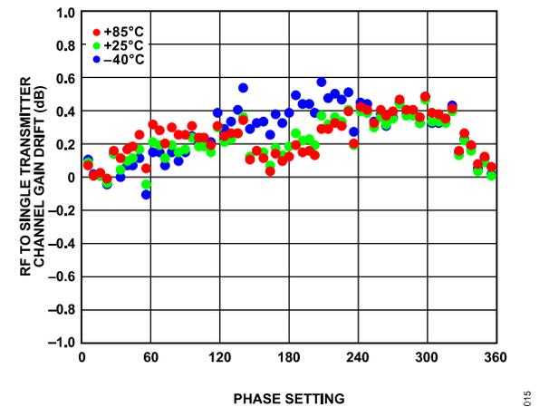
Figure 12. RF to Single Transmitter Channel Gain Drift vs. Phase Setting from 0 to 360 Degrees over Temperature at 27 GHz, Set to Maximum Gain
