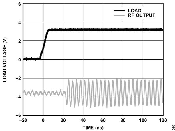
Figure 64. Gain Settling Time
