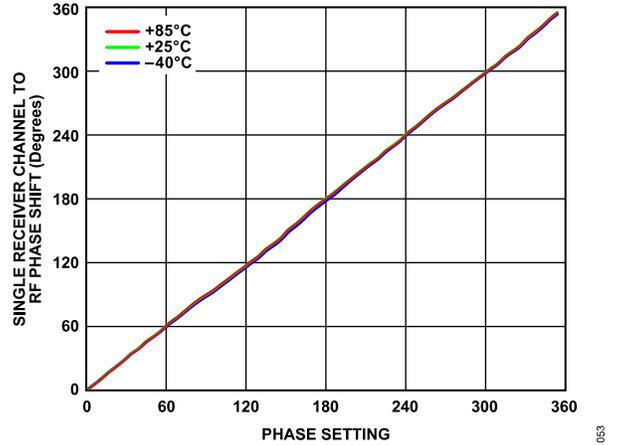
Figure 49. Single Receiver Channel to RF Phase Shift vs. Phase Setting from 0 to 360 Degrees over Various Temperatures at 27 GHz, Set to Maximum Gain
