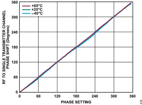
Figure 13. RF to Single Transmitter Channel Phase Shift vs. Phase Setting from 0° to 360° over Various Temperatures at 27 GHz, Set to Maximum Gain
