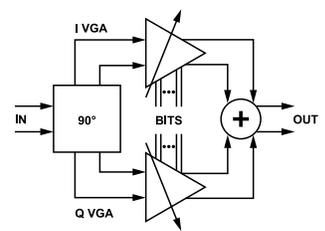
Figure 76. I/Q VM Phase Shift Block Diagram
