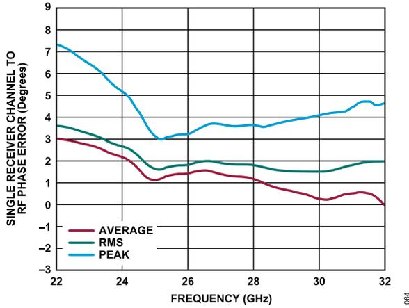
Figure 54. Single Receiver Channel to RF Phase Error vs. Frequency for Peak, Average, and RMS Error
