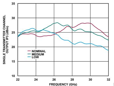
Figure 88. Single Transmitter Channel Output IP3 vs. Frequency at Various Power Modes, Maximum Gain
