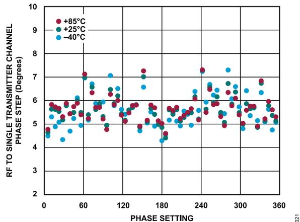
Figure 15. RF to Single Transmitter Channel Phase Step vs. Phase Setting from 0° to 360° over Various Temperatures at 27 GHz, Set to Maximum Gain, Nominal Step 5.625°
