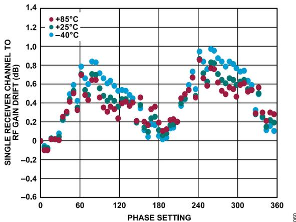
Figure 50. Single Receiver Channel to RF Gain Drift vs. Phase Setting from 0° to 360° over Temperature at 27 GHz, Set to Maximum Gain
