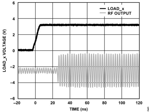
Figure 34. Gain Settling Time
