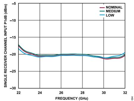
Figure 93. Single Receiver Channel Input P1dB vs. Frequency at Various Temperatures, Maximum Gain
