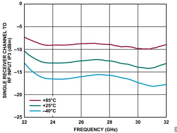
Figure 60. Single Receiver Channel to RF Input IP3 vs. Frequency at Various Temperatures at Maximum Gain
