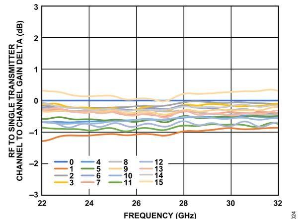
Figure 18. RF to Single Transmitter Channel to Channel Gain Delta vs. Frequency at Maximum Gain, Where Numbers in Legend Are Channel Numbers
