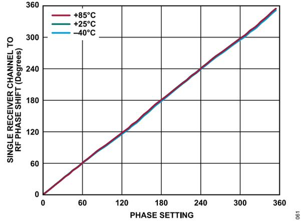
Figure 51. Single Receiver Channel to RF Phase Shift vs. Phase Setting from 0° to 360° over Various Temperatures at 27 GHz, Set to Maximum Gain
