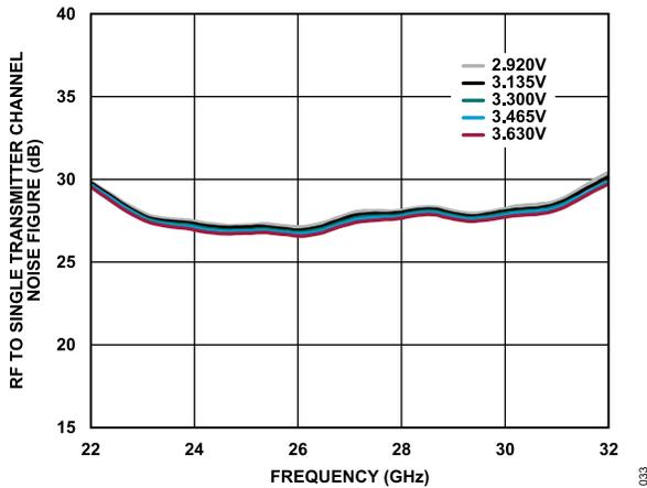
Figure 27. RF to Single Transmitter Channel Noise Figure vs. Frequency at Various Supply Voltages at Maximum Gain
