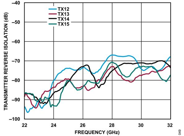
Figure 43. Transmitter Reverse Isolation vs. Frequency for TX12 to TX15
