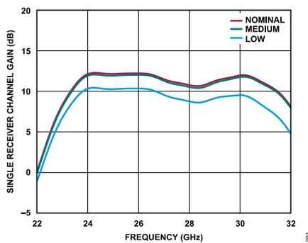
Figure 91. Single Receiver Channel Gain vs. Frequency at Various Temperatures, Maximum Gain
