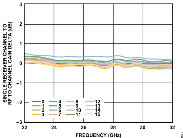
Figure 56. Single Receiver Channel to RF to Channel Gain Delta vs. Frequency at Maximum Gain, Where Numbers in Legend Are Channel Numbers
