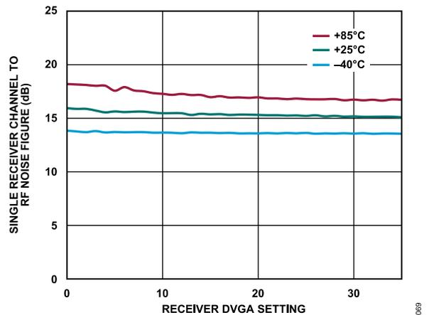
Figure 59. Single Receiver Channel to RF Noise Figure vs. Receiver DVGA Setting from 0 to 35 over Various Temperatures at 27 GHz
