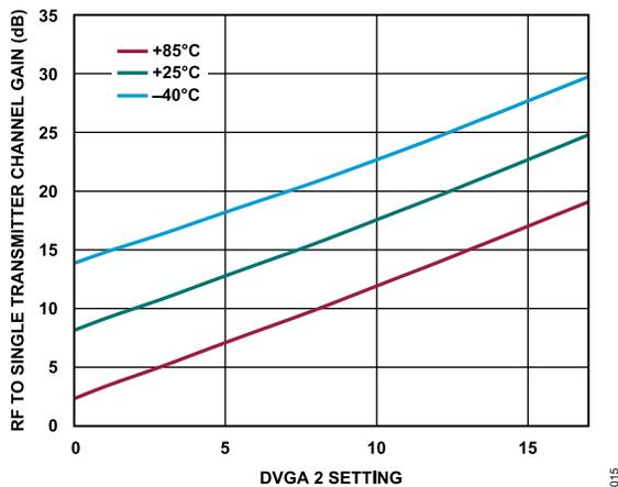
Figure 9. RF to Single Transmitter Channel Gain vs. DVGA 2 Setting from 0 to 17 over Various Temperatures at 27 GHz
