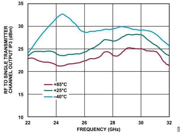
Figure 22. RF to Single Transmitter Channel Output IP3 vs. Frequency at Various Temperatures at Maximum Gain
