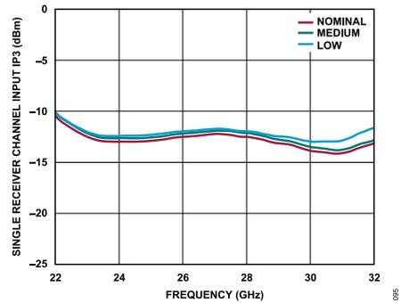
Figure 94. Single Receiver Channel Input IP3 vs. Frequency at Various Temperatures, Maximum Gain
