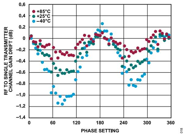
Figure 12. RF to Single Transmitter Channel Gain Drift vs. Phase Setting from 0° to 360° over Temperature at 27 GHz, Set to Maximum Gain
