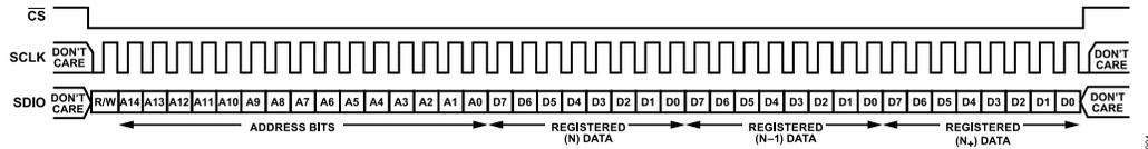
**Figure 82. Streaming Mode Write Timing Diagram, MSB First, Address Descending**
