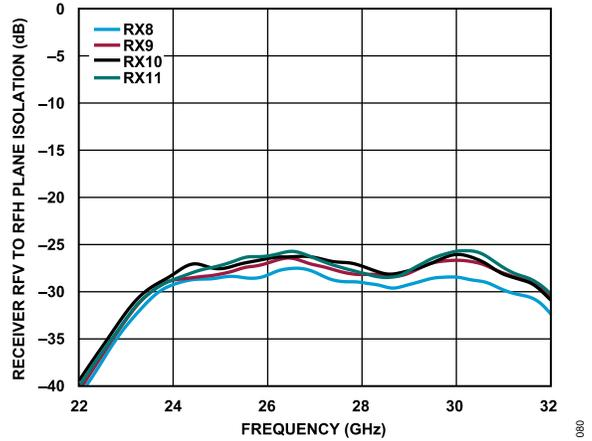
Figure 70. Receiver RFV to RFH Plane Isolation vs. Frequency for Receiver 8 (RX8), Receiver 9 (RX9), Receiver 10 (RX10), and Receiver 11 (RX11)
