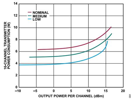
Figure 90. 16-Channel Transmitter Power Consumption vs. Output Power per Channel, Maximum Gain
