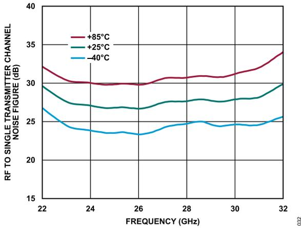
Figure 26. RF to Single Transmitter Channel Noise Figure vs. Frequency at Various Temperatures at Maximum Gain
