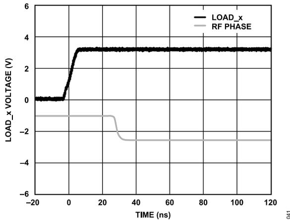
Figure 35. RF Phase Settling Time
