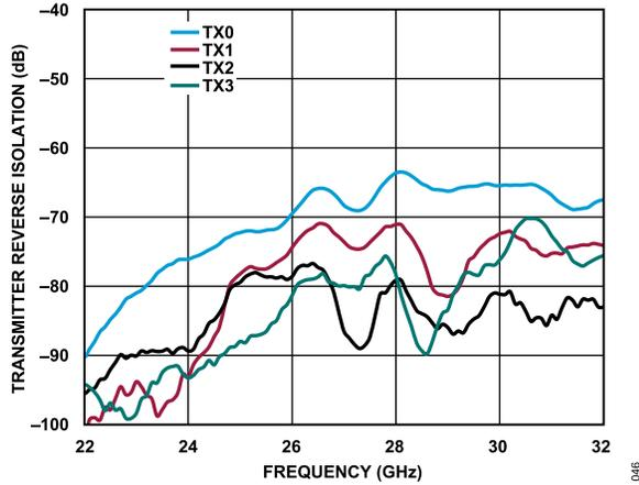
Figure 40. Transmitter Reverse Isolation vs. Frequency for TX0 to TX3
