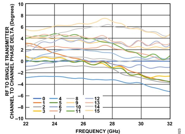
Figure 17. RF to Single Transmitter Channel to Channel Phase Delta vs. Frequency at Maximum Gain, Where Numbers in Legend Are Channel Numbers
