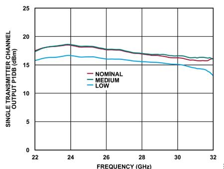
Figure 87. Single Transmitter Channel Output P1dB vs. Frequency at Various Power Modes, Maximum Gain
