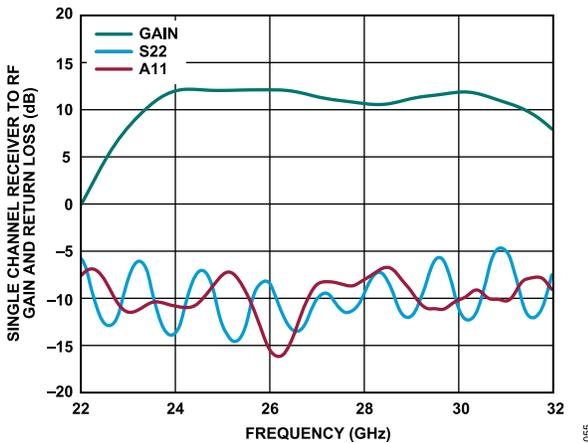
Figure 45. Single Channel Receiver to RF Gain and Return Loss vs. Frequency at Maximum Gain
