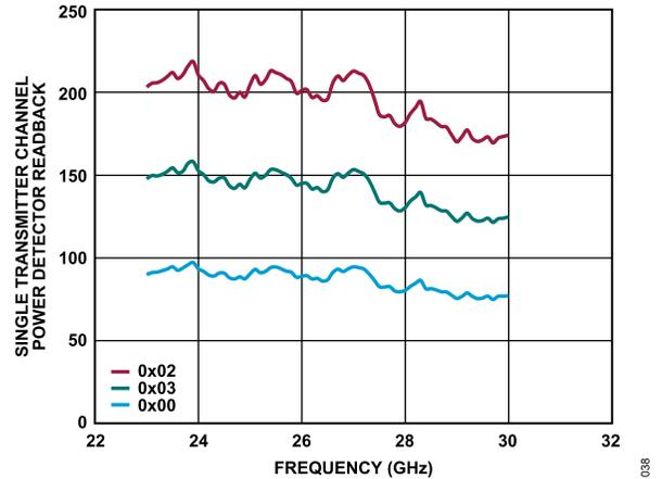
Figure 32. Single Transmitter Channel Power Detector Readback vs. Frequency at Various Detector Range Settings, Set to Maximum Gain, Input Power = 5 dBm
