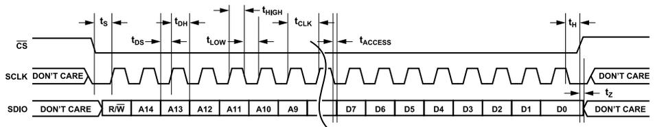
Figure 80. SPI Register Timing Diagram for Standard SPI, MSB First
