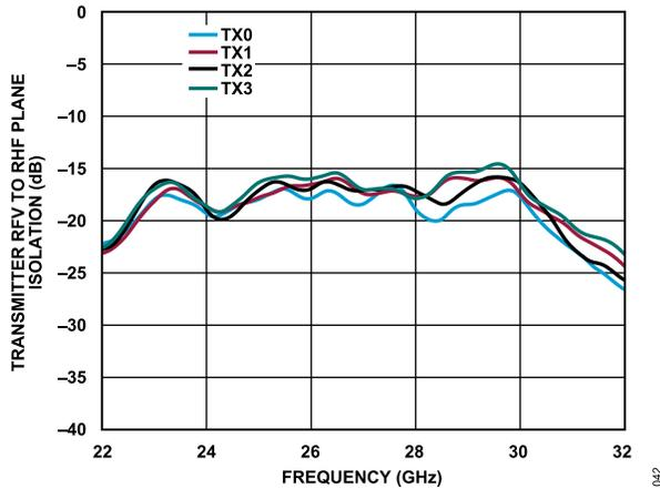
Figure 36. Transmitter RFV to RFH Plane Isolation vs. Frequency for Transmitter 0 (TX0), Transmitter 1 (TX1), Transmitter 2 (TX2), and Transmitter 3 (TX3)
