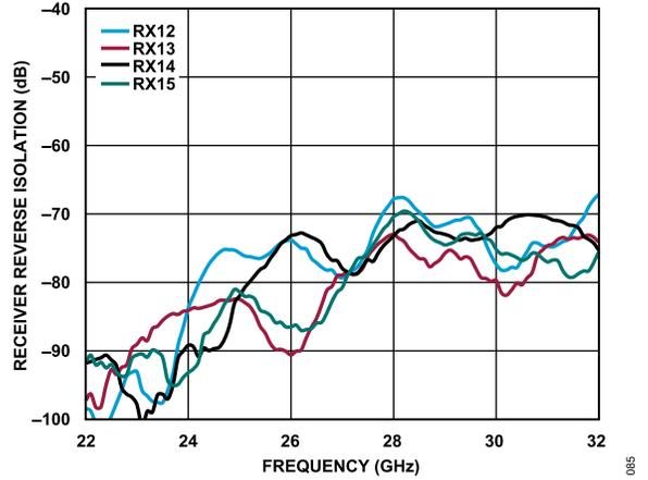
Figure 75. Receiver Reverse Isolation vs. Frequency for RX12 to RX15
