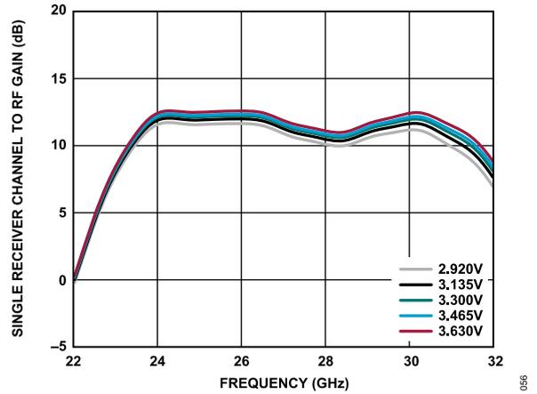
Figure 46. Single Receiver Channel to RF Gain vs. Frequency at Various Supply Voltages at Maximum Gain
