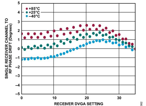
Figure 52. Single Receiver Channel to RF Phase Drift vs. Receiver DVGA Setting from 0 to 35 over Various Temperatures at 27 GHz
