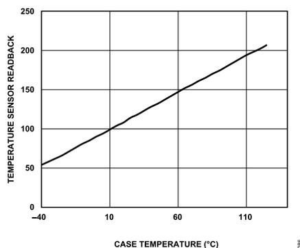
Figure 79. Temperature Sensor Readback vs. Case Temperature
