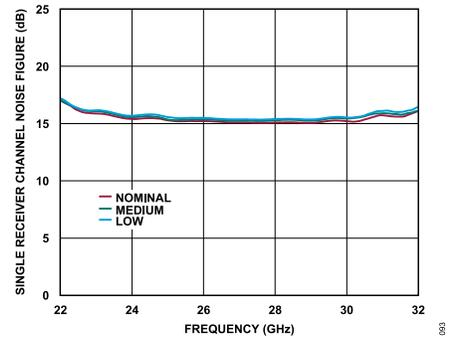
Figure 92. Single Receiver Channel Noise Figure vs. Frequency at Various Temperatures, Maximum Gain
