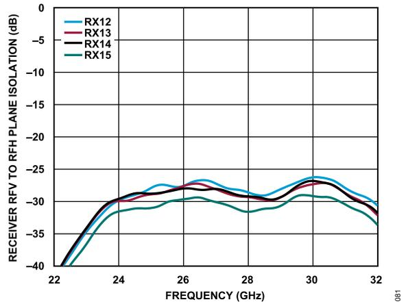
Figure 71. Receiver RFV to RFH Plane Isolation vs. Frequency for Receiver 12 (RX12), Receiver 13 (RX13), Receiver (RX14), and Receiver 15 (RX15)
