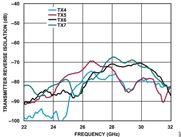
Figure 41. Transmitter Reverse Isolation vs. Frequency for TX4 to TX7
