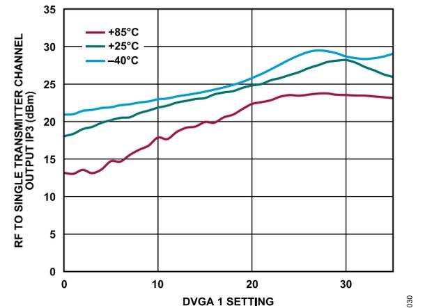
Figure 24. RF to Single Transmitter Channel Output IP3 vs. DVGA 1 Setting from 0 to 35 over Various Temperatures at 27 GHz
