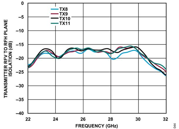
Figure 38. Transmitter RFV to RFH Plane Isolation vs. Frequency for Transmitter 8 (TX8), Transmitter 9 (TX9), Transmitter 10 (TX10), and Transmitter 11 (TX11)
