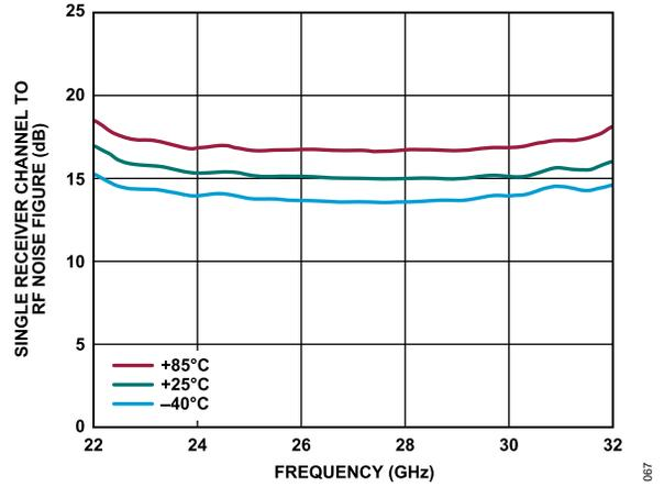
Figure 57. Single Receiver Channel to RF Noise Figure vs. Frequency at Various Temperatures at Maximum Gain
