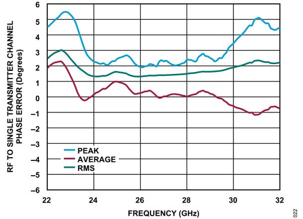
Figure 16. RF to Single Transmitter Channel Phase Error vs. Frequency for Peak, Average, and RMS Error
