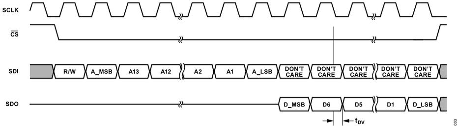
Figure 81. Timing Diagram for Standard SPI Register Read, 4-Wire Mode,
