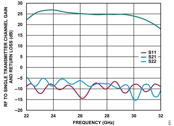
Figure 5. RF to Single Transmitter Channel Gain and Return Loss vs. Frequency at Maximum Gain
