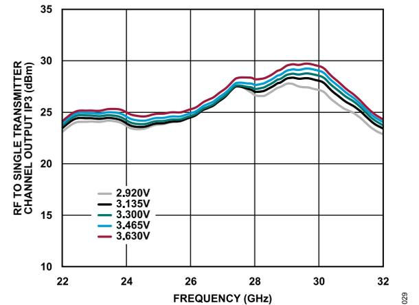
Figure 23. RF to Single Transmitter Channel Output IP3 vs. Frequency at Various Supply Voltages at Maximum Gain
