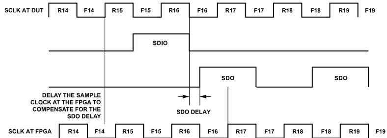
**Figure 85. Using a Delayed SCLK**
