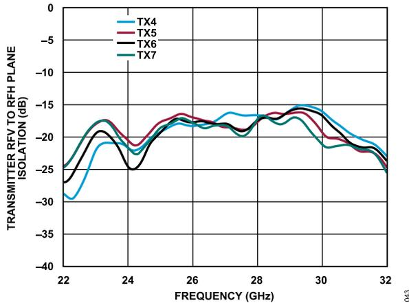
Figure 37. Transmitter RFV to RFH Plane Isolation vs. Frequency for Transmitter 2 (TX4), Transmitter 5 (TX5), Transmitter 6 (TX6), and Transmitter 7 (TX7)
