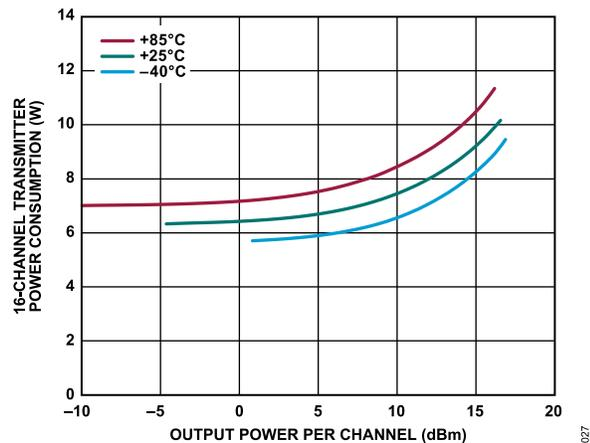
Figure 21. 16-Channel Transmitter Power Consumption vs. Output Power per Channel at Various Temperatures at Maximum Gain
