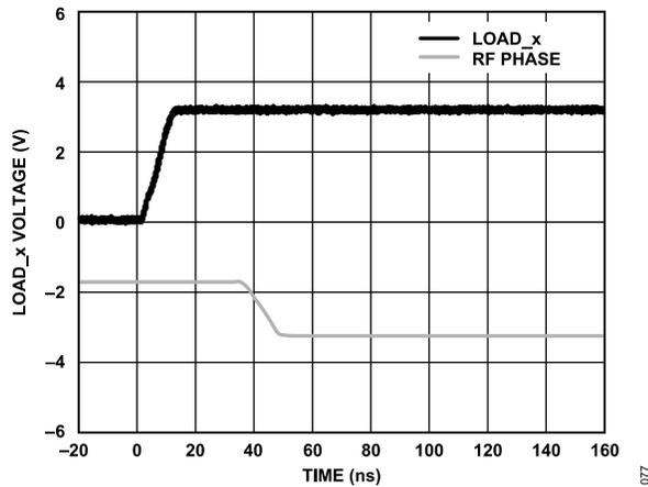
Figure 67. RF Phase Settling Time
