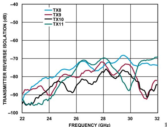
Figure 42. Transmitter Reverse Isolation vs. Frequency for TX8 to TX11
