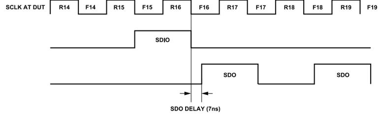
**Figure 83. SDO Delay Timing Diagram**
