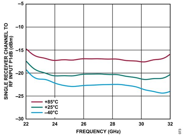
Figure 63. Single Receiver Channel to RF Input P1dB vs. Frequency at Various Temperatures at Maximum Gain
