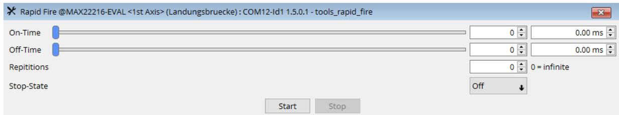
Figure 13: MAX22216 On/Off Slider Control for One Channel
