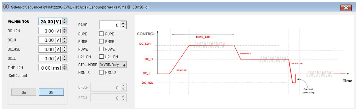
Figure 10: Sequencer Configuration of One MAX22216 Channel
