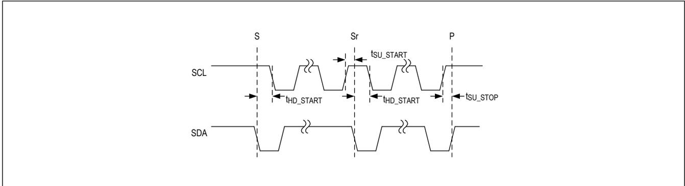
Figure 8. I<sup>2</sup>C Start Stop
