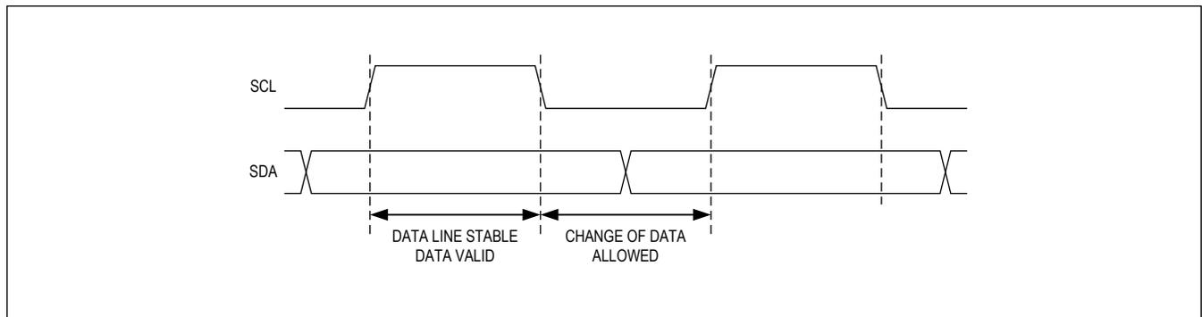
Figure 7. I<sup>2</sup>C Bit Transfer
