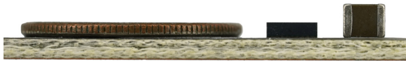
Figure 1. The small profile of the LTM4691 can be seen when placed next to a thin coin and a 1210 sized ceramic capacitor.
