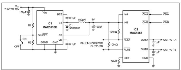
Figure 1. This automotive USB power supply generates two regulated, supply-voltage outputs from a single unregulated input.
