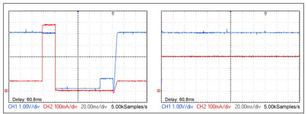
Figure 2. These current/voltage waveforms from Figure 1 show that an overload on output A (left graph) has no effect on output B (right graph). Fault indicator outputs FLTA and FLTB warn of overloads.
