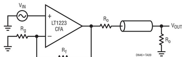
The cable driver circuit is the same for both types of amplifiers. But because most op amps do not have enough output drive current, they are not often used for heavy loads like cables. When driving a cable it is important to properly terminate both ends if even modest high frequency performance is required. The additional advantage of this is that it isolates the capacitive load of the cable from the amplifier so it can operate at maximum bandwidth
