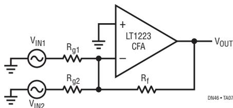
There is no  $I_{OS}$  spec on current feedback amplifiers because there is no correlation between the two input bias currents. Therefore, we will not improve the DC accuracy
