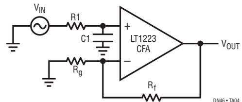
It is very common to limit the bandwidth of an op amp by putting a small capacitor in parallel with  $R_f$ . This works with all unity-gain-stable op amps; **DO NOT PUT A SMALL CAPACITOR FROM THE INVERTING INPUT OF A CURRENT FEEDBACK AMPLIFIER TO ANYWHERE, ESPECIALLY NOT TO THE OUTPUT.**
