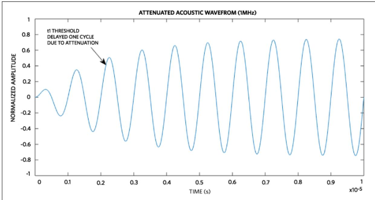
Figure 2. Attenuated transducer signal.
