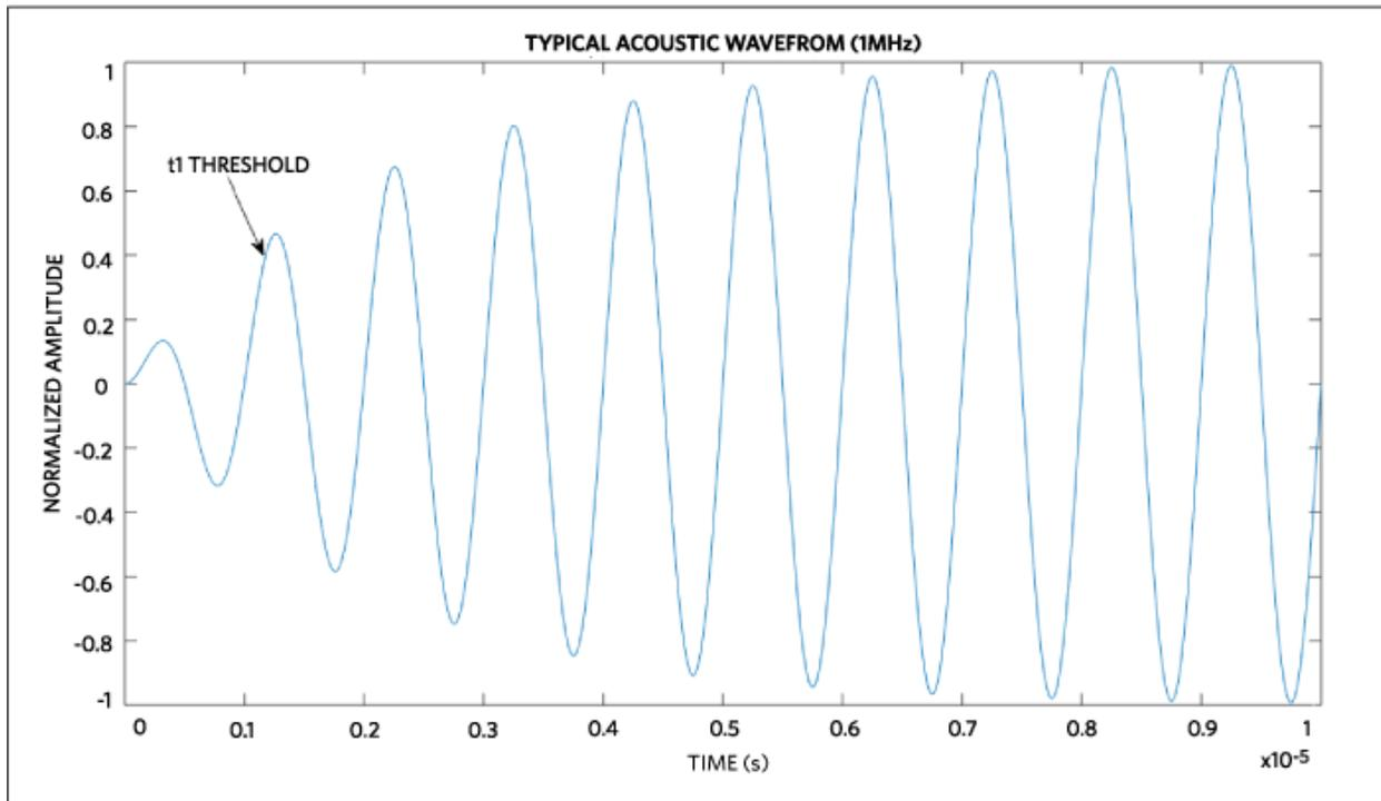
Figure 1. Normal transducer signal.
