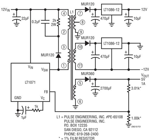
Figure 1. Multi-Output Flyback Converter
