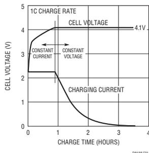
Figure 1. Typical Lithium-Ion Charge Characteristics
