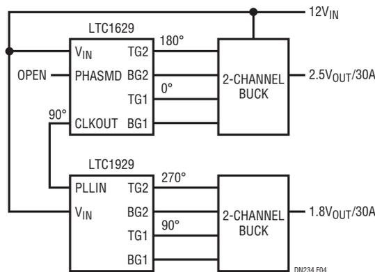
**Figure 4. Block Diagram of a 2-Output Power Supply**
