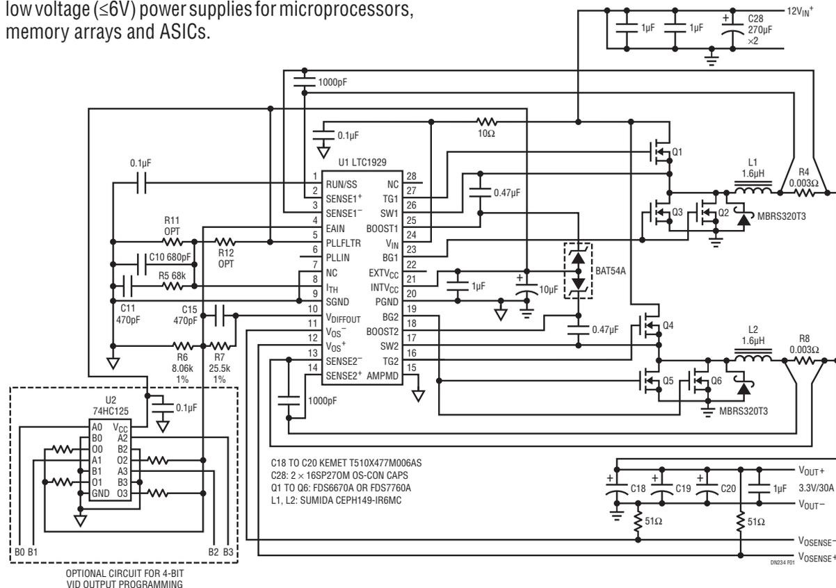
Figure 1. Schematic Diagram of a 30A Power Supply
