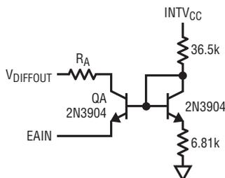
**Figure 3. Optional Circuit to Modify Foldback Current Limit**
