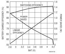
Figure 2. Switching PowerPath Battery Charger Efficiency and Power Savings Relative to a Linear Charger. ( $V_{BUS}$  = 5V, 5X MODE,  $R_{CLPROG}$  = 2.94k,  $R_{PROG}$  = 1k,  $I_{BAT}$  = 0.7A at  $V_{BAT}$  = 2.8V)
