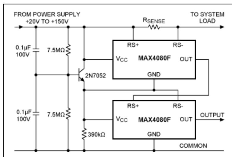
Figure 1. This circuit doubles the supply voltage at which current can be sensed.
