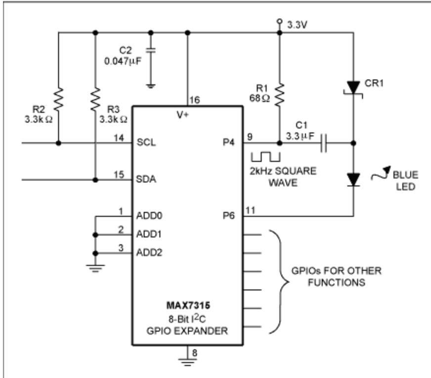
Figure 1. While performing other functions, this GPIO-expander chip can easily drive a blue LED as well.
