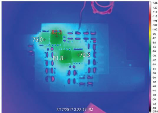
Figure 4. Thermal test at 48 V input, 24 V output at 20 A, and 200 kHz switching frequency.
