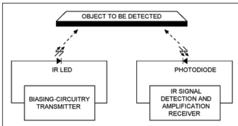
Figure 1. Basic principle of an IR proximity sensor.
