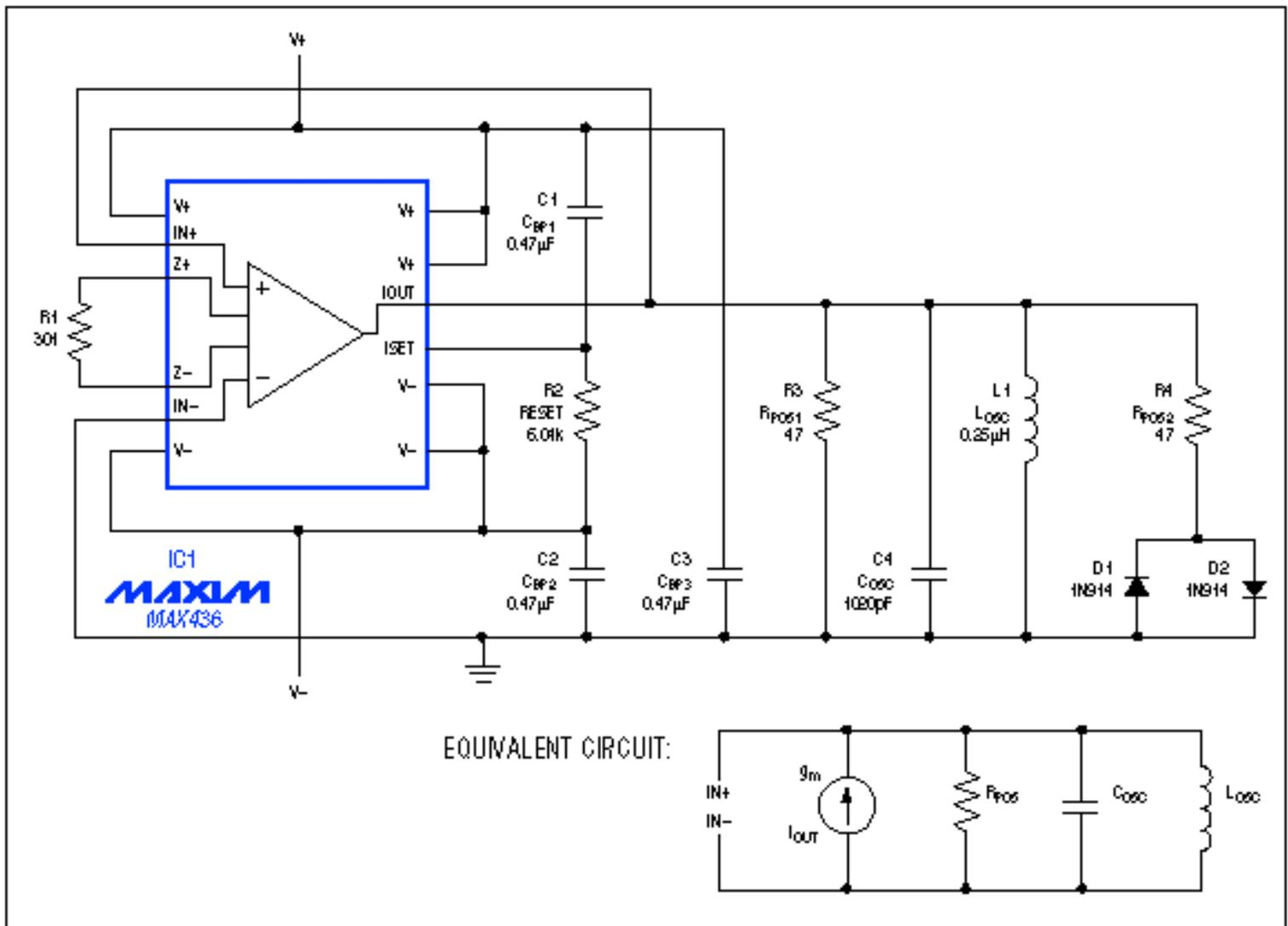
Figure 1. This 9.3MHz oscillator includes a wideband transconductance amplifier (IC1), whose negative resistance counters losses in the L1/C4 tank circuit.
