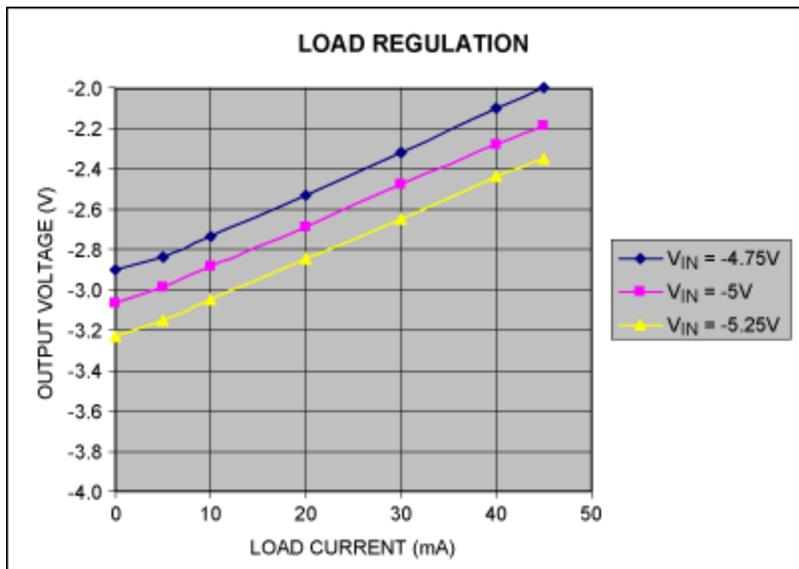
Figure 3. Load regulation for the Figure 1 circuit at  $V_{\text{IN}}$  levels of  $-4.75\text{V}$ ,  $-5\text{V}$ , and  $-5.25\text{V}$ .
