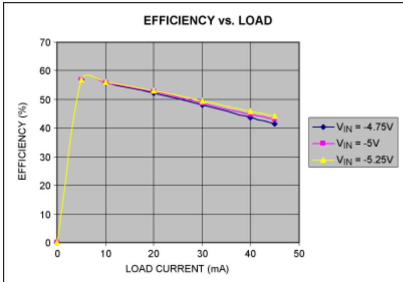
Figure 2. Efficiency vs. load for the Figure 1 circuit at  $V_{\text{IN}}$  levels of  $-4.75\text{V}$ ,  $-5\text{V}$ , and  $-5.25\text{V}$ .
