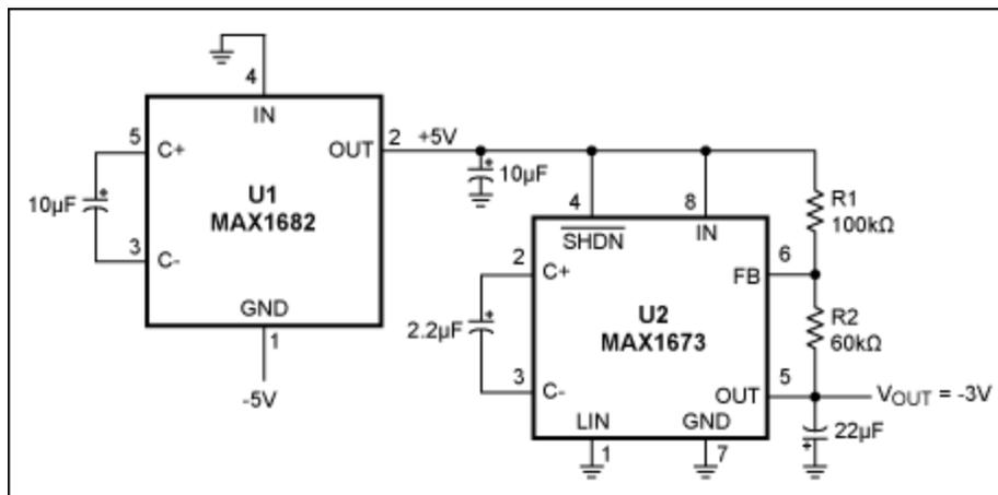
Figure 1. This negative stepdown converter (-5V to -3V) requires no inductor.
