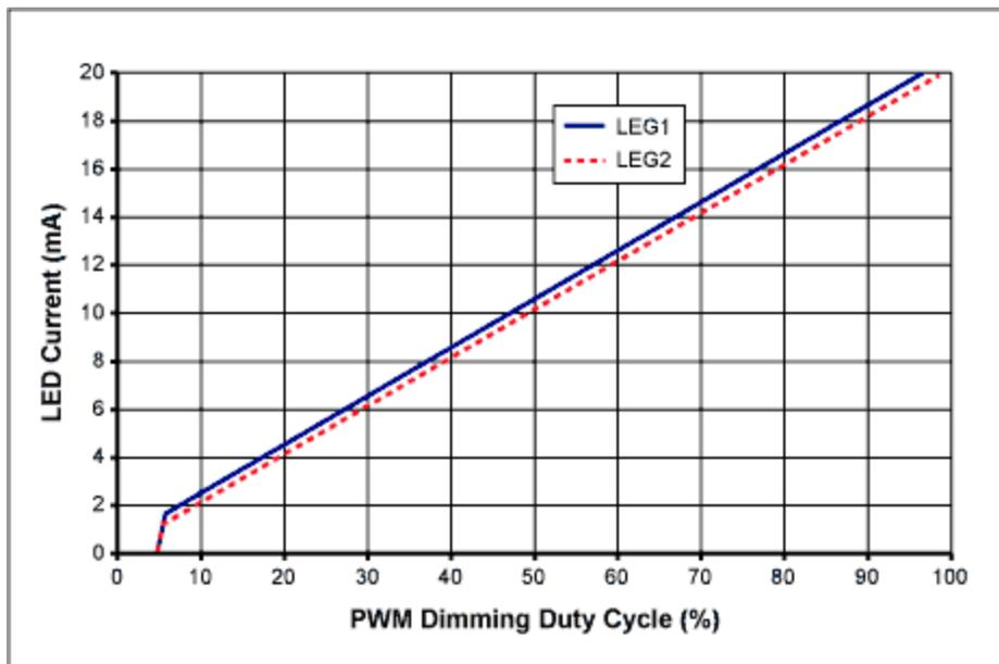
Figure 2. PWM dimming adjusts LED current and controls 1μA shutdown mode. Leg-to-leg current matching is good (better than 0.5mA).
