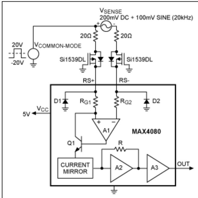
Figure 1. The two p-channel MOSFETs shown protect this high-side current-sense amplifier against negative common-mode voltages.
