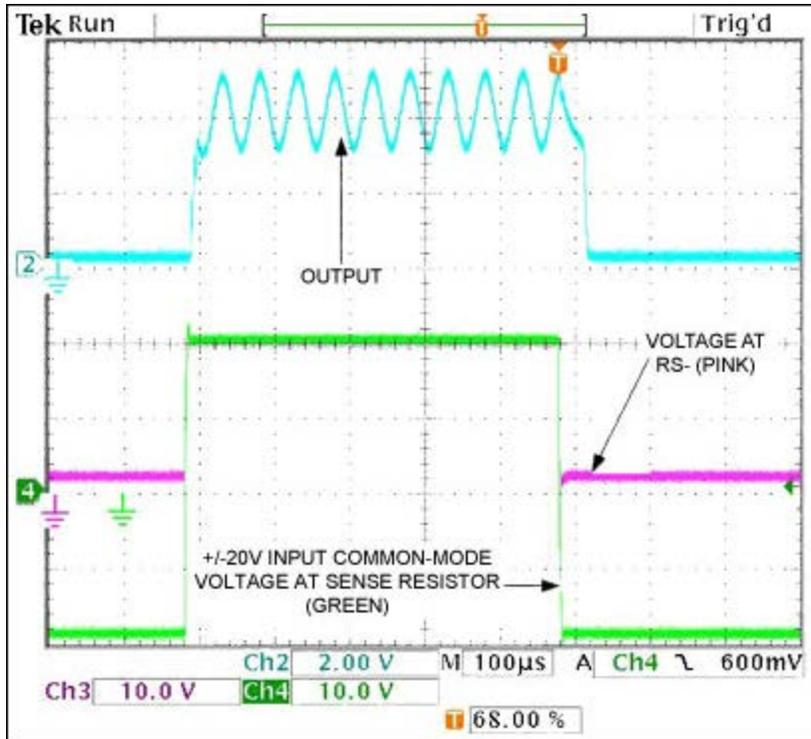
Figure 2. For the Figure 1 circuit with  $RS+/RS-$  inputs driven as described in the text, these waveforms show that the IC works normally for positive common-mode voltages up to 20V, and protects itself by shutting OFF ( $V_{RS-} = 0V$ ) during negative common-mode voltages down to -20V.
