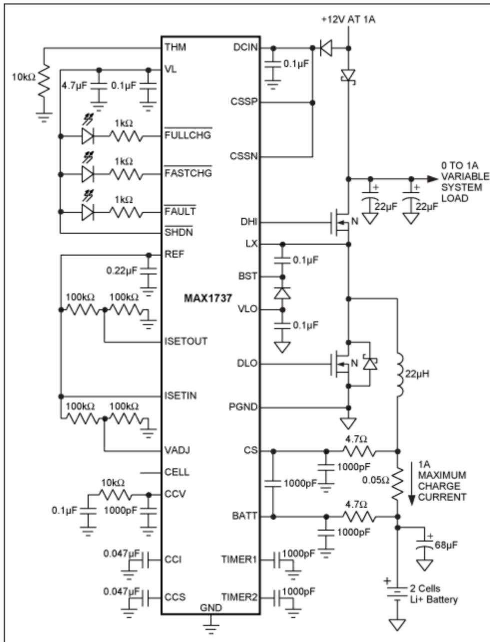
Figure 2. Disabling the source-current loop of the MAX1737 reduces cost and size by eliminating seven components. With the source-current loop disabled, the power source must be able to supply the maximum battery charging current and the maximum system load current.
