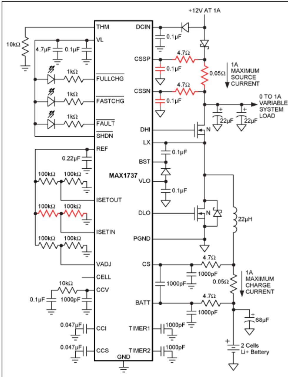
Figure 1. To limit the power drawn from the source, the standard implementation of the MAX1737 decreases the battery charge current as the system load increases.
