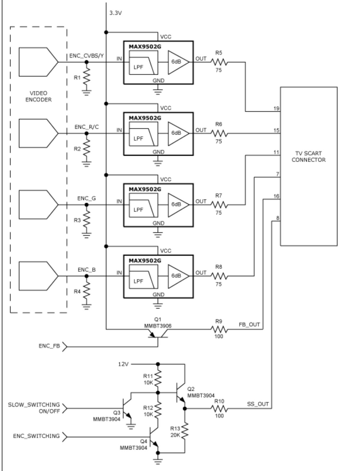
Figure 1. Simple, low-cost circuit for a single TV SCART video driver.
