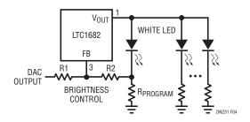
Figure 4. Brightness Control Using DAC Output
