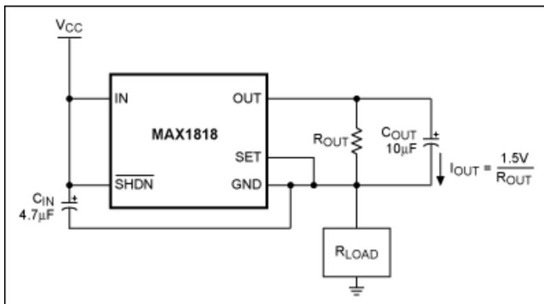
*Figure 1. This high-side constant-current source features the MAX1818 LDO and draws  $1.5V/R_{OUT}$  from  $R_{LOAD}$ . The circuit requires the voltage for  $R_{OUT}$  between the IN and GND terminals to be minimally 2.5V.*
