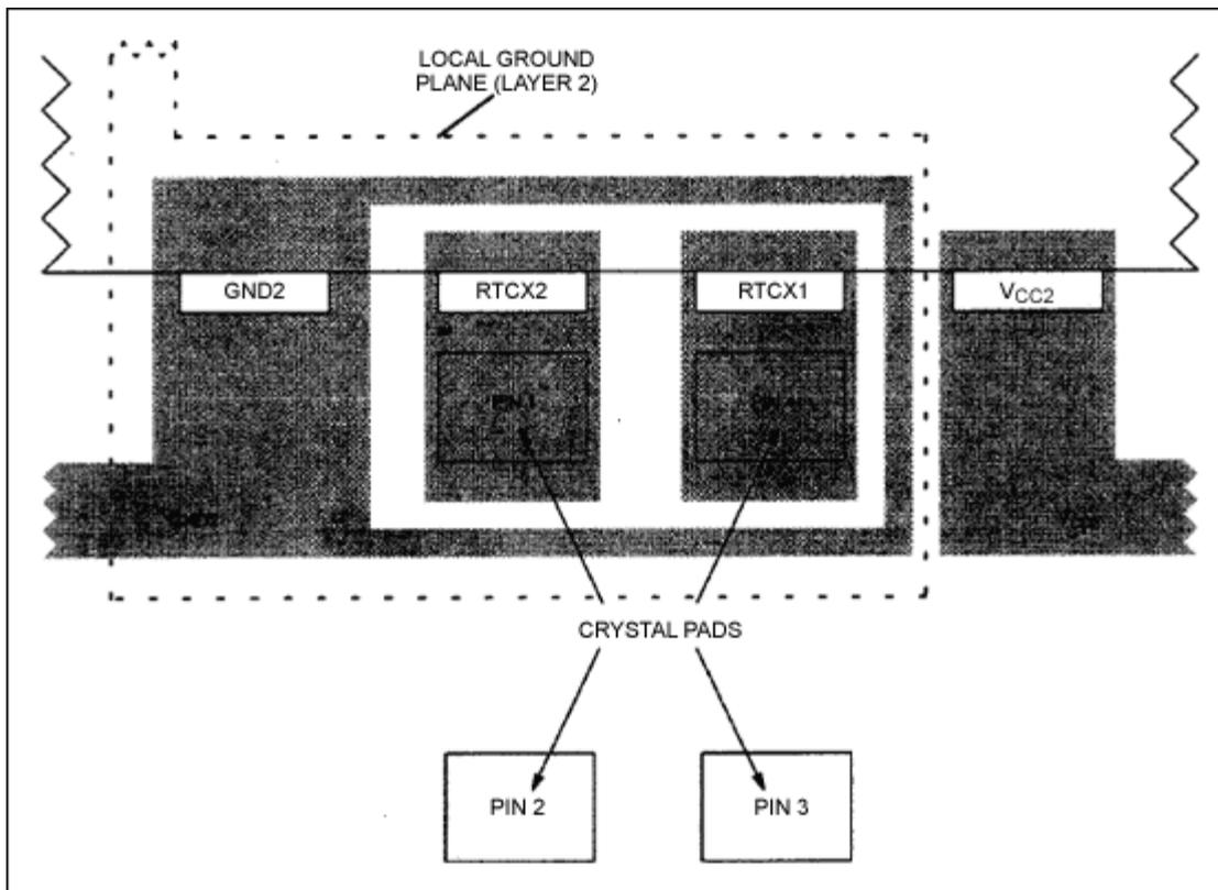
Figure 2. Example crystal placement on PC board.
