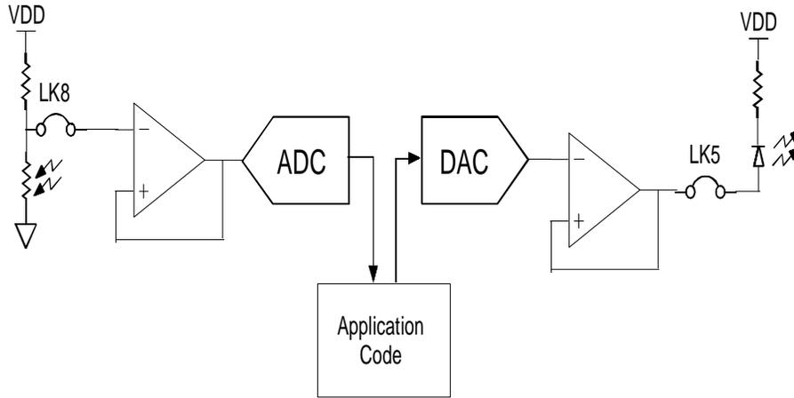
*Figure 2: Circuit diagram of the LDR Circuit*
