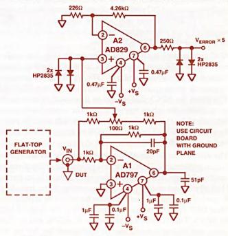
A1, the DUT in this circuit, is configured for a gain of -1. The voltage divider from input to output forms a second "false" summing node that will replicate the signal at the amplifier's summing node. The  $100-\Omega$  potentiometer is used to null the dc voltage. The wiper of the potentiometer is clamped by the diodes at the input of A2 to limit saturation effects in this amplifier. The output is also similarly clamped.
