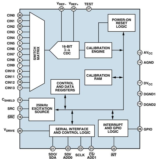
Figure 3. AD7142 block diagram.
