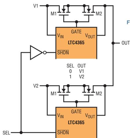
Figure 7. Selecting between one of two supplies
