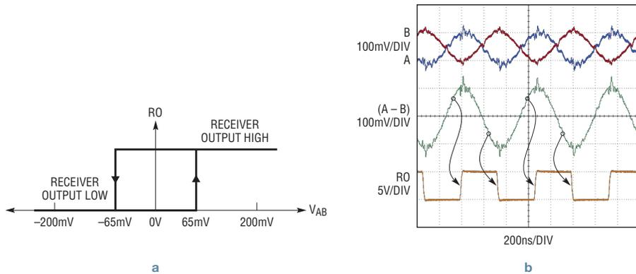
**Figure 12. (a) RS485 receiver input threshold characteristics for fast moving signals. (b) Measured 3Mbps signal driven down 4000ft of CAT5e cable. Top Traces: receiver signals after transmission through cable; Middle Trace: math showing the differences of the top two signals; Bottom Trace: receiver output, exhibiting excellent duty cycle.**
