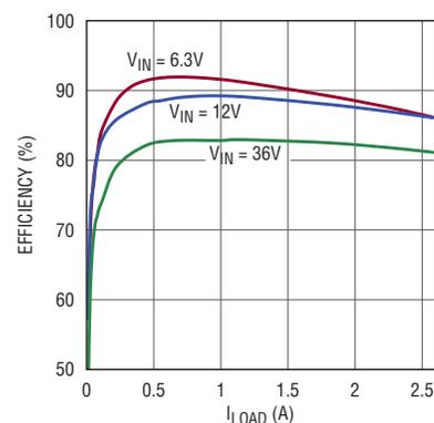
Figure 3. Switching regulator efficiency
