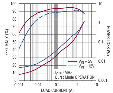
Figure 4. Burst Mode operation yields high efficiency at light loads, and low R<sub>DS(ON)</sub> switches maintain high efficiency at maximum load.
