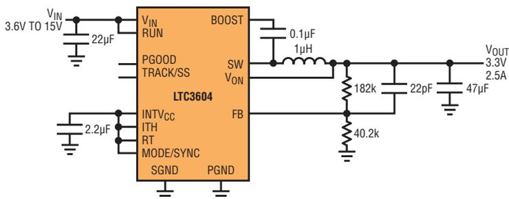
The LTC3601 and LTC3604 employ a unique constant frequency/controlled on time architecture with a minimum on-time of 20ns—ideal for high step-down ratio applications that demand high switching frequencies and fast transient response.
