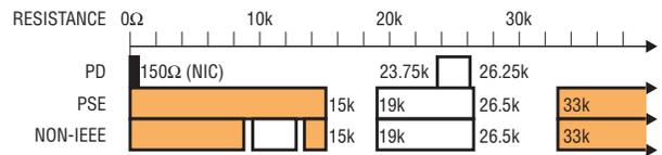
solutions, Linear's LTPoE++ provides mutual identification between the PSE and PD. LTPoE++ PSEs can differentiate between an LTPoE++ PD and all other types of IEEE compliant PDs, allowing LTPoE++ PSEs to remain compliant and interoperable with existing equipment.
