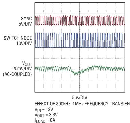
Figure 3. The synchronized switching frequency can be shifted on the fly, with little change in V<sub>OUT</sub>.
