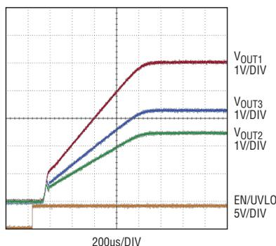
Figure 2. Ratiometric tracking waveforms
