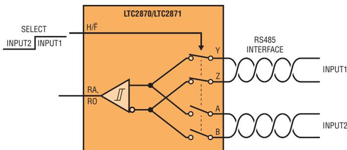
without disturbing the bus. Optionally, the bus may be driven during loopback by simply enabling the appropriate driver. Figure 14 shows loopback operation.
