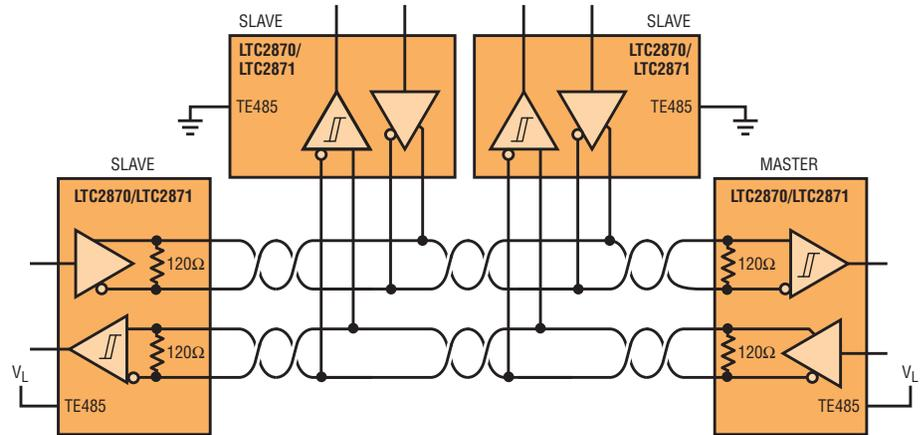
twice the one-way propagation delay in the cable. This small deviation from ideal is easily tolerated in most communications systems, and can improve performance, which is why the PROFIBUS standard specifies a similar termination mismatch.
