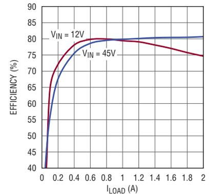
Figure 5. Efficiency of the converter in Figure 4
