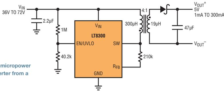
Figure 3. A 5V/300mA micropower isolated flyback converter from a 36V-to-72V input
