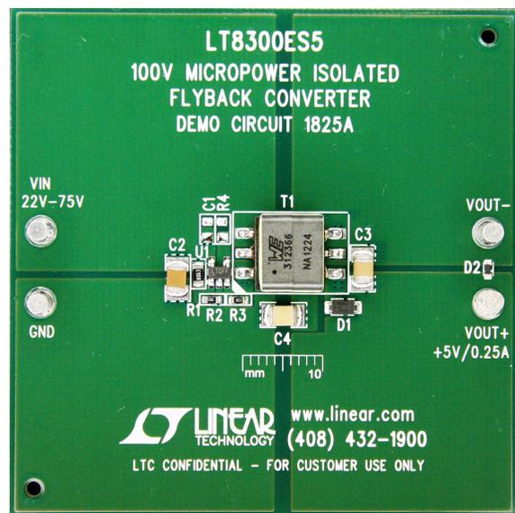
Figure 2. The LT8300 isolated flyback converter solution size is less than 1 inch by 1/2 inch in a standard demo board DC1825A.
