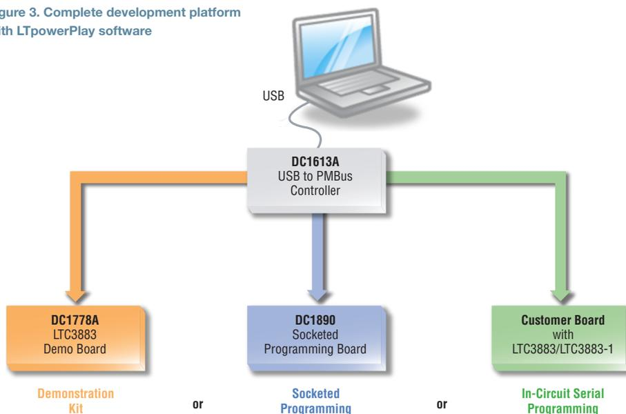
Digital power system management makes it possible to quickly and efficiently develop complex multirail systems. Design is further simplified by LTpowerPlay software, which enables PC-based board monitoring and parametric adjustments.
