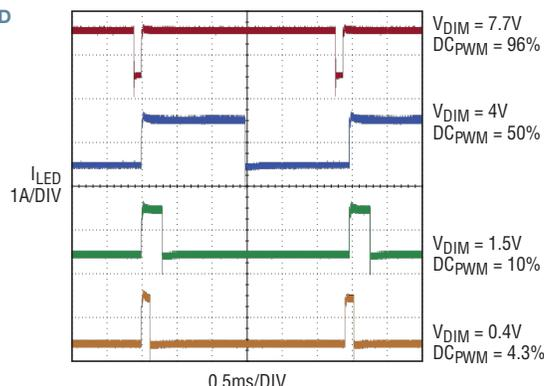
LT3761 requires only an external DC voltage, much like analog dimming control, for high performance PWM dimming at a chosen frequency. It can still receive a PWM input signal to drive the LED string with that signal in standard fashion.
