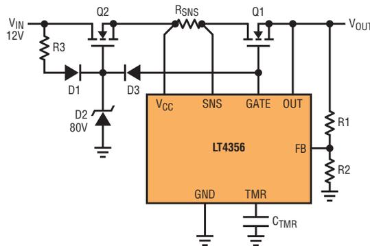
MOSFETs to replace a single, and much more costly, special high SOA device. As the peak input voltage requirement rises above 200V, the SOA becomes increasingly concentrated in Q2 and the series connection offers no substantial relief.
