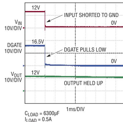
b. In reverse input conditions, the DGATE pins pulls to the SOURCE pin, keeping the ideal diode MOSFET off and cutting off back feeding.
