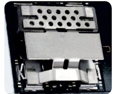
Figure 2. LTM4620 side view rendering and photo of an unmolded LTM4620 showing topside heat sink
