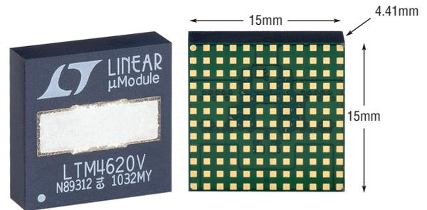
**Figure 1.** The LTM4620 LGA package includes thermal contacts on the top and bottom that connect to a unique internal heat sink, which keeps internal components cool by minimizing the internal thermal resistance.
