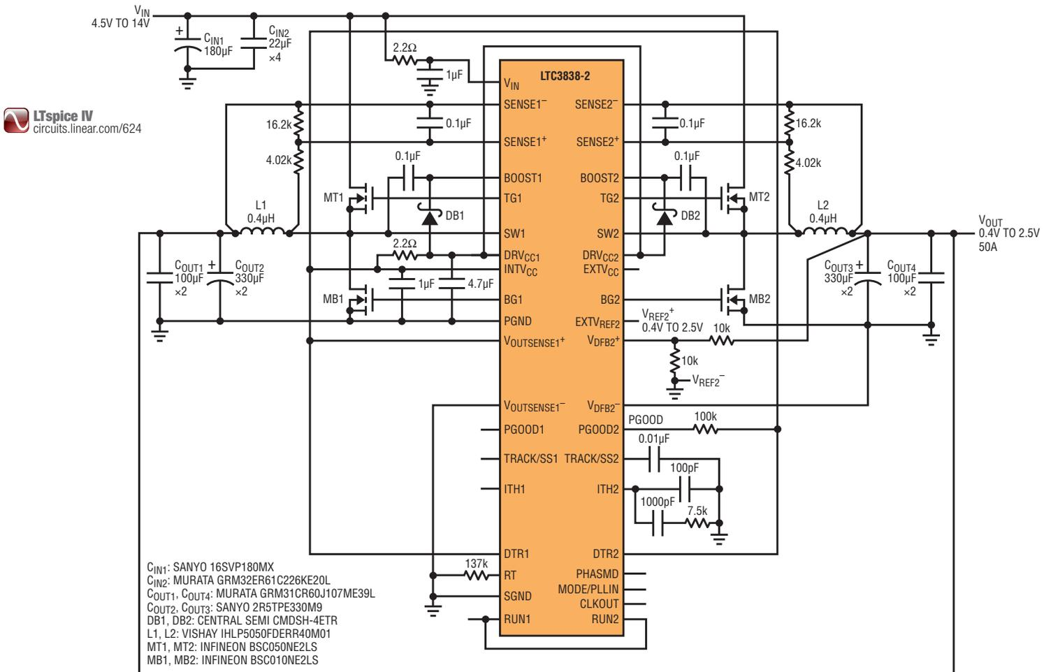
In addition to regulation accuracy, the LTC3838-2 offers wide-bandwidth tracking to a dynamic external reference. Tracking bandwidth is important in applications like dynamic voltage scaling because bandwidth determines how quickly the supply can respond to changes to the programmed external reference.
