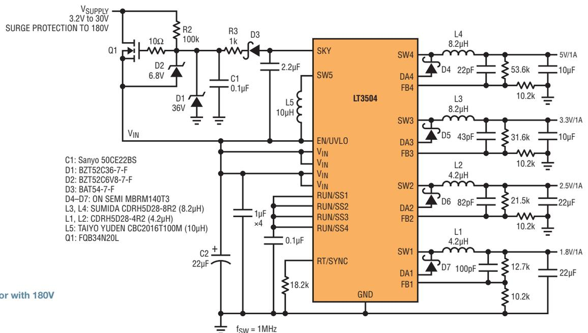
Figure 1. Complete quad buck regulator with 180V surge protection
