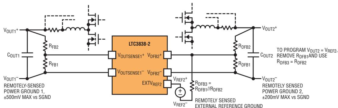
For differential external reference sensing, the LTC3838-2 has only one pin for external reference input. Channel 2 features a unique feedback amplifier configuration, which eliminates the need for a separate pin to sense the external reference's remote ground. Instead, one additional resistor, equal to the parallel of the two feedback resistors, is used to connect to the remote ground externally.
