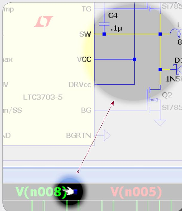
Alt + left-click on a label, V(n008), in the waveform viewer to highlight that particular net in the schematic editor.
