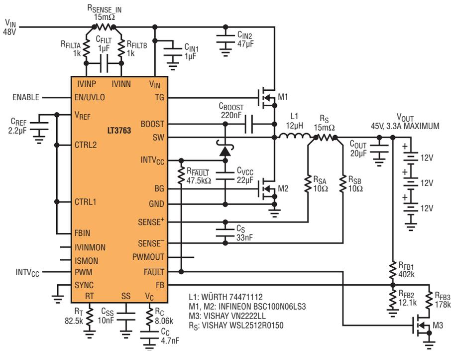
Figure 4. 3.3A, six-cell (36V) SLA battery charger
