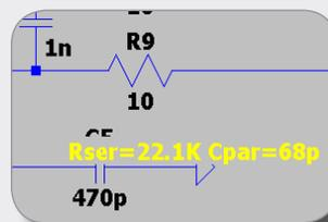
Ctrl + Alt + Shift + H temporarily highlights all hidden text within the schematic. In this example, a series resistor and parallel capacitor are encapsulated and hidden within C5 to simplify layout.
