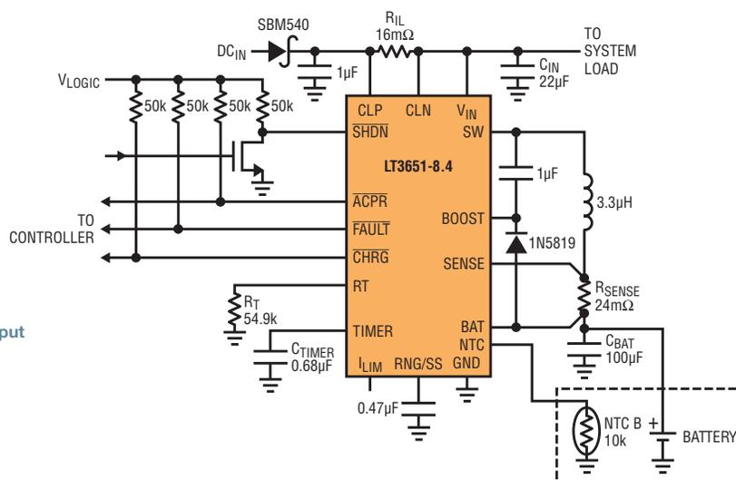
Figure 2. 2-cell Li-ion 9V to 32V charger with input current limit and 3-hour charge timeout
