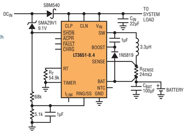
The LT3651 is a versatile, compact and easy-to-use solution for charging Li-ion batteries with up to 4A in current and from input supplies up to 32V (40V ride through). High efficiency, built in safety controls and compact size make it an easy fit in a wide variety of applications.
