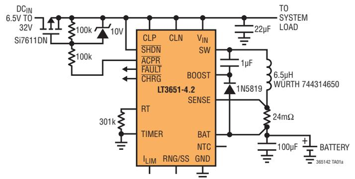
Charger safety is a significant concern as batteries increase in capacity and usage. The LT3651 includes all of the necessary charge termination and protection features. Charge termination methods include C/10 termination or safety timer termination.
