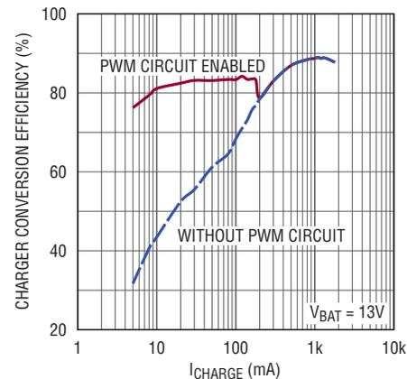
Figure 7. Efficiency curve for circuit in Figure 6
