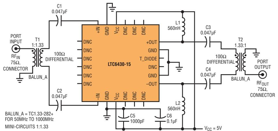
Figure 16. 50MHz to 1000MHz CATV push-pull amplifier with 75Ω input and 75Ω output
