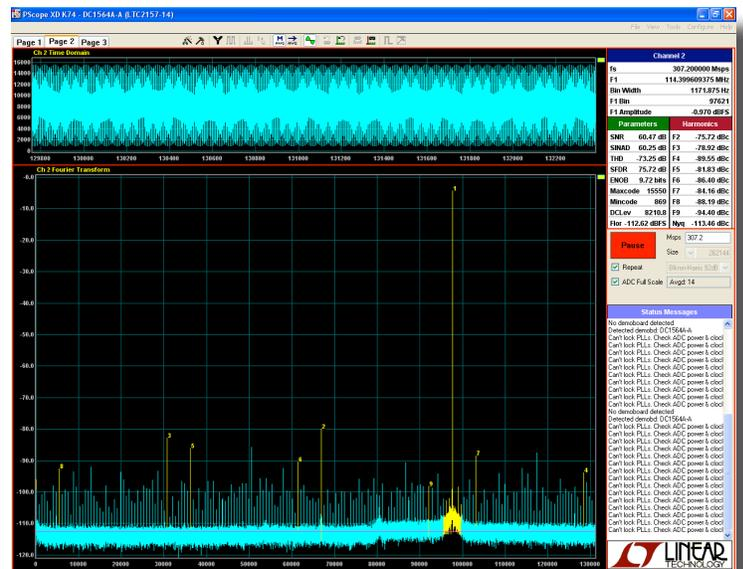
**Figure 11. 500MHz 2-tone measurement of IM3 products of LTC6430-15 and LTC2158 driver/ADC combo board (IM3 low = -101dBfs, IM3 high = -102dBfs)**
