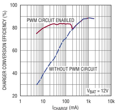
Figure 4. Efficiency for the circuit in Figure 2
