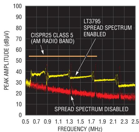
Figure 2. Conducted peak EMI around the AM band is reduced by 3dB $\mu$ V–6dB $\mu$ V when the LT3795's spread spectrum frequency modulation is used. The CISPR25 Class 5 AM-band limit is provided for reference.
