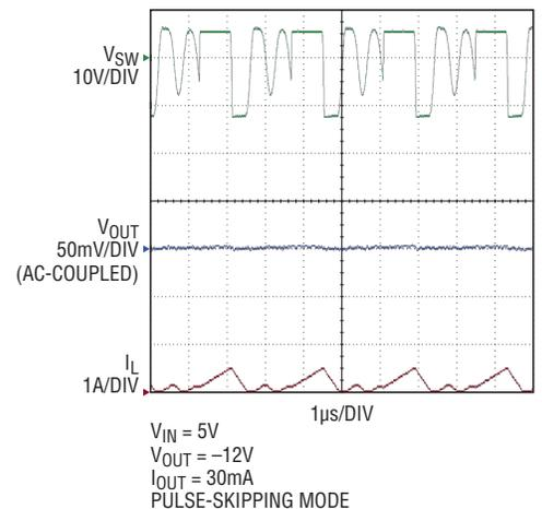
The LTC3863 can produce a  $-0.4\text{V}$  to  $-150\text{V}$  negative output voltage from a positive input range of  $3.5\text{V}$  to  $60\text{V}$ . It uses a single-inductor topology with one active P-channel MOSFET switch and one diode. The high level of integration yields a simple, low parts count solution.
