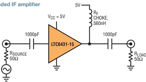
Noise (characterized by NF) limits an amplifier's sensitivity at low input signal amplitudes, while linearity (characterized by OIP<sub>3</sub>) limits sensitivity at high input amplitudes. Taken together, these two metrics, NF and OIP<sub>3</sub>, define the amplifier's useful dynamic range for a signal.
