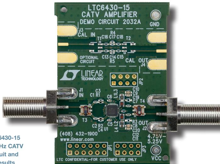
Figure 17. LTC6430-15 50MHz-1000MHz CATV evaluation circuit and performance results
