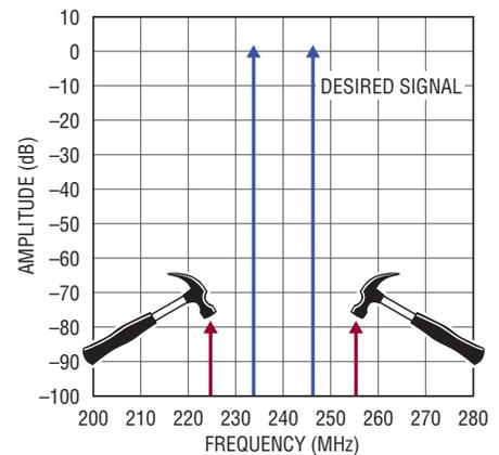
Figure 4. The LTC6431-15 boasts an OIP3 of 47dBm at 240MHz—essentially hammering the IM3 products of a 2-tone signal into the noise floor so that they don't interfere with the intended signals.
