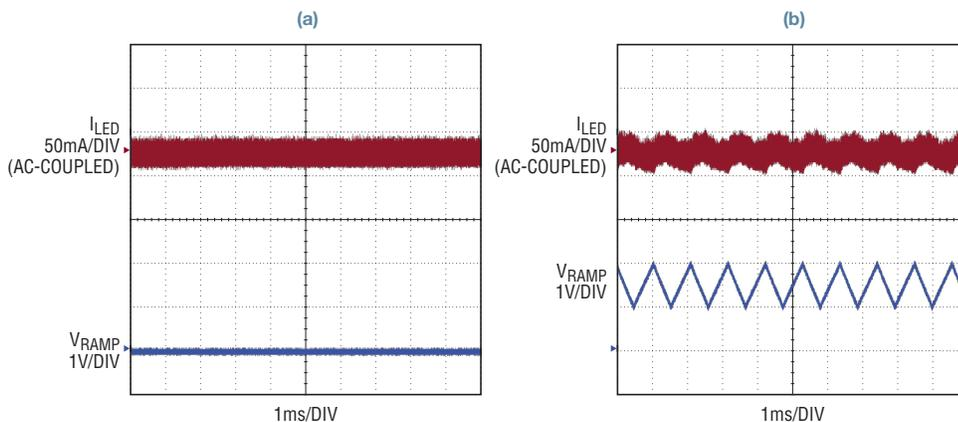
The 6.8nF capacitor at the RAMP pin sets the spread spectrum frequency modulation rate to a 1kHz triangle—that is, the LT3795’s operating frequency sweeps from 300kHz to 450kHz and back every millisecond. The addition of the triangular 1kHz spread spectrum signal has a negligible effect on LED ripple current, as shown in Figure 4.
