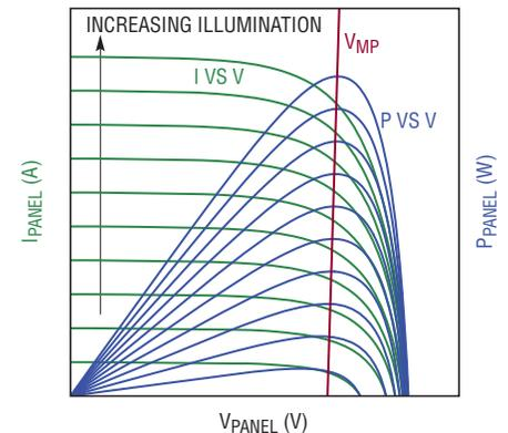
Figure 1. A solar panel produces maximum power at a particular output voltage,  $V_{MP}$ , which is relatively independent of illumination level. The LT3652 2A battery charger maximizes the output power of a solar panel by regulating the input panel voltage at  $V_{MP}$ .
