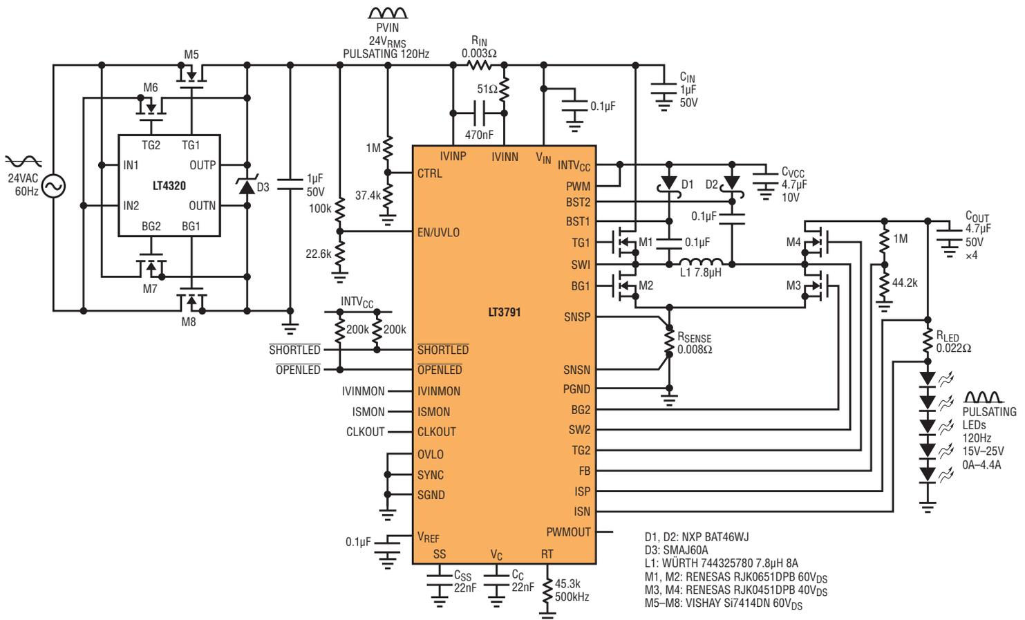
Figure 1. 24V AC to 60W LED driver (600W halogen equivalent) features high power factor and high efficiency
