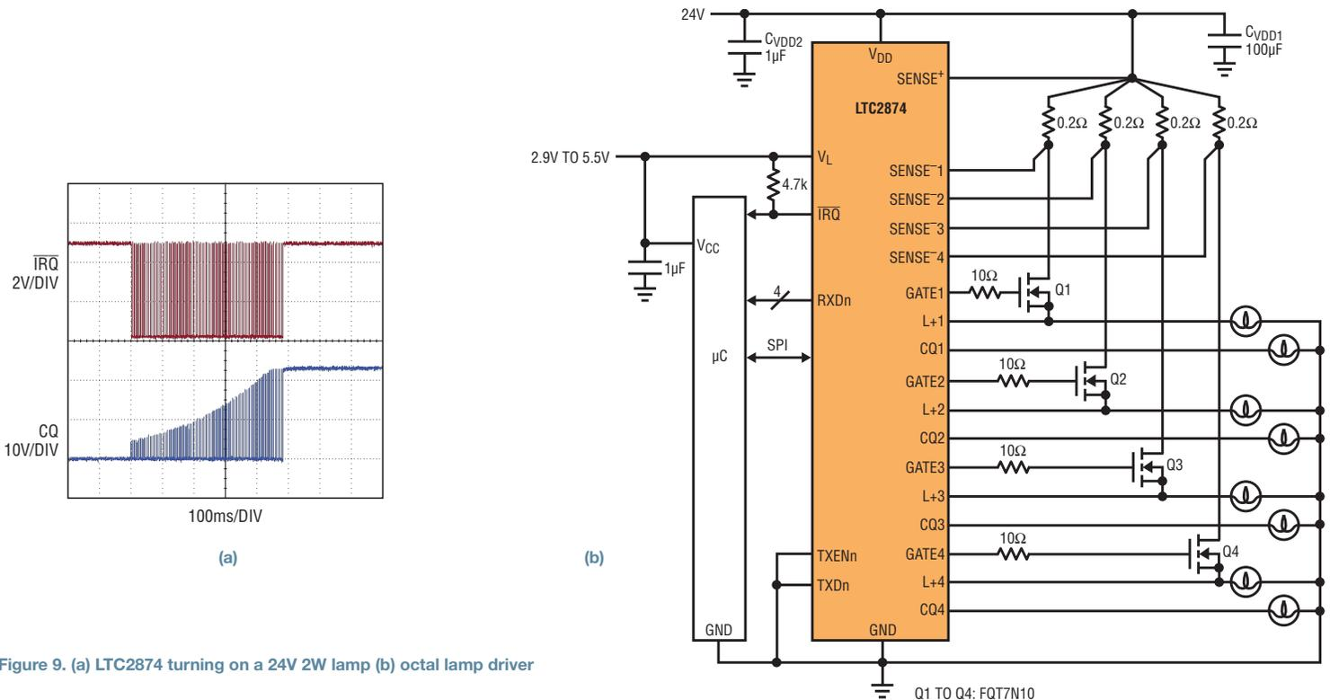
Figure 9. (a) LTC2874 turning on a 24V 2W lamp (b) octal lamp driver
