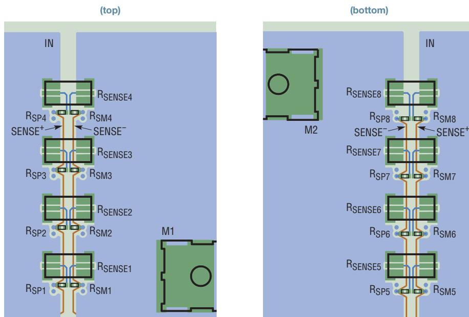
Modern servers utilize load currents that bring new challenges to Hot Swap design. Two areas of concern are MOSFET safe operating area, and the Kelvin sensing techniques for multiple sense resistors. The 12V/100A LTC4218 Hot Swap controller solution shown here specifically addresses these design points.
