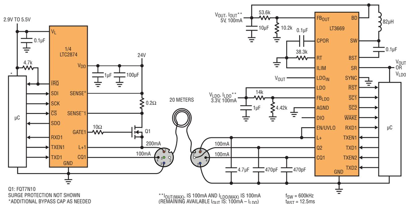
Figure 18. Complete 24V 3-wire power and signaling interface to sensor or actuator. One of four available master ports is shown.
