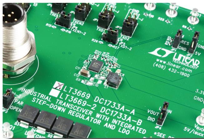
Sensors offer a wide breadth of physical measurement capabilities, and with that just as many varied power requirements. It is impossible to meet this range of requirements with just a switching regulator or LDO. Both are built into the LT3669 and LT3669-2, allowing these devices to meet most power requirements without additional converters.
