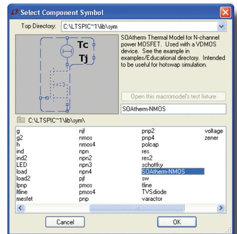
Easily model the thermal behavior of MOSFETs in LTspice using the SOAtherm NMOS symbol.
