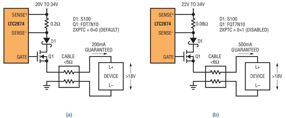
Figure 4. (a) LTC2874 configured for IO-Link-compliant 200mA device supply. Optional D1 provides supply isolation. (b) Alternative configuration for 500mA.
