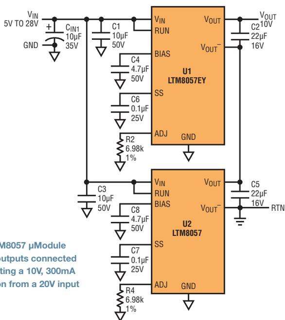
Figure 2. Two LTM8057  $\mu$ Module regulators with outputs connected in series, supporting a 10V, 300mA output application from a 20V input
