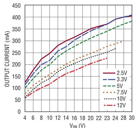
Figure 1. Typical maximum output current vs input voltage
