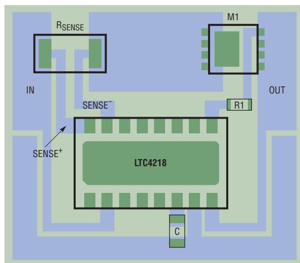
Figure 2. Kelvin sensing with single sense resistor
