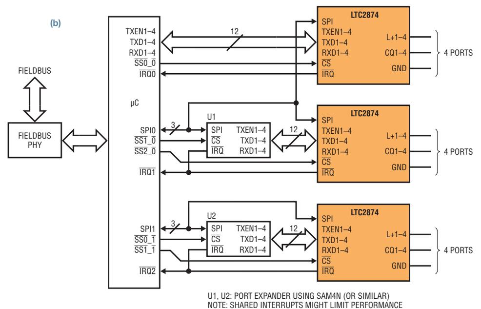
The dense integration of a quad IO-Link master PHY into QFN and TSSOP packages makes the LTC2874 ideal for building larger multiport masters.
