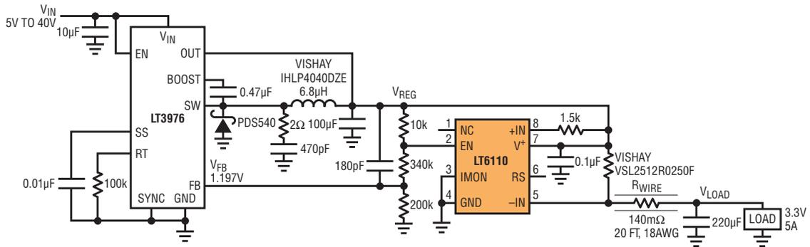
Figure 2. Example of a high current remote load regulation: a 3.3V, 5A buck regulator with LT6110 cable/wire voltage drop compensation
