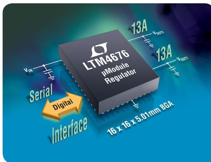
Linear was recognized by *EE Times China* in September with the Product of the Year Award in the Power Management category for the LTM4676, a dual 13A or single 26A  $\mu$ Module step-down DC/DC regulator with a serial digital interface.
