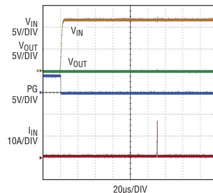
Figure 5. Start-up into a short circuit
