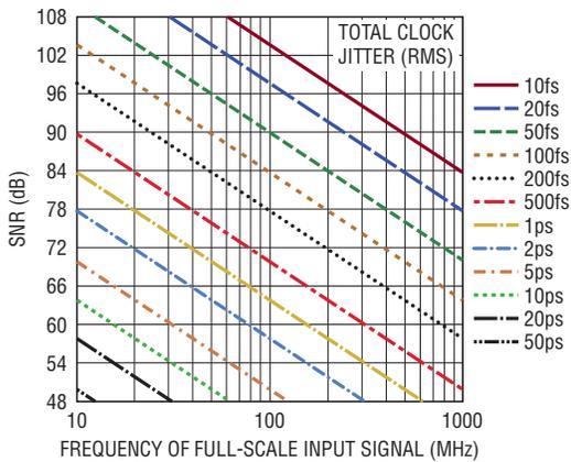
Figure 7. Graphical representation of Equation 3
