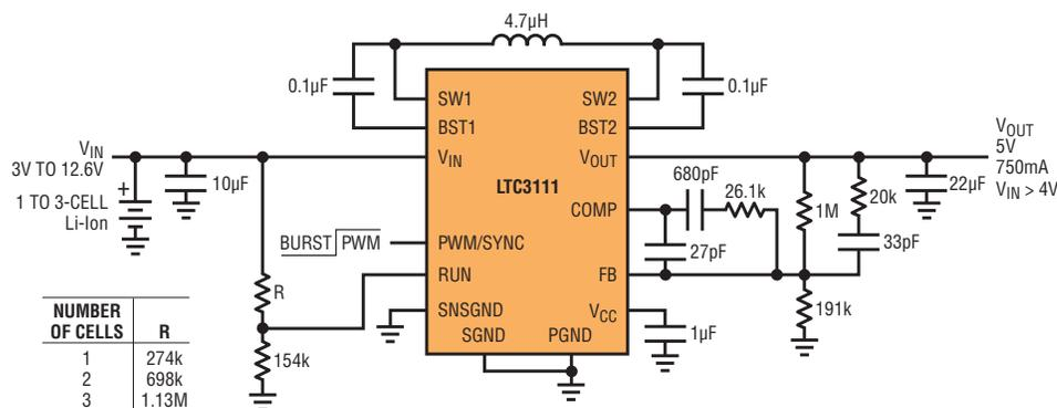
In addition to its wide operating range, the LTC3111 features Linear Technology's proprietary low noise buck-boost PWM control architecture, effectively eliminating jitter and EMI that can occur when crossing the boundary between step-up and step-down operation. This reduces or eliminates the need for expensive filtering or shielding for noise sensitive data conversion or RF circuitry in the system.
