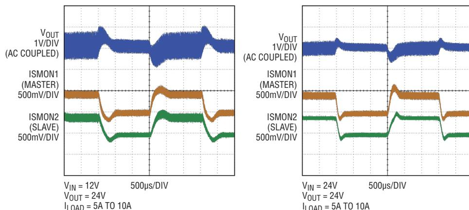
Figure 5. Parallel converter transient response evenly shares current
