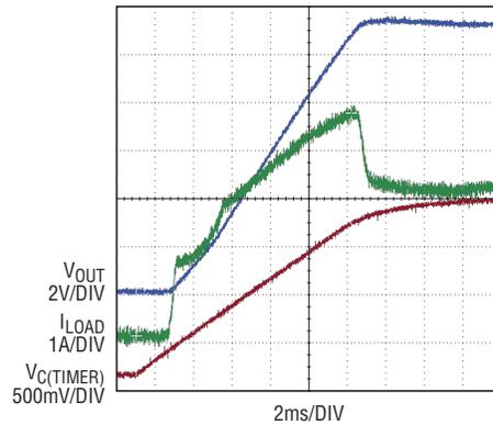
**Figure 6. R-C load with limited  $S_O$ .** Operating point leaves current limit mode in the first area, where current limit is  $I_{INIT}$ .
