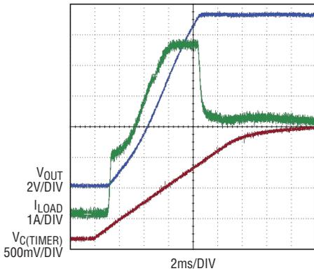
**Figure 5. R-C load without limitation for  $S_O$ .** Operating point leaves current limit mode in the third area, where current limit is  $I_{LIMIT}$ .
