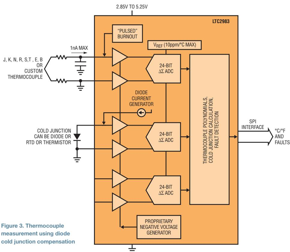
Figure 3. Thermocouple measurement using diode cold junction compensation
