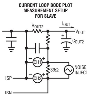
perturbation signal and measuring the loop response, as shown in Figure 6.
