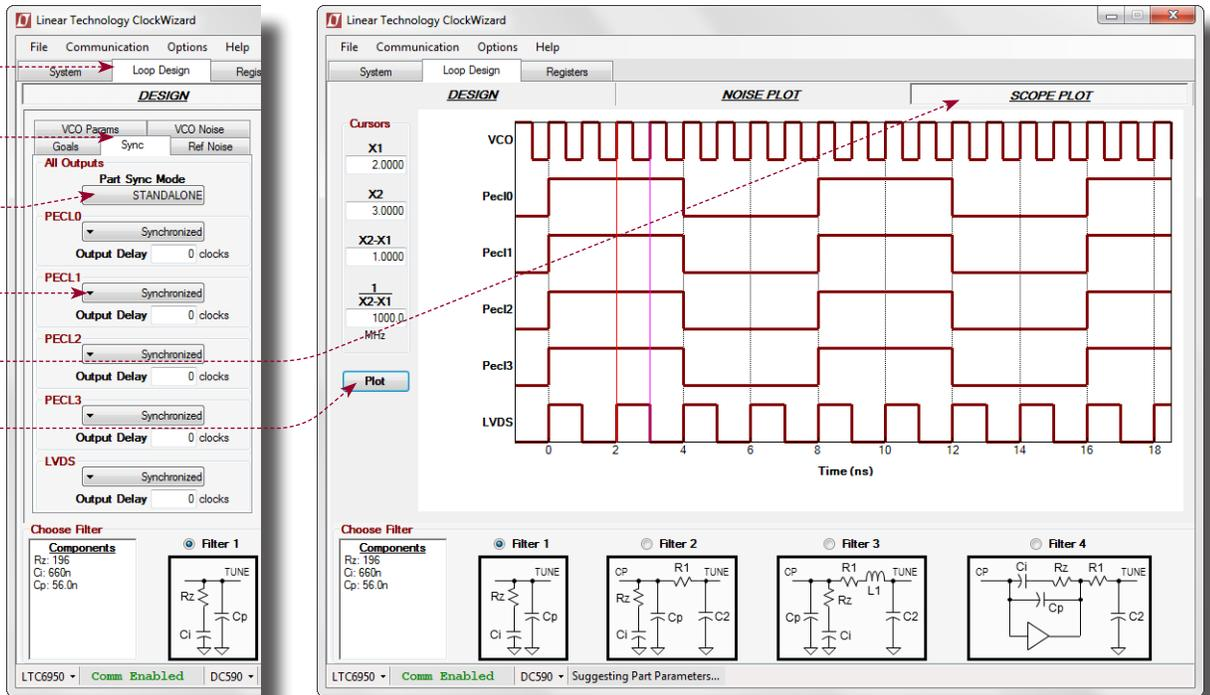
Figure 5. Simulating the LTC6950's output frequencies and output delays in STANDALONE mode using ClockWizard
