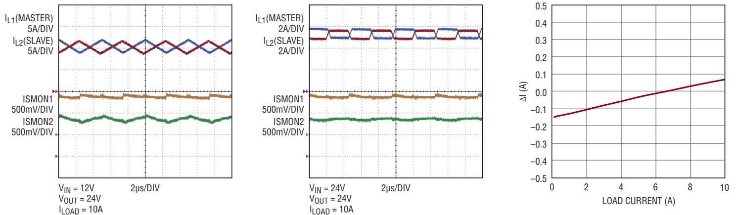
Figure 4. Parallel converter inductor and output current matching
