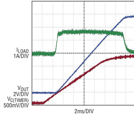
Figure 3. (Case 2) Pure capacitive load with a limited  $S_O$  (natural output voltage slew rate). Operating point leaves current limit mode in the first area, where current limit is  $I_{INIT}$ .
