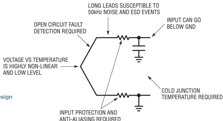
Figure 2. Thermocouple design challenges
