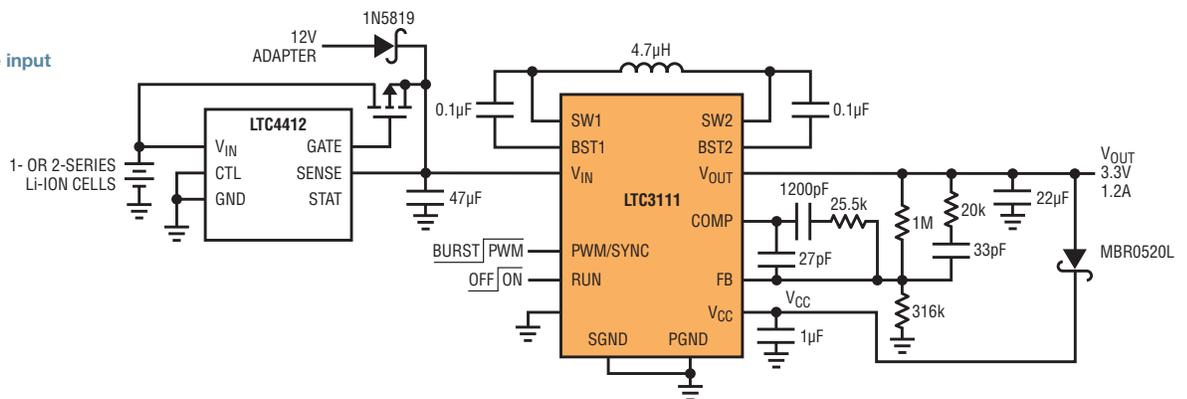
The LTC3111 includes circuitry to minimize loop gain variation, resulting in improved line transient response. Regulation for  $V_{OUT} = 3.3V$  remains within 50mV, or 1.5%, during a 20 $\mu$ s, 7.2V-to-12V,  $V_{IN}$  rise and fall transition with a 22 $\mu$ F output capacitor and 1A load.
