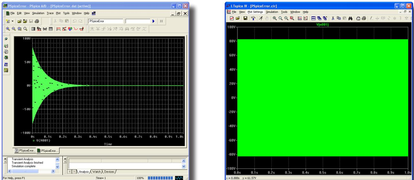
Figure 3. PSpice (left), utilizing modified Gear numerical integration, incorrectly artificially dampens ringing in the circuit of Figure 2. LTspice (right) produces the correct result.
