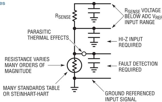
the temperature of the sensor solving Steinhart-Hart equations or table data.
