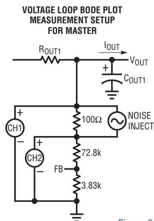
Figure 6. Loop response measurement of parallel converters
