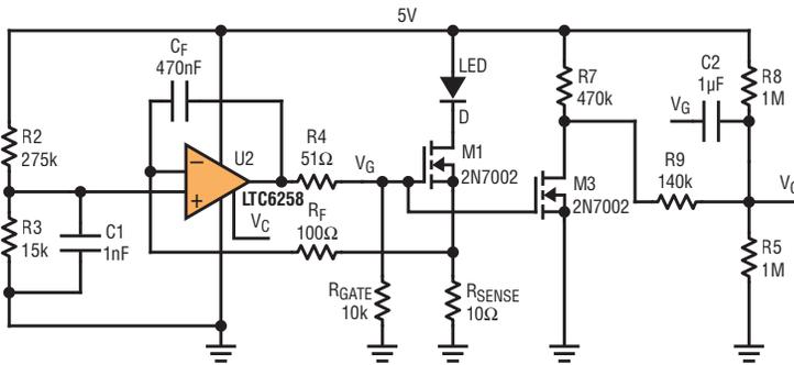
Figure 9. LED driver with self-oscillation
