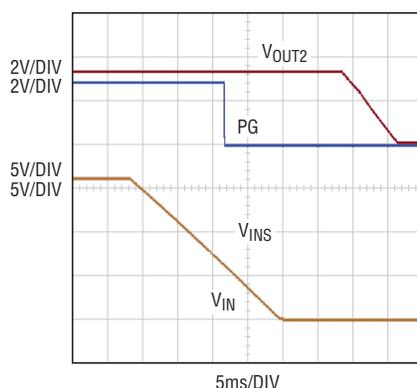
Figure 2. When the input voltage  $V_{IN}$  drops, the converter U1 boosts  $V_{OUT1}$  to maintain  $V_{INS}$  at 8V.  $V_{INS}$  provides power to keep  $V_{OUT2}$  in regulation for over 20ms after  $V_{IN}$  drops out.
