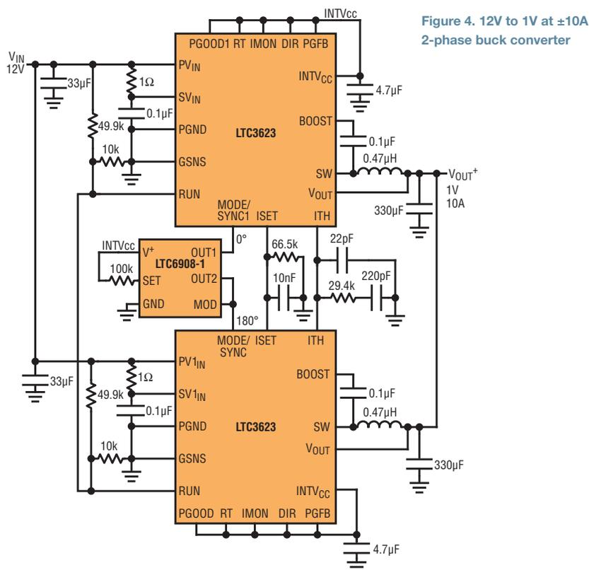
Figure 4. 12V to 1V at  $\pm 10A$
