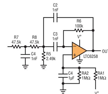
Figure 4. 10kHz bandpass filter
