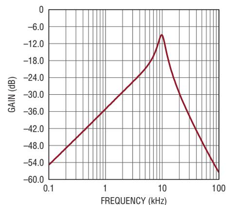
Figure 5. Bandpass filter gain/phase vs frequency
