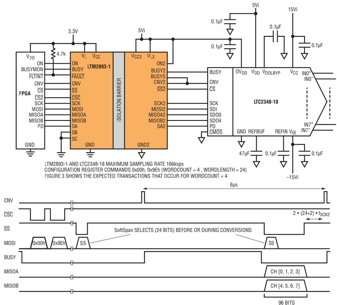
Additionally, with ADCs that support chaining (Figure 5), up to eight ADCs can be connected to a single LTM2893. Reading more than two parallel ADCs requires a write to the configuration register in the LTM2893 to select the number of devices. The configuration register allows the selection of two, four, six or eight devices to be accessed through the two MISOA and MISOB SPI outputs.
