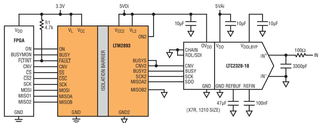
Figure 2. Standard digital isolator SPI read delays can add up to 38ns, reducing effective SCK frequency to approximately 25MHz.
