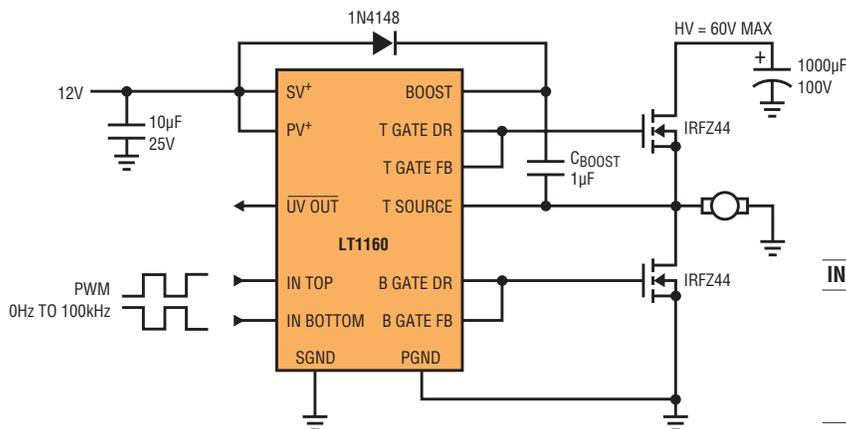
**LT1160/LT1162: 60V MAX SUPPLY REFERENCED DC MOTOR HALF-BRIDGE DRIVER**
