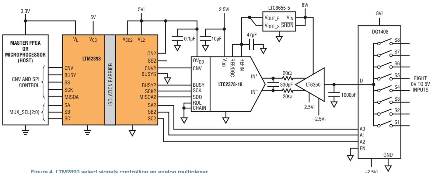
Figure 4. LTM2893 select signals controlling an analog multiplexer
