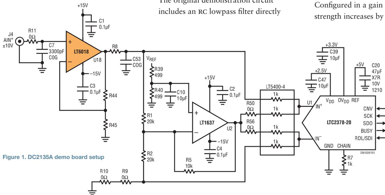
Figure 1. DC2135A demo board setup
