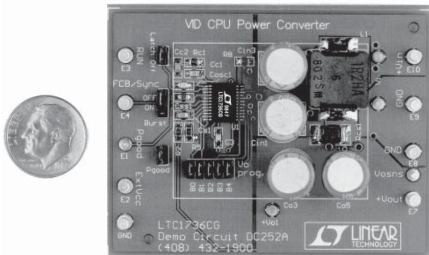
Figure 1. LTC1736 evaluation circuit: a complete 5V-24V to 0.9V-2V/12A converter in 2.15in<sup>2</sup> of PC board space
