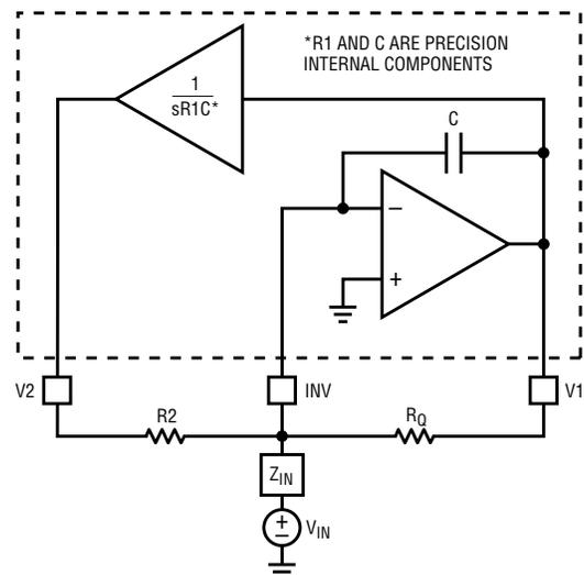
Figure 2. Single 2nd order Operational Filter section (inside dashed line) with external components added: resistor for  $Z_{IN}$  gives lowpass at V2, bandpass at V1; capacitor for  $Z_{IN}$  gives bandpass at V2, highpass at V1.
