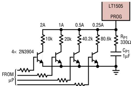
Figure 3. Programming of battery-charge current
