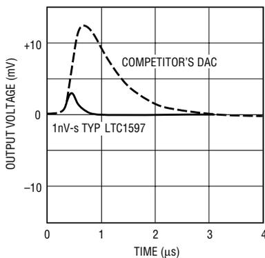
**Figure 5. The proprietary deglitcher** reduces the output glitch to less than 1nV-s, which is ten times less than any other 16-bit, voltage-output DAC. Further, the deglitcher makes the glitch uniform, independent of code.
