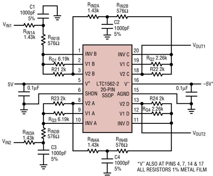
Figure 11. 400kHz dual 6th order Butterworth lowpass filter
