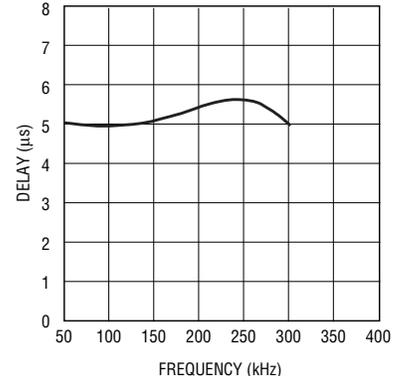
**Figure 8. Group delay response of Figure 5's circuit**
