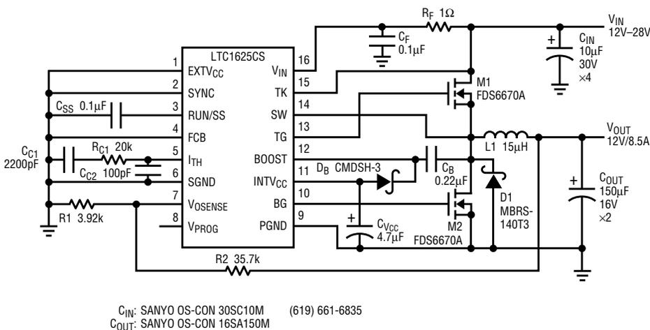
Figure 1. 100W, 12V, 8.5A supply
