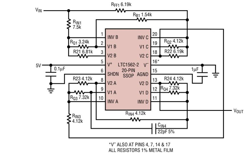
**Figure 5. 256kHz linear-phase 6th order lowpass filter**
