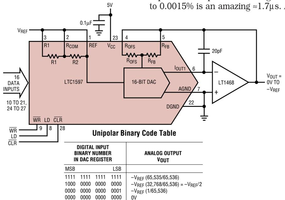
**Figure 3. With a single external op amp, the LTC1597 performs 2-quadrant multiplication with  $\pm 10$ V input and 0V to  $-V_{REF}$  output. With a fixed  $-10$ V reference, it provides a precision 0V to 10V unipolar output.**
