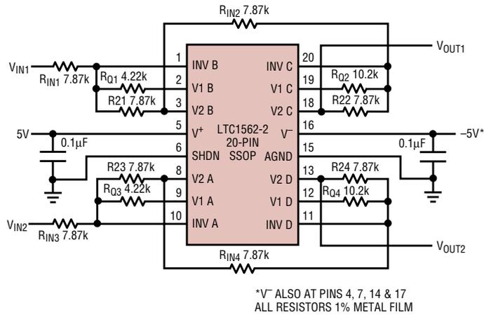
**Figure 3. Dual 4th order 200kHz Butterworth lowpass filter**
