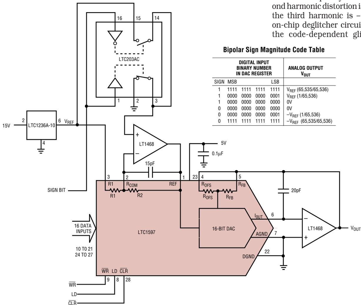
Figure 8. This 17-bit sign-magnitude DAC uses the LTC1597 in its unipolar mode with the reference bit inverted ( $-V_{REF}$ ) for the output range 0V to  $V_{REF}$ . When the sign bit changes, the analog switch changes the reference input polarity to noninverting ( $V_{REF}$ ) for the output range 0V to  $-V_{REF}$ . The resulting circuit produces an impressive bipolar zero error of 140μV (0.92LSB) max at room temperature—less than 1LSB at 17 bits.
