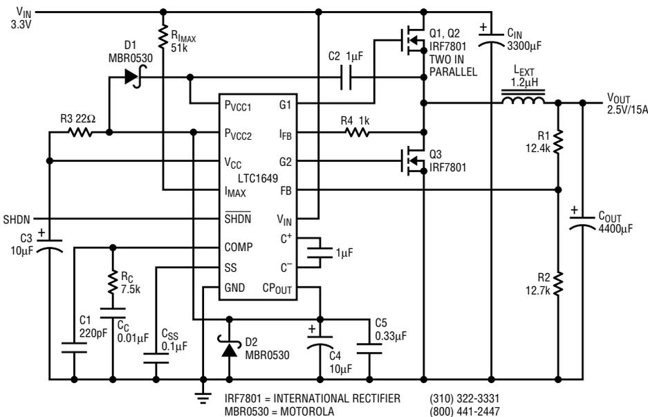
Figure 1. 3.3V to 2.5V/15A converter using the LTC1649
