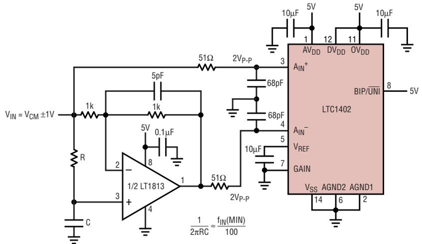
**Figure 8b. True differential inputs accept 4V<sub>p-p</sub> bipolar differential signal with 2V<sub>p-p</sub> swings on each input and an effective gain of 2 from the LT1813 inputs. SINAD = 70.7dB with a 1MHz input.**
