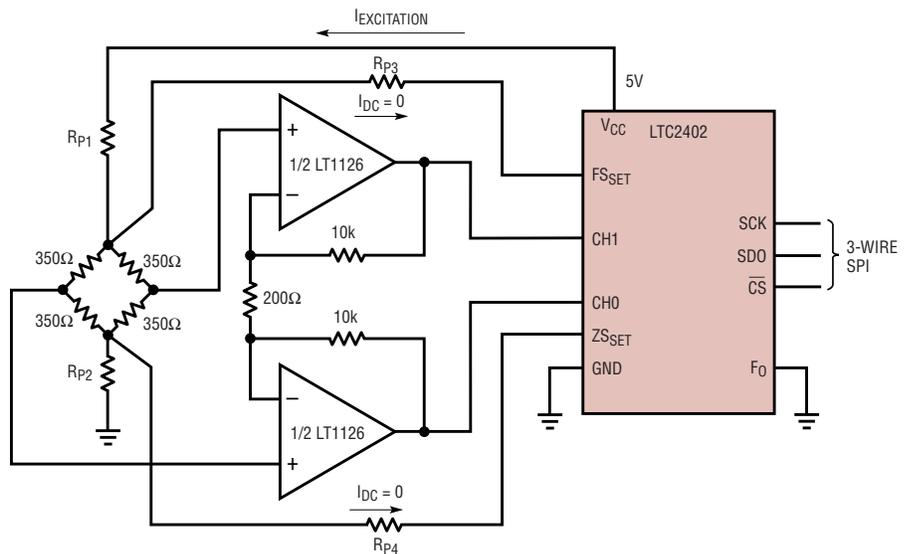
**Figure 7. 100,000 count pseudodifferential strain gauge application**
