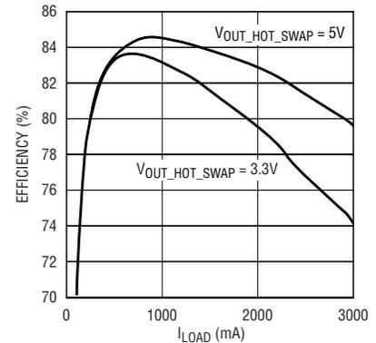
**Figure 6. LTC1735 efficiency vs load current ( $V_{OUT\_SWITCHER} = 3.3V$ )**
