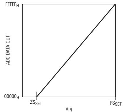
Figure 3. Transfer curve with zero-scale and full-scale set
