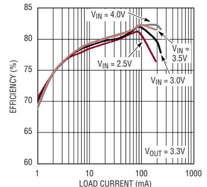
**Figure 8. Efficiency of Figure 7's circuit**
