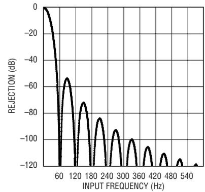
**Figure 6. Single-ended LTC2401/LTC2402 input rejection**
