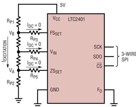
Figure 2. Half-bridge digitizer with zero-scale and full-scale sense
