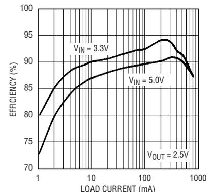
Figure 3. Efficiency of Figure 2's circuit
