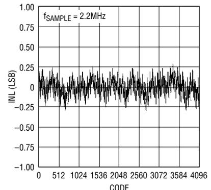
**Figure 7. Integral nonlinearity vs output code (unipolar 0V-4V)**
