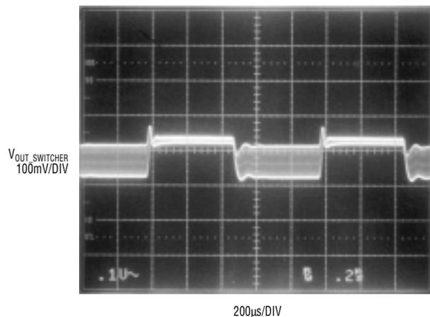
**Figure 8. LTC1735 transient response: load step = 0.5A–3.3A**
