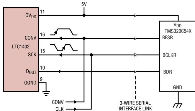
Figure 1a. DSP serial interface to the TMS320C54X
