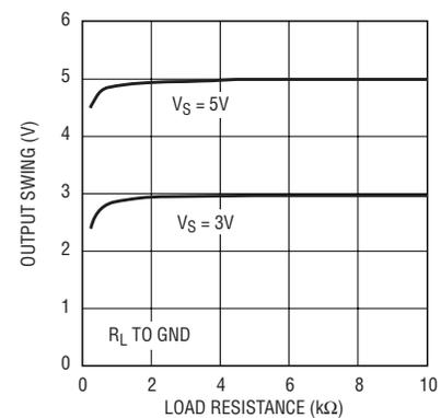
**Figure 3. LTC2050 output voltage swing vs load resistance**
