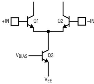
Figure 2. Voltage feedback input stage
