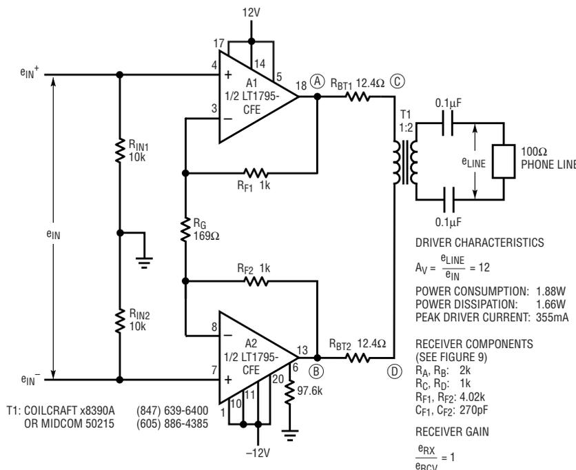
Figure 12 ADSL Full Rate downstream (CO) line driver
