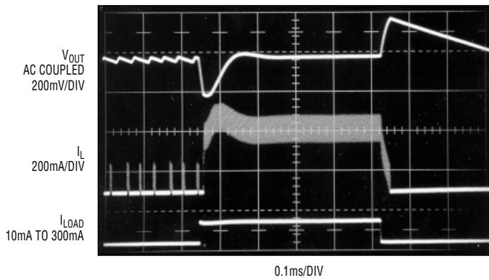
Figure 10. Transient response for Figure 9's circuit
