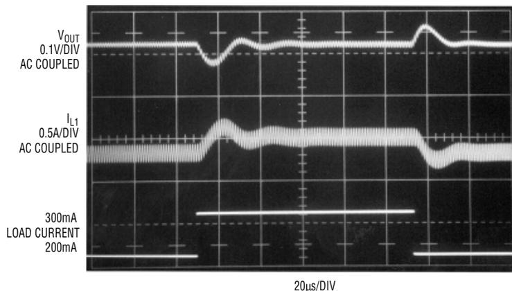
Figure 2. Transient response of Figure 1a's circuit
