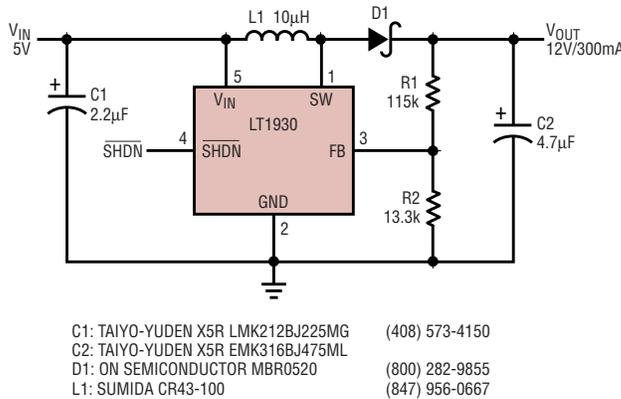
**Figure 3a. 5V to 12V/300mA step-up DC/DC converter**
