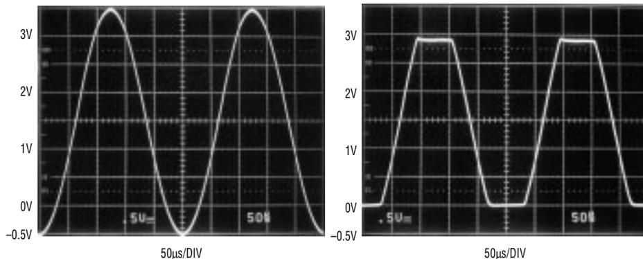
**Figure 1.** Input (left) and output (right) of an LT1677 configured as a voltage follower with input exceeding the supply voltage ( $V_S = 3\text{V}$ , input = -0.5V to 3.5V)
