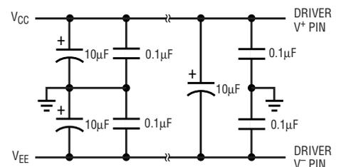
Figure 8. Recommended power supply bypassing for any design
