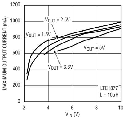
**Figure 2. Maximum output current vs input voltage**
