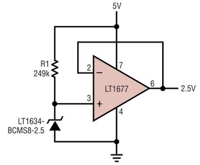
Figure 5. 2.5V reference from a 5V supply
