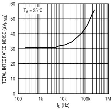
**Figure 4. LTC1563-X total integrated noise vs cutoff frequency**
