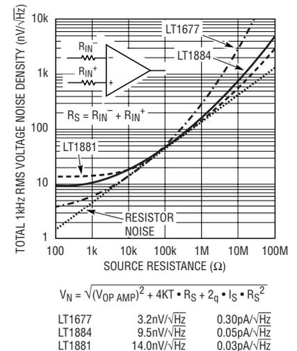
Figure 7. 1kHz noise voltage vs source resistance
