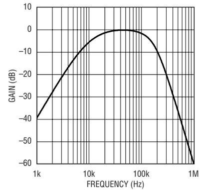
Figure 14. Frequency response of Figure 13's circuit
