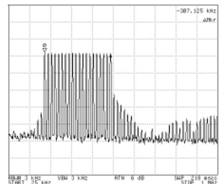
**Figure 5c. Spectrum of 20 carrier tones with I<sub>O</sub> of 2.2mA/amplifier**
