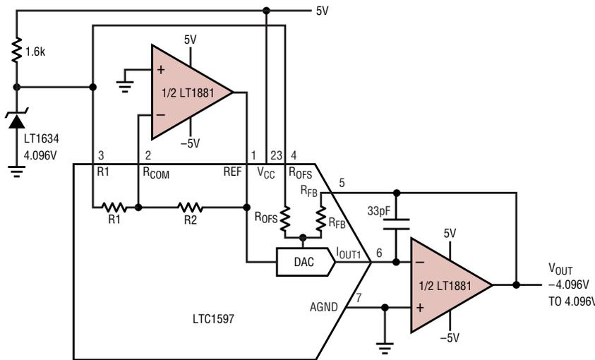
**Figure 10. 16-bit voltage-output DAC on a ±5V supply**
