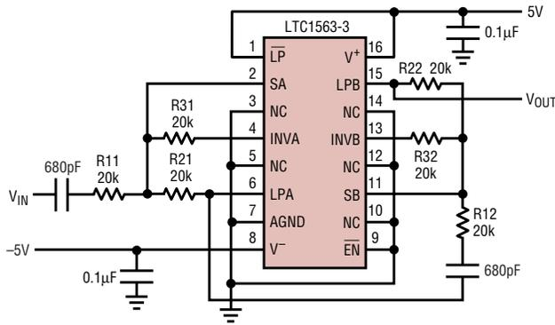
Figure 13. 50kHz wideband bandpass filter
