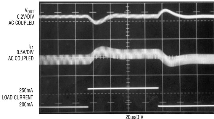
**Figure 4. Transient response of Figure 3a's circuit**
