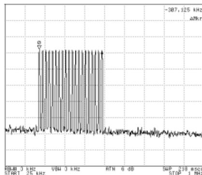
**Figure 5b. Spectrum of 20 carrier tones with I<sub>O</sub> of 12mA/amplifier**
