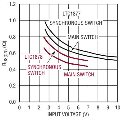
**Figure 1.  $R_{DS(ON)}$  for both switches vs input voltage**
