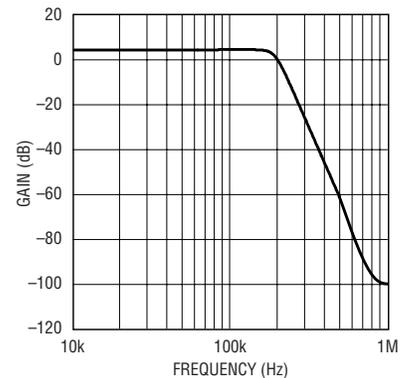
Figure 9b. Frequency response of Figure 9a's circuit
