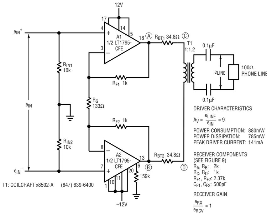
Figure 11. ADSL G.Lite downstream (CO) line driver
