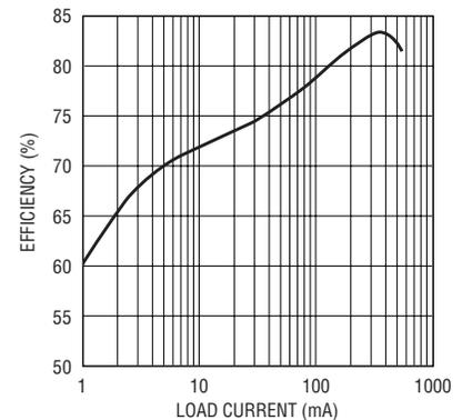
**Figure 9. 5V to 3.3V converter efficiency peaks at 83%**
