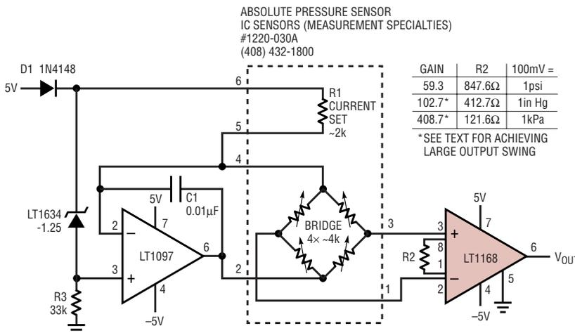
Figure 1. Simple barometer
