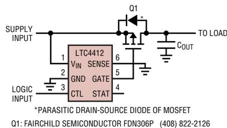
**Figure 7. Logic controlled high side power switch**
