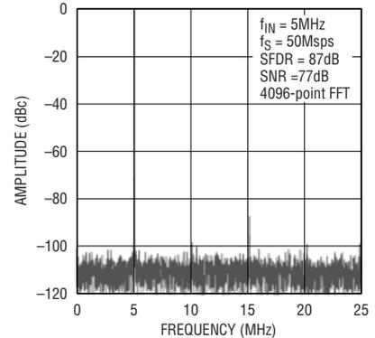
Figure 2. FFT with a 5MHz input signal
