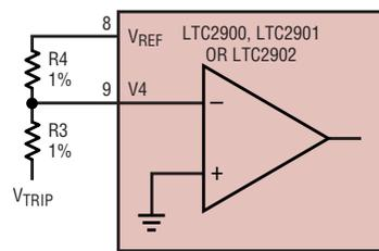
Figure 4. Setting the negative adjustable trip point (V<sub>TRIP</sub> = -V<sub>REF</sub>(R3/R4))
