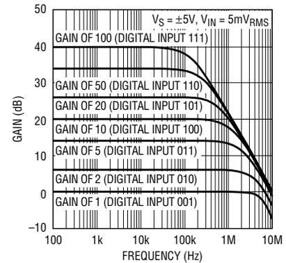
**Figure 2. LTC6910-1 frequency response at non-zero gain settings**
