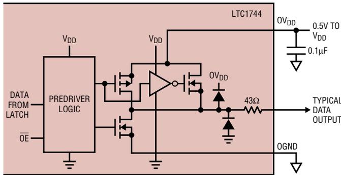
Figure 3. Equivalent circuit for a digital output buffer
