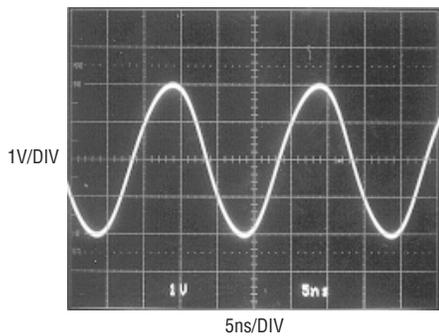
**Figure 3a. LT1818 response to 50MHz, 4V<sub>P-P</sub> sine wave maintains good fidelity.**
