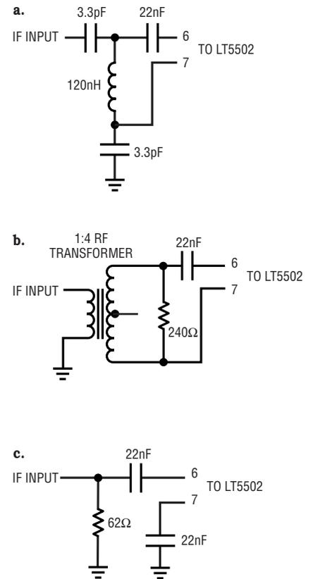
Figure 6. IF single-ended-to-differential input conversion and impedance matching
