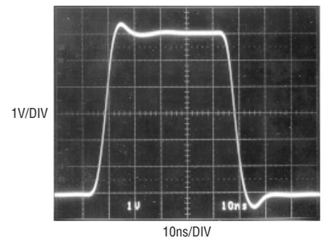
**Figure 7. Large-signal transient response of 20dB gain block**
