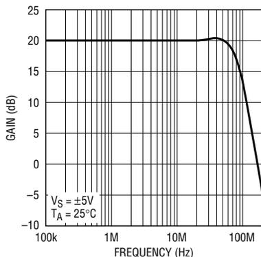
**Figure 5. Frequency-domain response of 20dB gain block**
