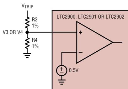
Figure 3. Setting the positive adjustable trip point, V<sub>TRIP</sub> = 0.5V(1 + R3/R4)
