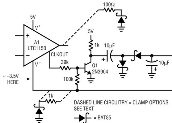
**Figure 1. Single rail powered amplifier has true zero volt output swing. A1's clock output switches Q1, driving diode-capacitor charge pump. A1's V<sup>-</sup> pin assumes negative voltage, permitting zero (and below) volt output swing.**
