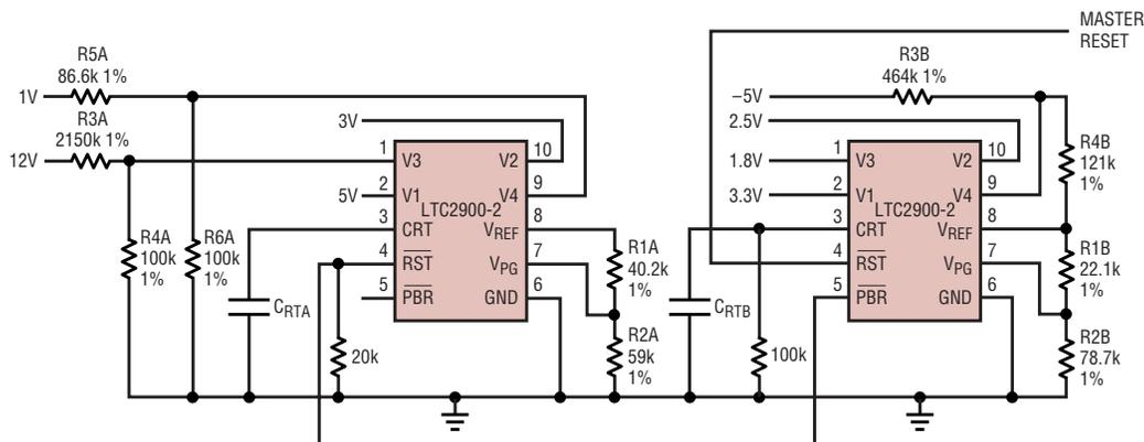
**Figure 7. Two supervisors cascaded to monitor eight voltages**
