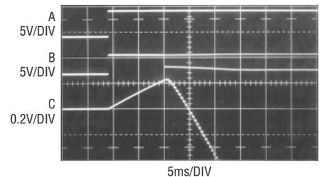
**Figure 2. Amplifier bootstrapped supply start-up. Amplifier V<sup>-</sup> pin (trace C) initially rises positive at 5V supply (trace A) turn-on. When amplifier internal clock starts (trace B, 5th vertical division), charge pump activates, pulling V<sup>-</sup> pin negative.**
