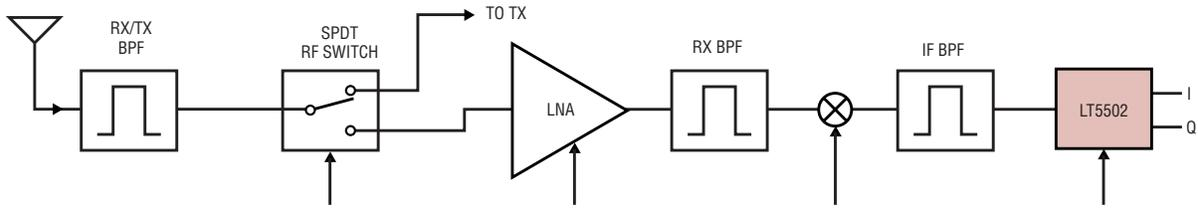
Figure 4. Example configuration of a 2.4 GHz-2.5GHz receiver
