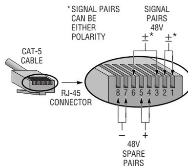
**Figure 1. Signal and spare pairs on RJ-45 connector**
