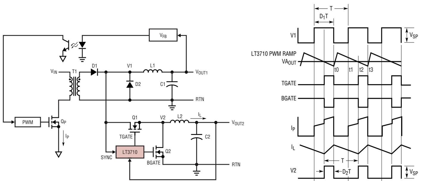
Figure 1. Simplified application schematic and key waveforms
