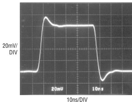
**Figure 6. Small-signal transient response of 20dB gain block**
