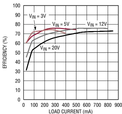
**Figure 6. Efficiency of the low profile SEPIC shown in Figure 4 is as high as 76% and increases as the input voltage approaches the output voltage.**
