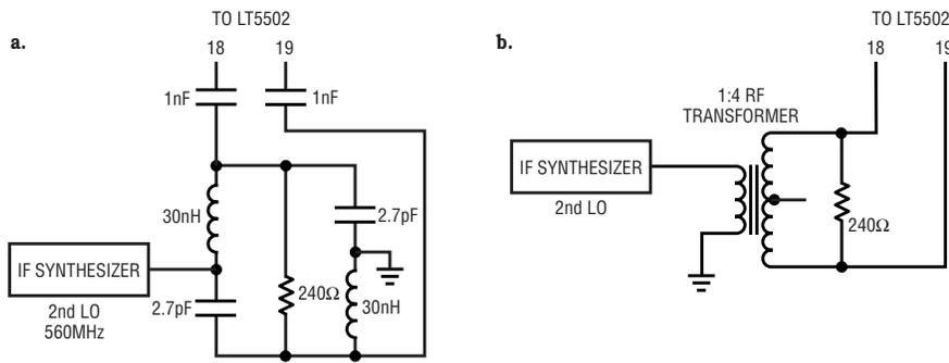
**Figure 7. LO single-ended-to-differential input conversion and impedance matching**
