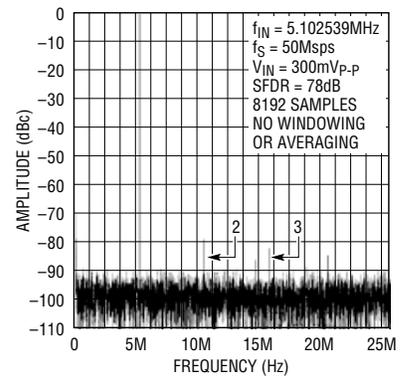
Figure 9. FFT of single ended ADC driver
