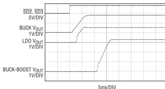
Figure 3. Output voltages during sequenced start-up
