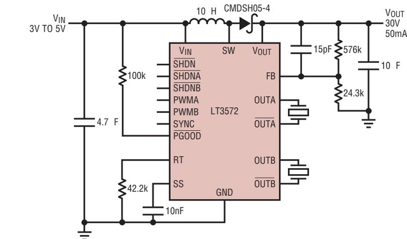
Figure 1. A typical LT3572 Piezo motor drive circuit
