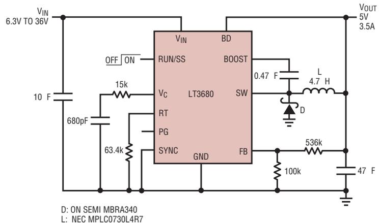
Figure 1. This 600kHz 6.3V–36V input DC/DC converter delivers 3.5A at 5V output.
