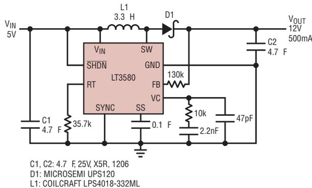
Figure 3. The high 2.5MHz switching frequency of this 5V to 12V boost converter allows the use of a tiny 4mm x 4mm x 1.7mm inductor.
