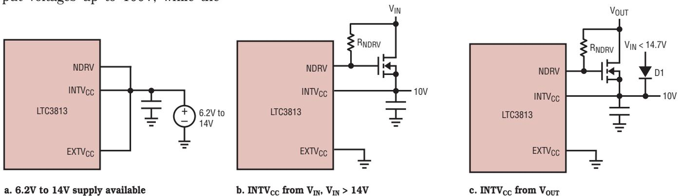
Figure 1. Three ways to generate IC/driver supply
