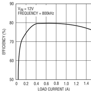
**Figure 7. Efficiency vs load current for Figure 6 application**
