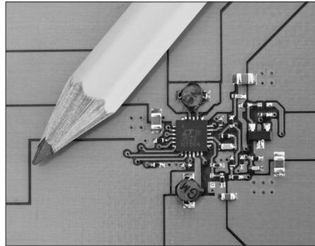
**Figure 1. Complete triple-output supply: Li-Ion to 3.3V, 1.8V, and 1.5V**
