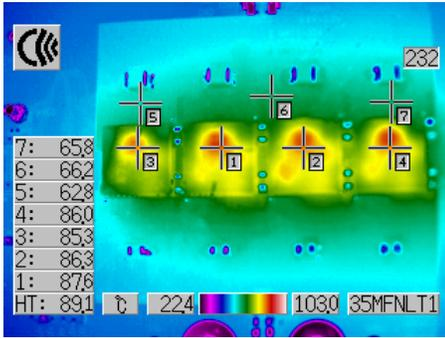
**Figure 7. Thermograph of four parallel LTM4601s without airflow (20V input to 1.5V output at 40A)**
