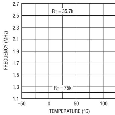
Figure 4. Typical internal oscillator frequency at  $V_{IN} = 5V$
