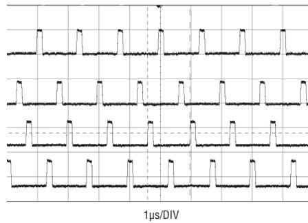
Figure 2. Individual LTM4601 switching waveforms for the circuit in Figure 1 shows the 90° out-of-phase relationship.
