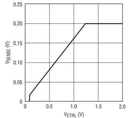
Figure 3. Dimming and shutdown using the CTRL pin
