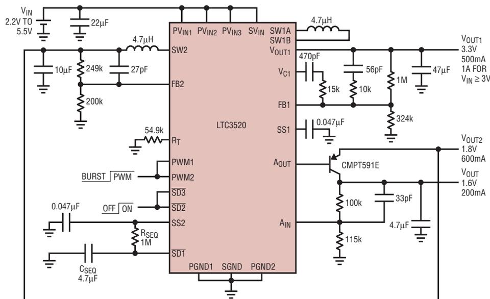
**Figure 2. Sequenced start-up, triple-output converter**
