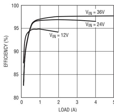
Figure 7. Efficiency of the circuit in Figure 6
