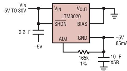
Figure 2. A simple reconfiguration of the µModule generates a negative output
