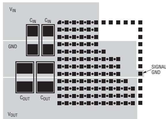
Figure 4. The LTM4601's pin layout promotes simple power plane placement and uncomplicated part paralleling
