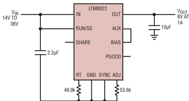
Figure 4. The LTM8022 can produce 8V, too
