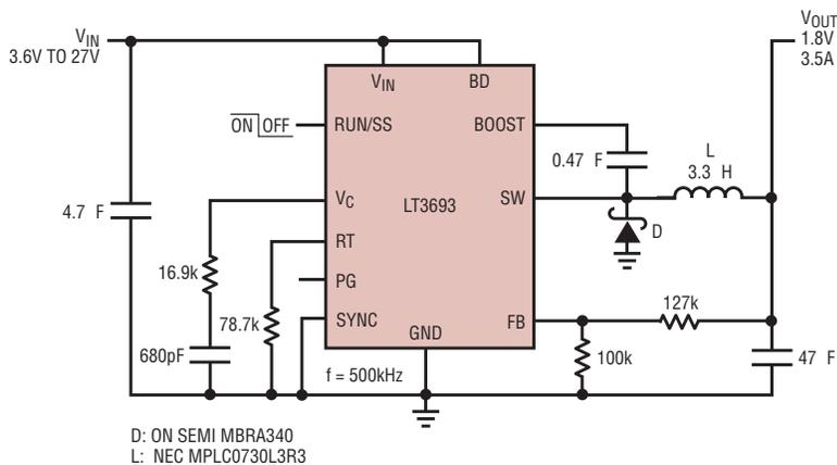
**Figure 4. This 500kHz 3.6V–27V input DC/DC converter delivers 3.5A at 1.8V output.**
