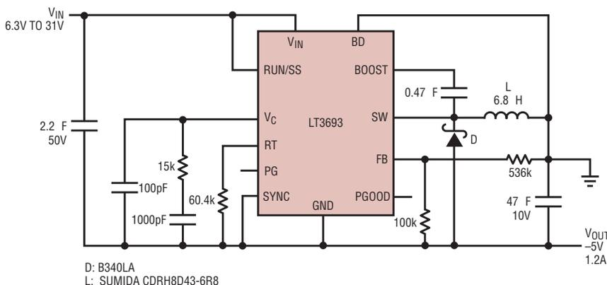
**Figure 5. This negative output DC/DC converter delivers 1.2A at –5V output.**
