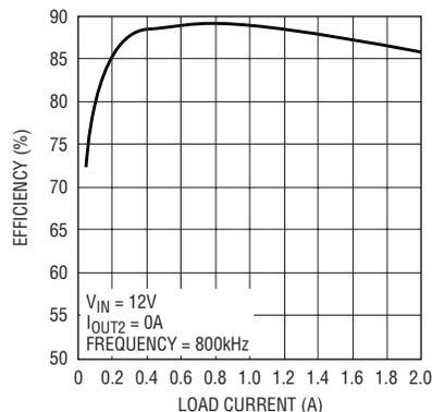
Figure 2. LT3500 switching regulator efficiency
