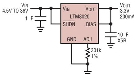
Figure 1. Generate 3.3V at 200mA with the LTM8020, two caps and a resistor
