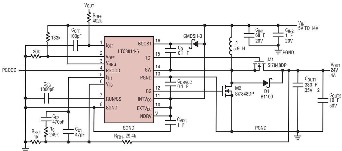
Figure 2. 5V-14V to 24V, 100W DC/DC converter
