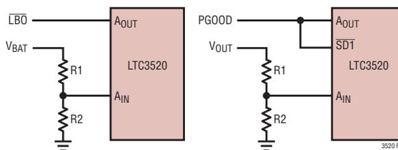
Figure 4. Implementation of low battery and power-good indicators
