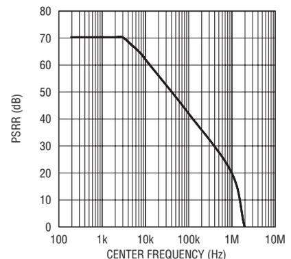
Figure 4. PSRR vs Frequency for  $V_{OUT2}$  for the application shown in Figure 1
