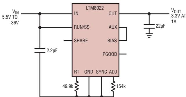
Figure 3. Produce 3.3V at 1A with LTM8022 and just four passive components
