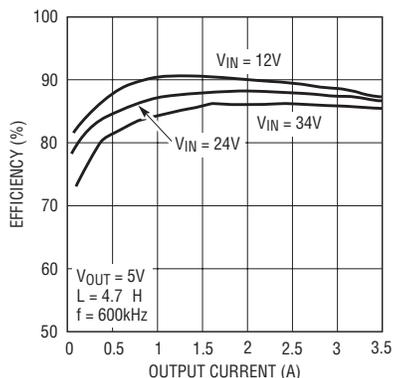
Figure 2. Efficiency vs load current for circuit in Figure 1
