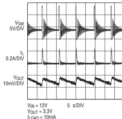
Figure 3. LT3680 Burst Mode operation at 10mA load
