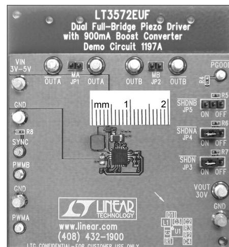
Figure 2. Typical layout for the Figure 1 converter
