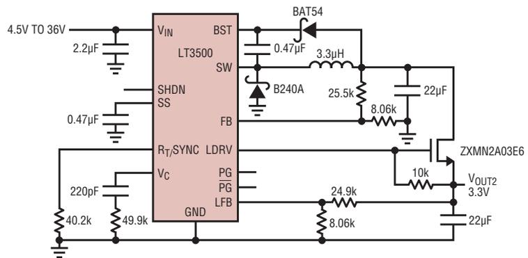
**Figure 6. High efficiency linear regulator**
