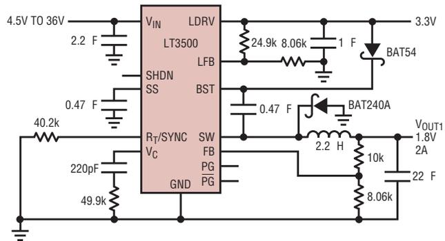
**Figure 5. 1.8V/2A step-down regulator**
