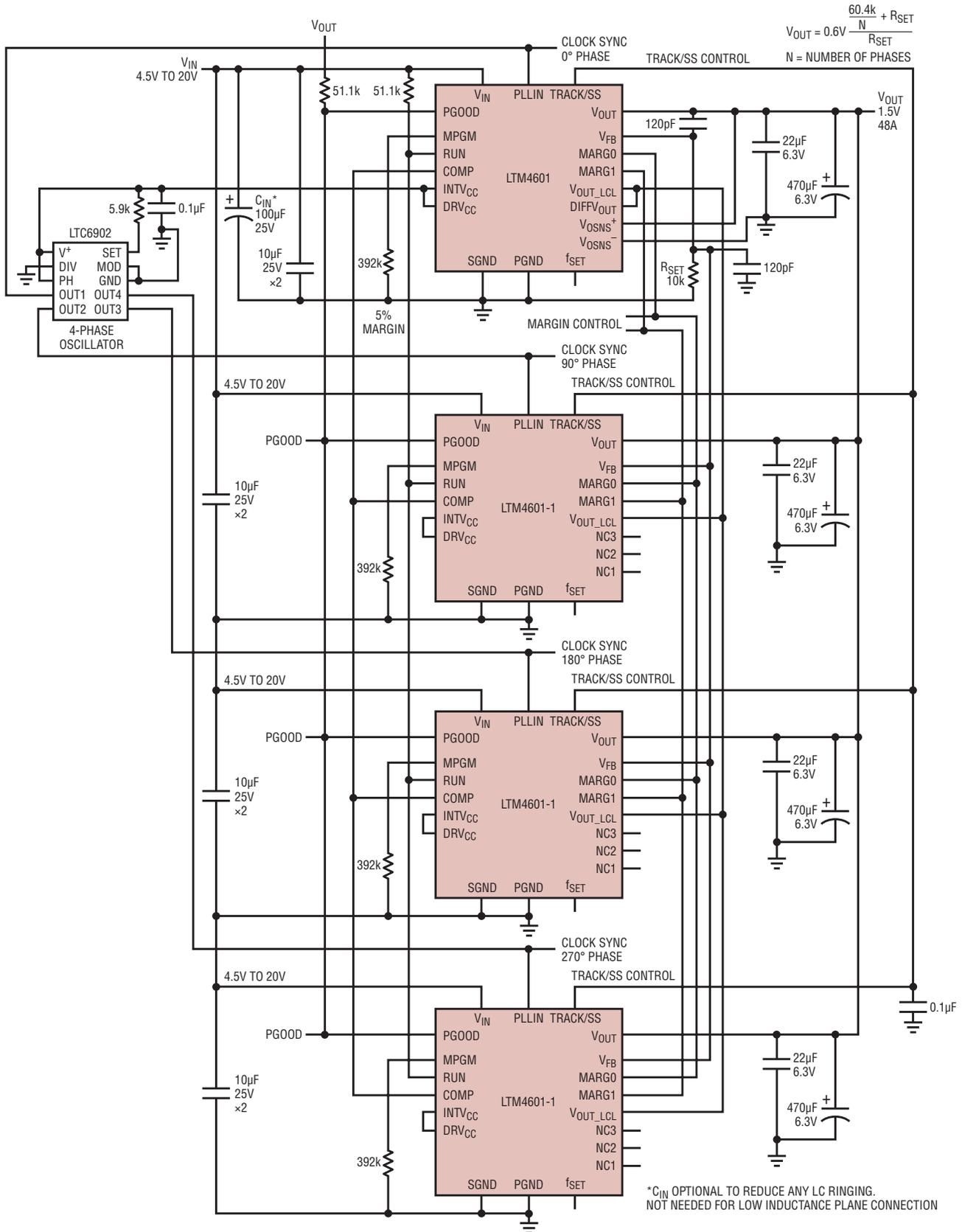
Figure 1. Designing a high density power supply for a limited space application could not be easier. Here, four LTM4601 µModule regulators are paralleled in a simple scheme. Board layout is just as easy, since there are so few external components.
