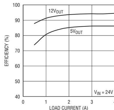
Figure 2. Efficiency of the converter in Figure 1
