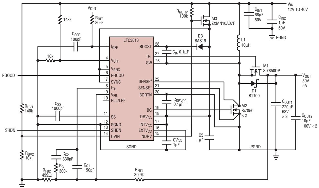
Figure 6. 12V-40V to 50V, 250W DC/DC converter
