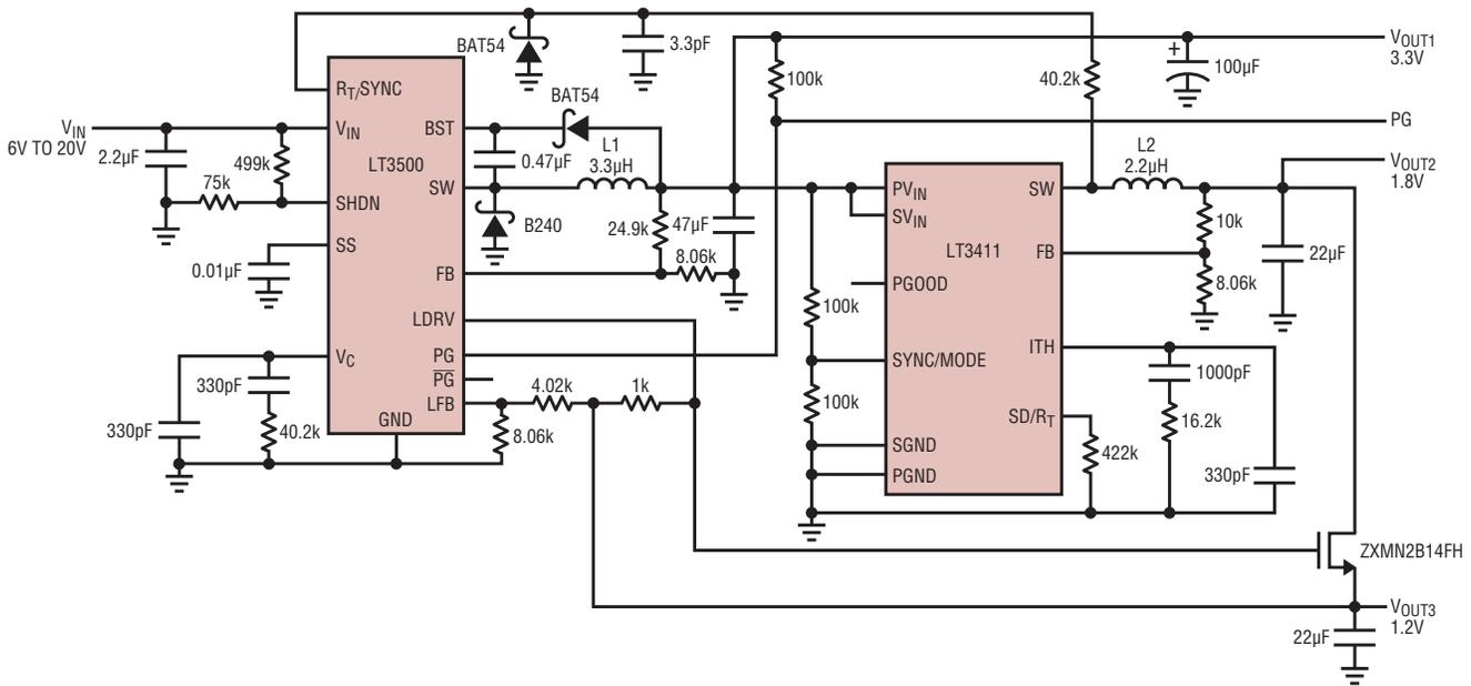
Figure 8. Triple output application
