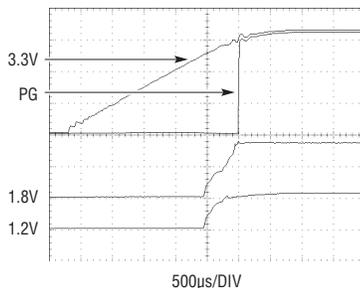
Figure 10. Start-Up waveforms for Figure 8 application
