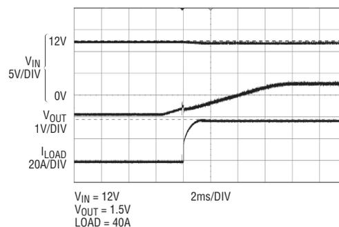
Figure 12. Soft-start ramp for four parallel LTM4601s
