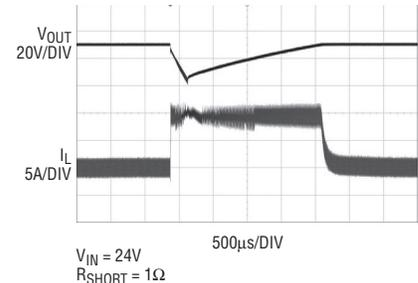
**Figure 5. Overcurrent performance of the circuit in Figure 2**
