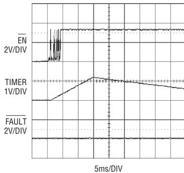
**Figure 2. TIMER blanking time prevents false fault reset from EN pin contact bounces.**
