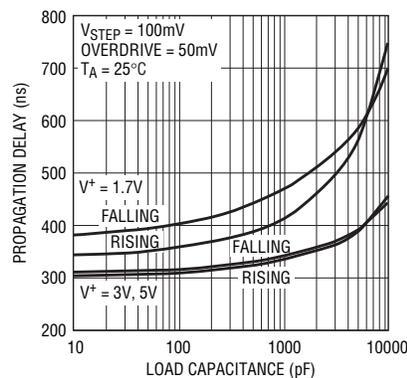
Figure 1. Speed is maintained with high capacitive loads
