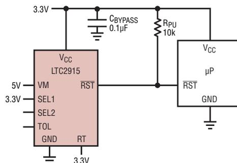
Figure 2. A 5V, -10% tolerance supply monitor with 200ms internal reset timeout
