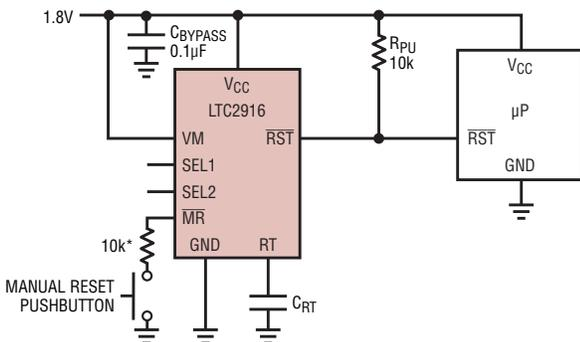
\*OPTIONAL RESISTOR RECOMMENDED TO EXTEND ESD TOLERANCE
