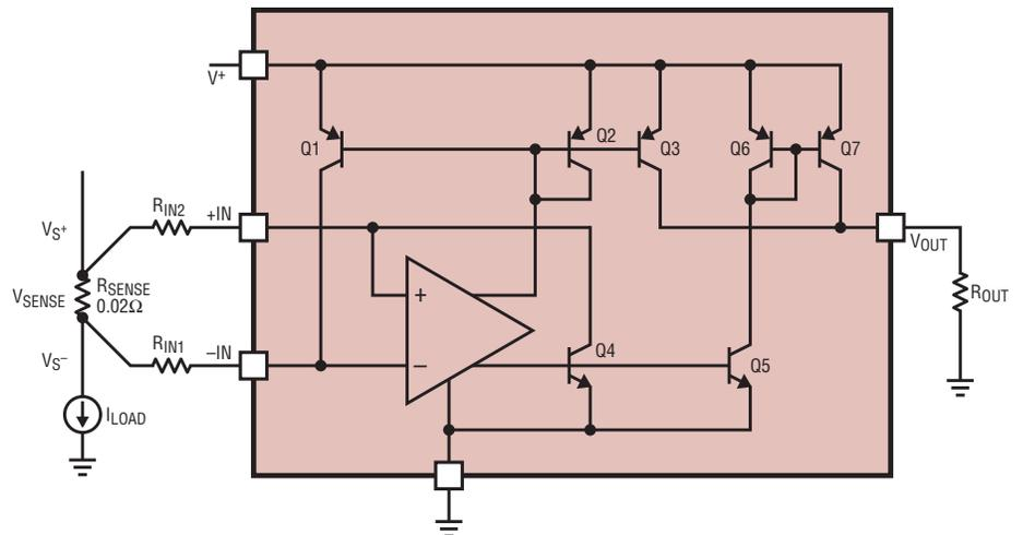
Figure 5. Block diagram of the LT6105
