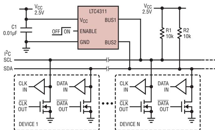
Figure 4. Typical LTC4311 application with low current shutdown
