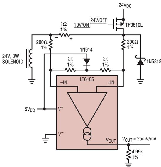
**Figure 8.** Similar circuit to Figure 6 but with solenoid grounded, so freewheeling forces inputs negative. Providing resistive pullups keeps amplifier inputs from falling outside of their accurate input range.
