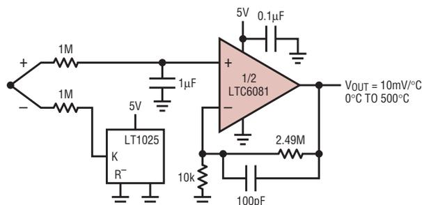
SENSOR: OMEGA 5TC-TT-K-30-36 K-TYPE THERMOCOUPLE
