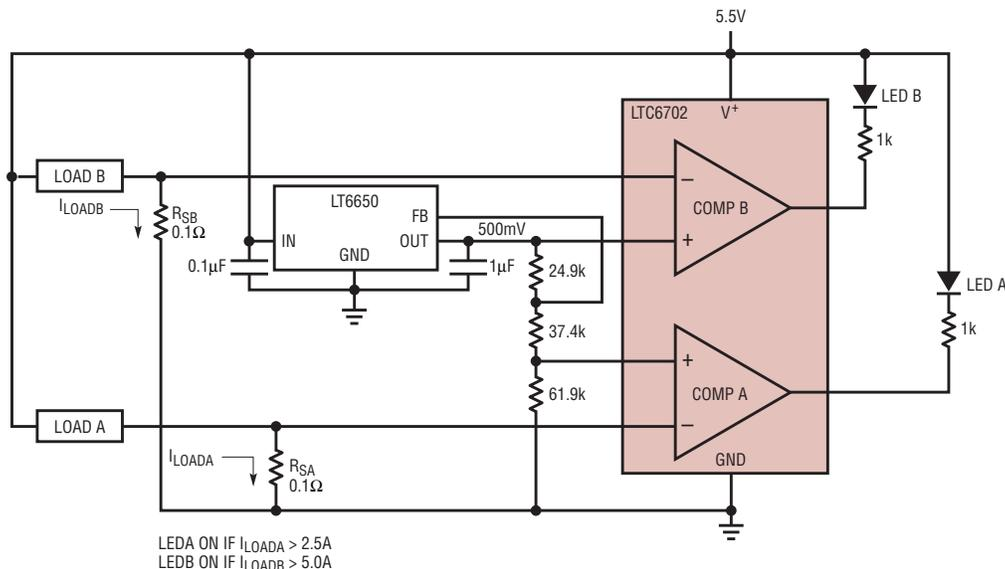
Figure 4. This micropower dual low side current sense alarm can drive an LED or relay
