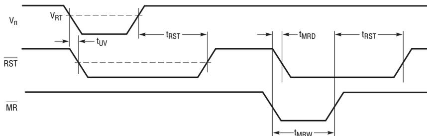
Figure 8.  $\overline{\text{MR}}$  timing diagram
