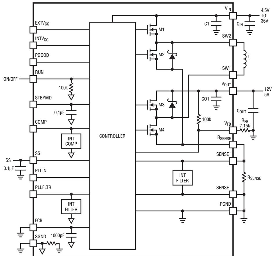
**Figure 2. Simplified block diagram of the LTM4607**
