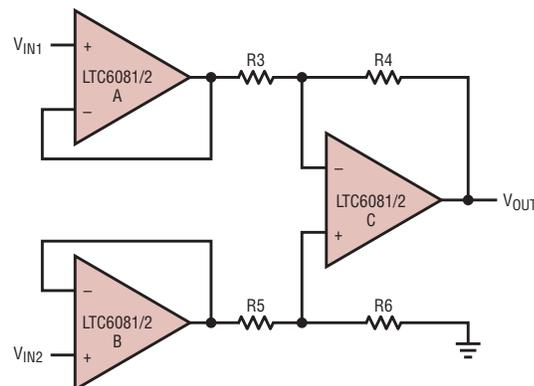
Figure 3. Instrumentation amplifier with unity gain buffers
