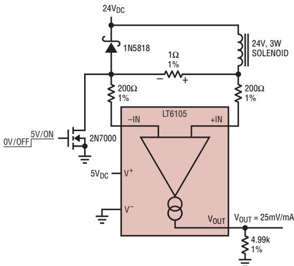
**Figure 6.** Simplest form of solenoid driver. The LT6105 monitors the current in both on and freewheel states. Lowest common mode voltage is 0V, while the highest is 24V plus the forward voltage of the Schottky diode. See waveforms, Figure 7.
