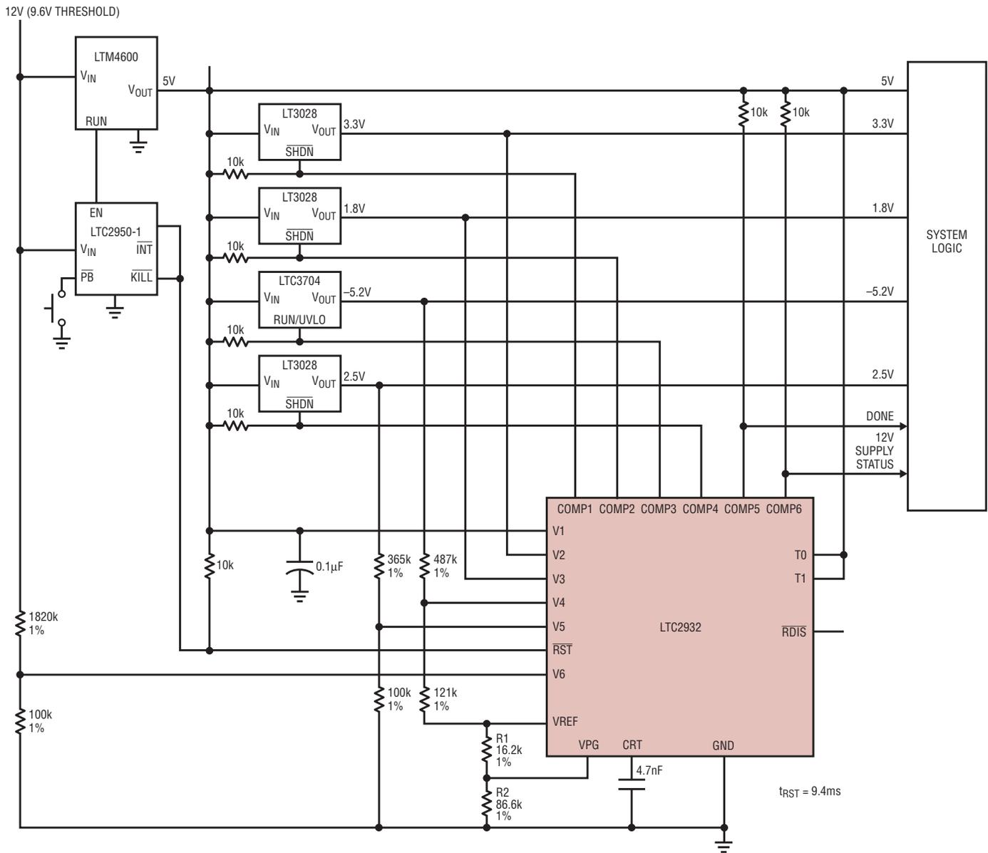
Figure 7. Five supply 12.5% tolerance power-up sequencer with pushbutton
