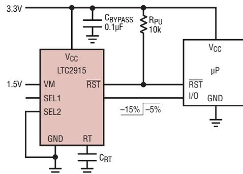
Figure 6. 1.5V supply monitor with tolerance control for margining, -5% operation with -15% margining
