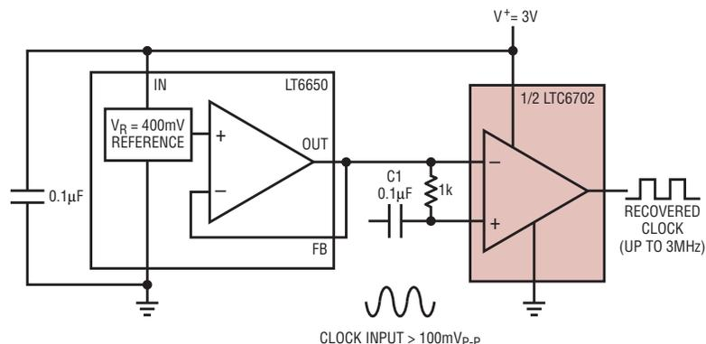
Figure 2. Clock recovery circuit efficiently recovers clock signals up to 3MHz
