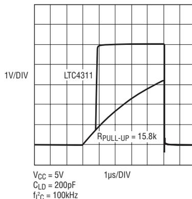
Figure 2. Comparison of I<sup>2</sup>C waveform for the LTC4311 vs resistive pull-up
