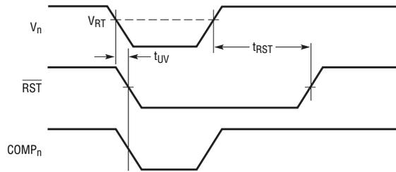
**Figure 5.  $\overline{RST}$  timing diagram**
