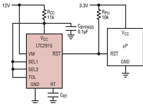
Figure 1. A 12V supply monitored from 12V, utilizing internal shunt regulator with 3.3V logic out
