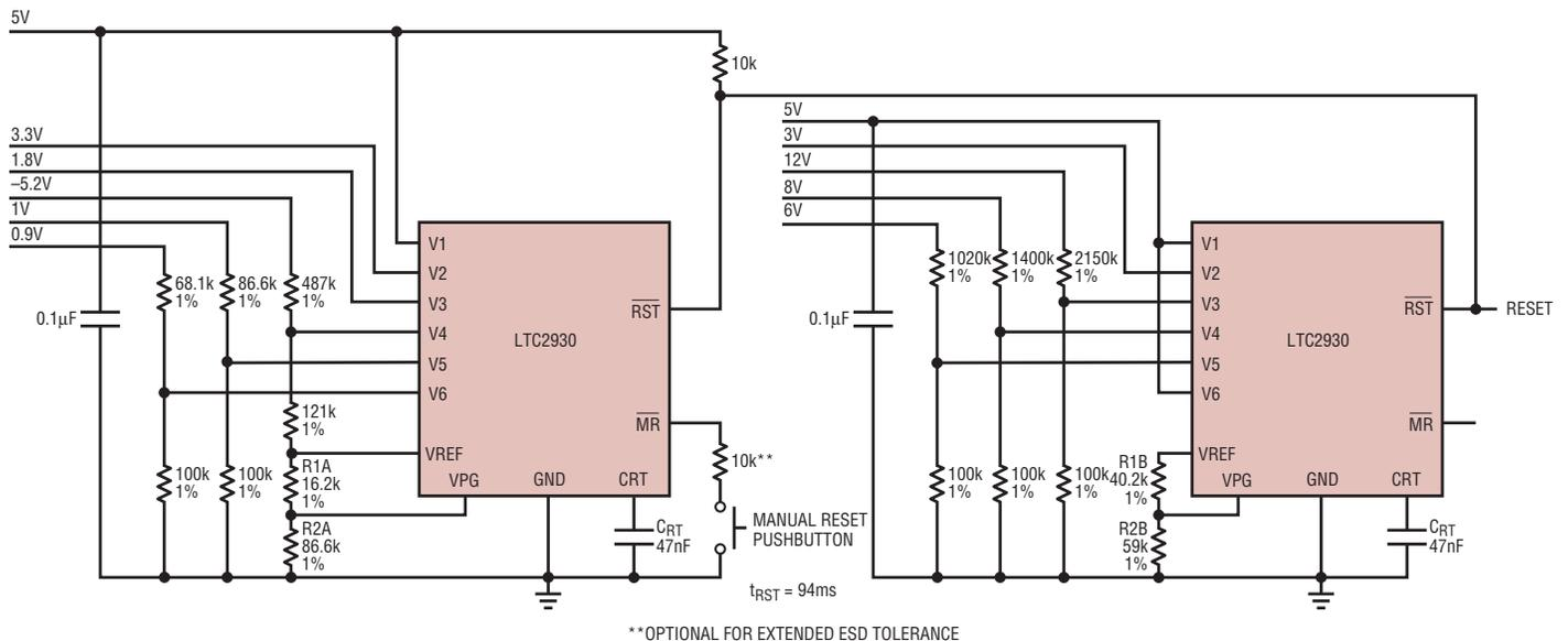
**Figure 6. Wired-OR system reset**
