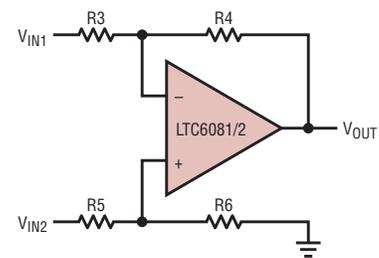
**Figure 4. Difference amplifier with no input buffers**
