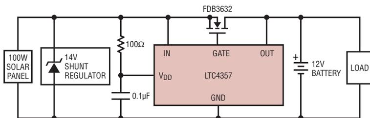
Figure 2. Solar panel charging 12V battery through ideal diode to prevent back feeding
