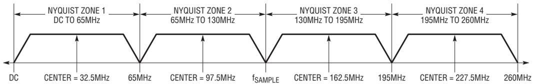
**Figure 2. Nyquist zones for 130MHz sample rate**
