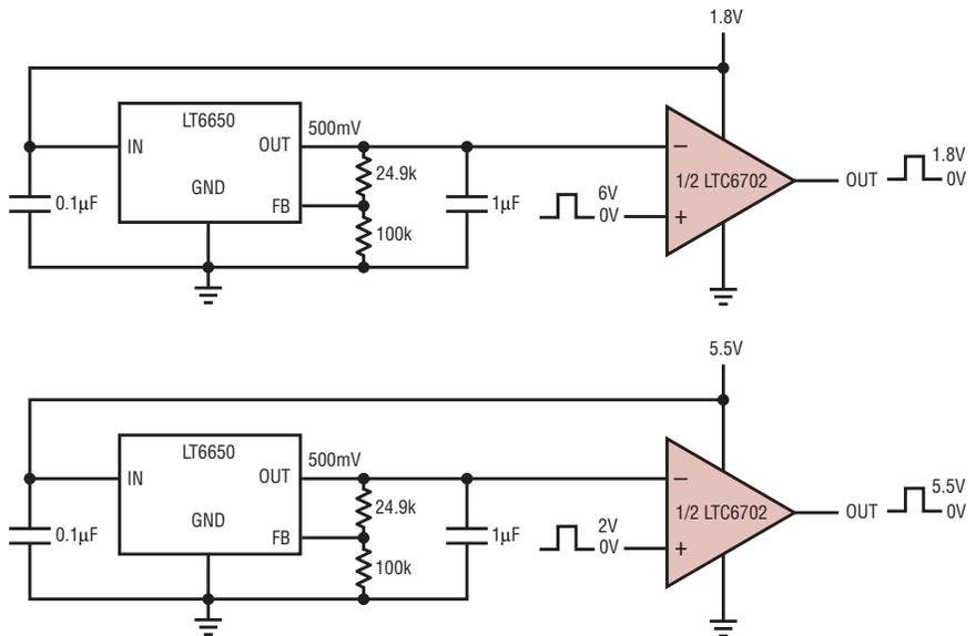
Figure 3. Level translation without the need of an additional supply or pull-up resistor
