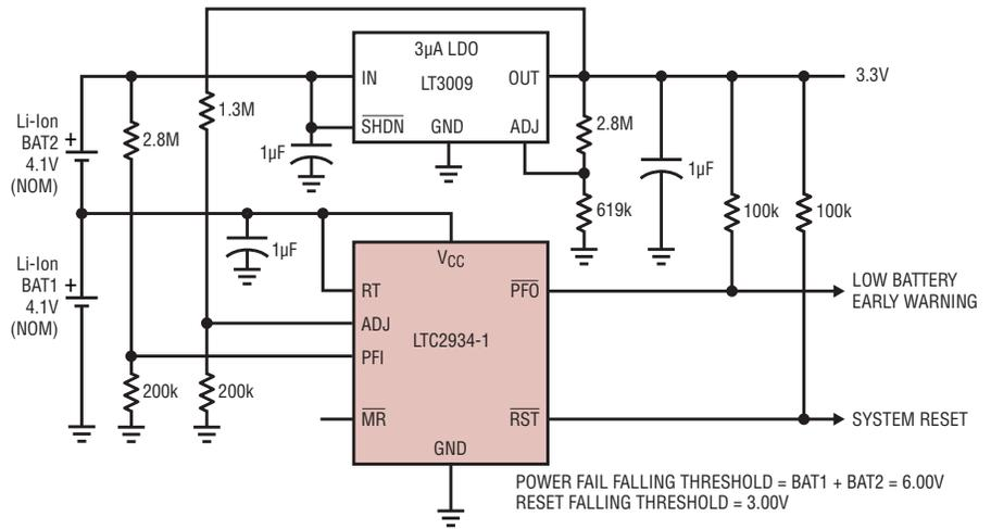
Figure 4. Stacked Li-ion cell and LDO supervisor
