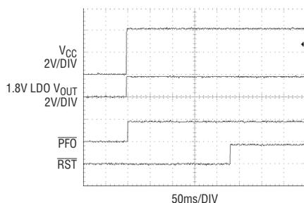
Figure 2. Typical power-up waveforms
