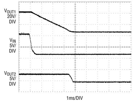
Figure 3. Output waveforms when power is removed from the circuit in Figure 2
