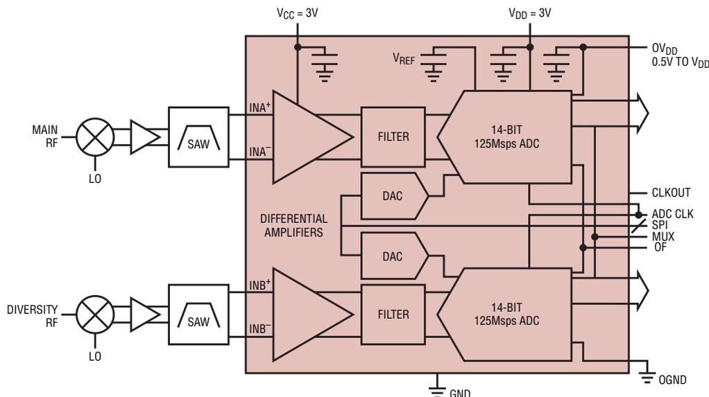
Figure 1. LTM9002 used for a Main/Diversity receiver.
