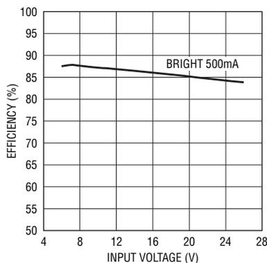
Figure 3. Efficiency for Figure 1
