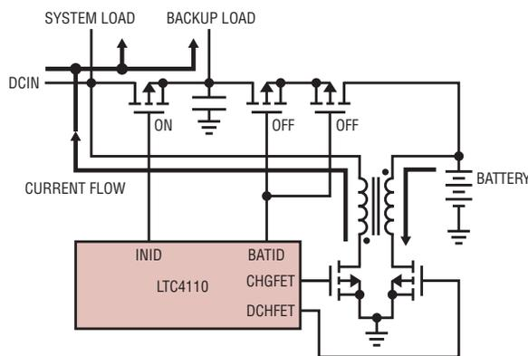
Figure 4. LTC4110 in calibration mode
