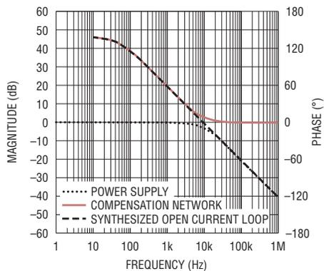
Figure 3. Current loop Bode design with power supply having first order transfer function
