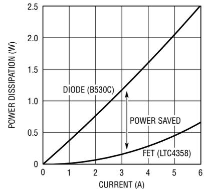
Figure 2. The LTC4358 ideal diode takes on a 5A B530C Schottky diode. The LTC4358 easily wins in voltage drop, power loss and package size.
