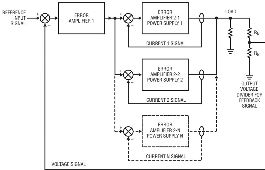
Figure 2. Power system control loop
