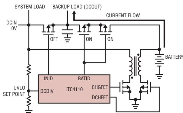
Figure 5. The LTC4110 in battery backup mode
