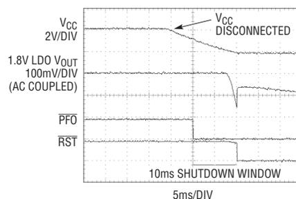
Figure 3. Typical power-down waveforms
