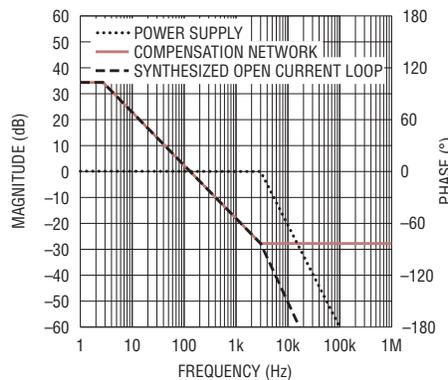
Figure 4. Current loop synthesis with 0,-1,-2 shape
