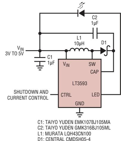
Figure 3. LED driver in Buck-Boost mode driving one LED
