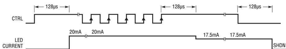
Figure 2. Current programming and shutdown timing
