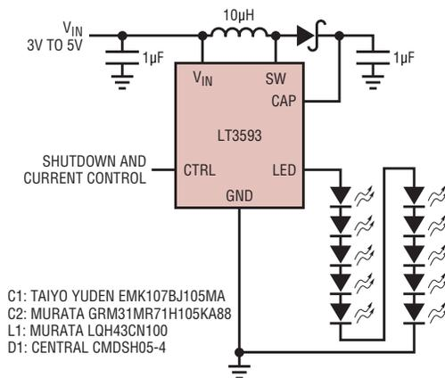
Figure 1. LED driver for ten white LEDs
