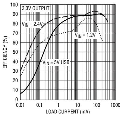
Figure 2. Converter efficiency for the circuit of Figure 1
