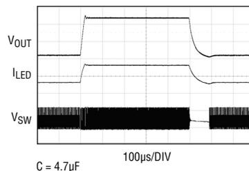
Figure 4. Switching between dim (50mA) and bright (500mA) modes with 4.7µF output cap
