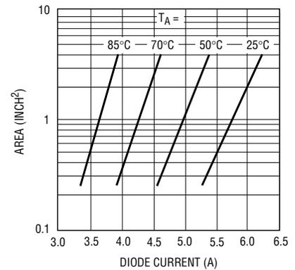
Figure 4. Maximum diode current vs PCB area
