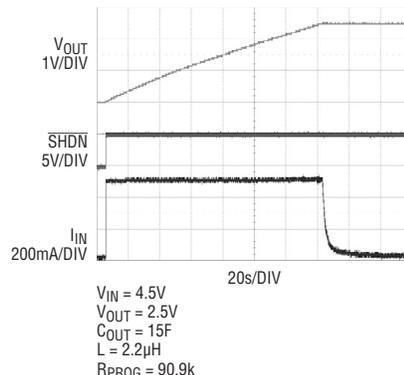
**Figure 4.** Waveforms of input current and  $V_{OUT}$ , charging large  $C_{OUT}$  from 0 volts
