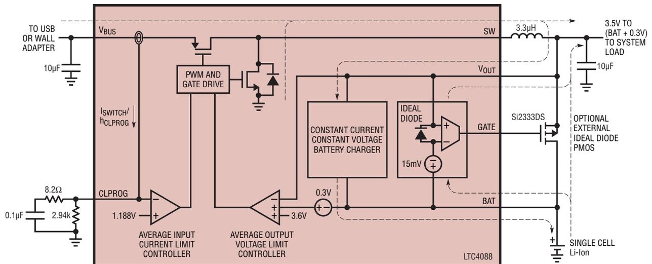
**Figure 3. Switching PowerPath block diagram.** The big advantage of a switching PowerPath scheme over a linear PowerPath is that the path from  $V_{IN}$  to  $V_{OUT}$  maintains relatively high efficiency regardless of the  $V_{IN}/V_{BAT}$  ratio.
