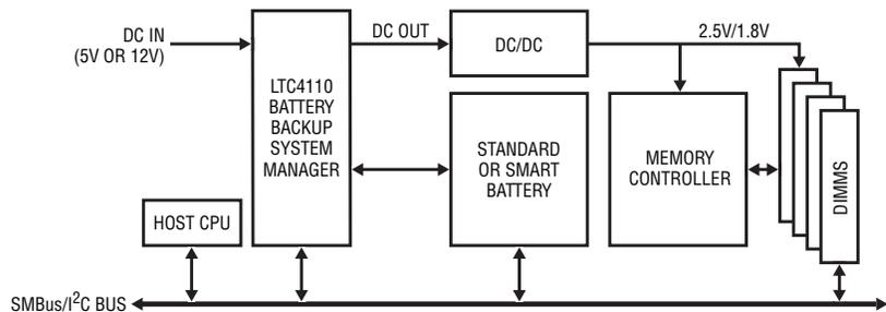
Figure 1. Block diagram of LTC4110 in a CPU/server system
