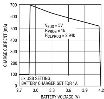
**Figure 4. Input power limited charge current**
