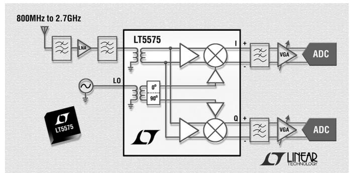
and WiMAX basestation receivers. The LT5575's extended operating frequency range from 800MHz to 2.7GHz covers all of the cellular and 3G infrastructure, WiMAX and RFID bands with a single part. Its capability to convert from RF directly to baseband at DC or low frequency results in simplified receiver designs, reduced component count and use of lower cost, low frequency components.
