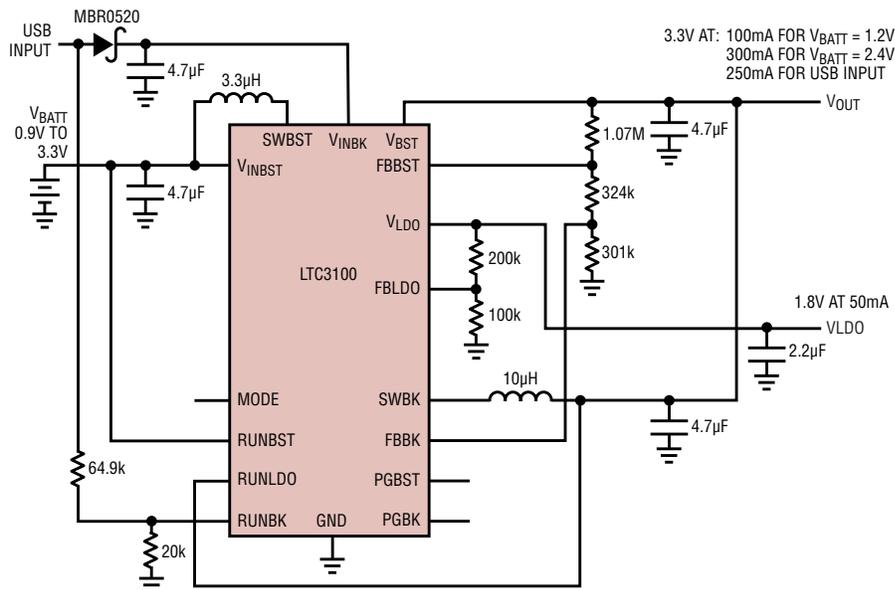
Figure 1. Multiple-input source 3.3V and 1.8V converter
