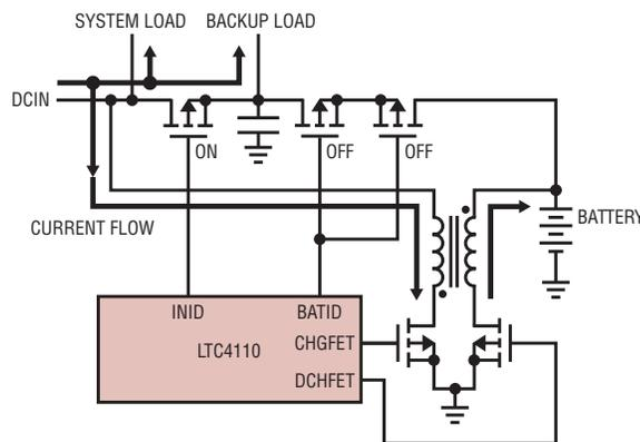
Figure 3. The LTC4110 in charge mode
