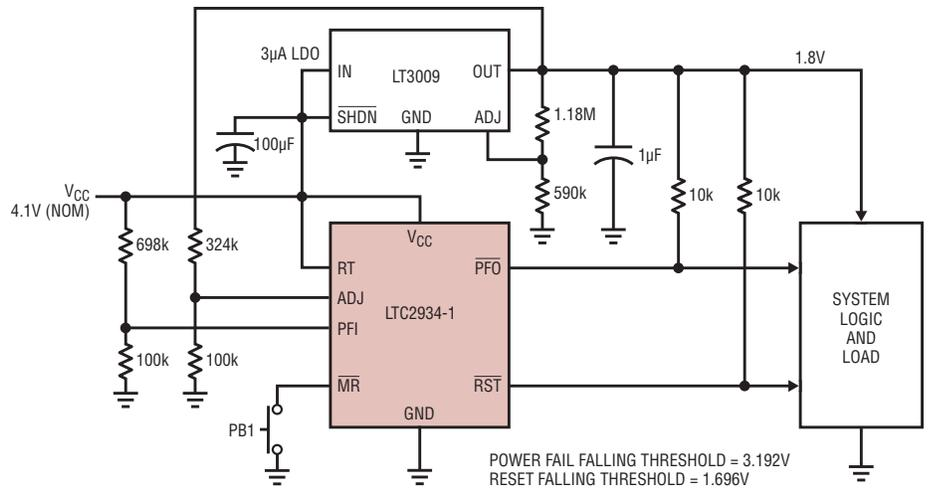
Figure 1. Typical supply monitor application
