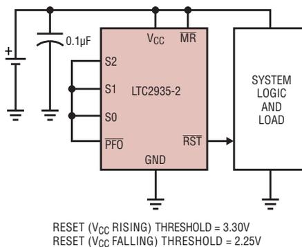
Figure 5. Active threshold control
