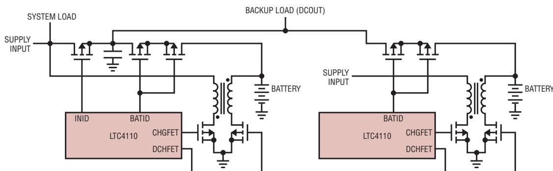
Figure 6. Dual LTC4110 system using standard batteries
