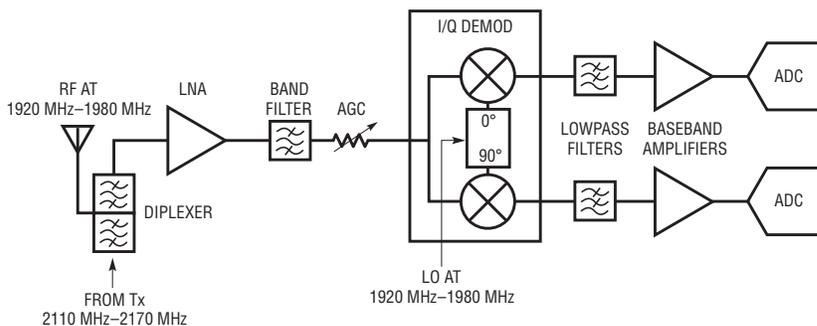
Figure 1. Direct conversion receiver architecture
