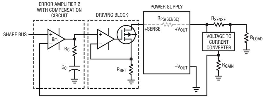
**Figure 5. Current loop functional block diagram**
