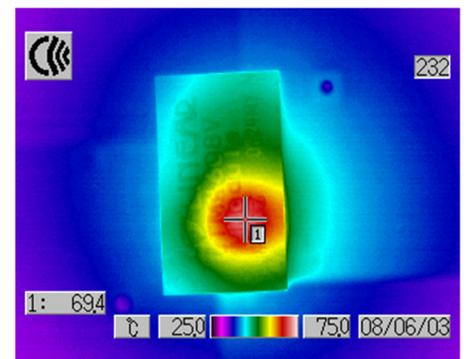
Figure 7. Good thermal balance is maintained between two paralleled LTM4608 boards supplying 16A output current.
