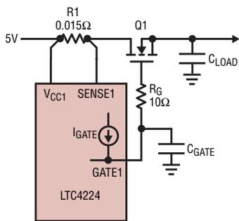
**Figure 3. A method to adjust inrush current by gate capacitor.  $R_G$  prevents parasitic self-oscillation in Q1**
