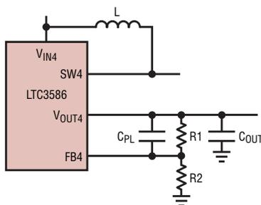
**Figure 5. Boost converter application circuit**
