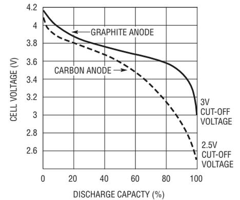
**Figure 4. Li-ion discharge voltage profile for different anode materials**
