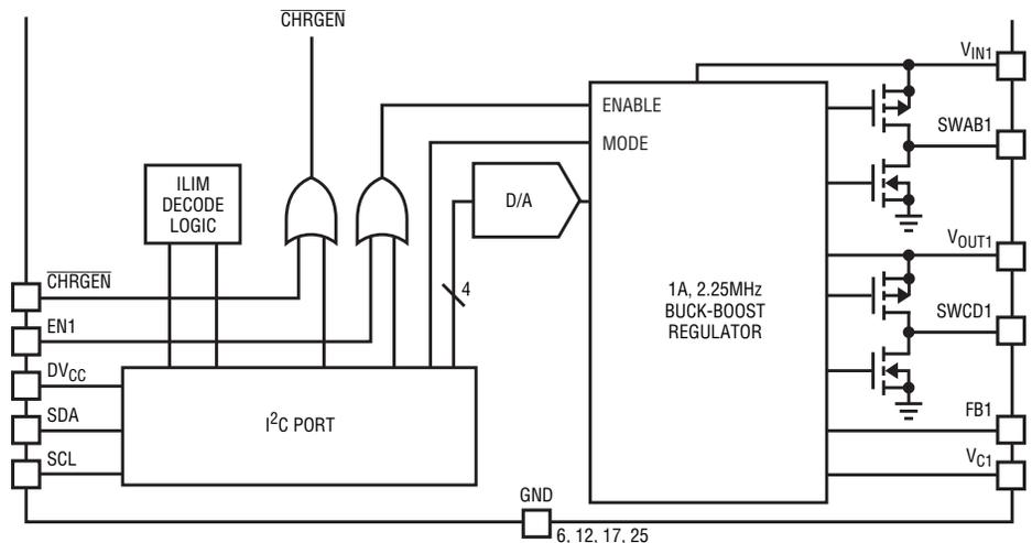
**Figure 6. The LTC3567 I/O and DC/DC output voltage control interface**
