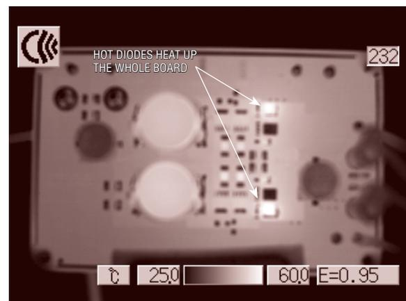
b. Thermal image of the board in Figure 2 built up with boost diodes
