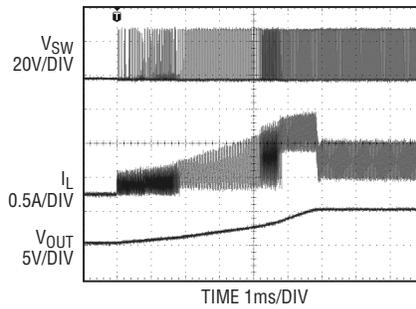
Figure 3. Soft-start waveforms
