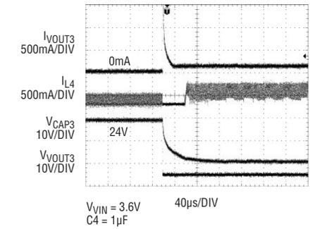
**Figure 6. Fault detection of a short circuit event**
