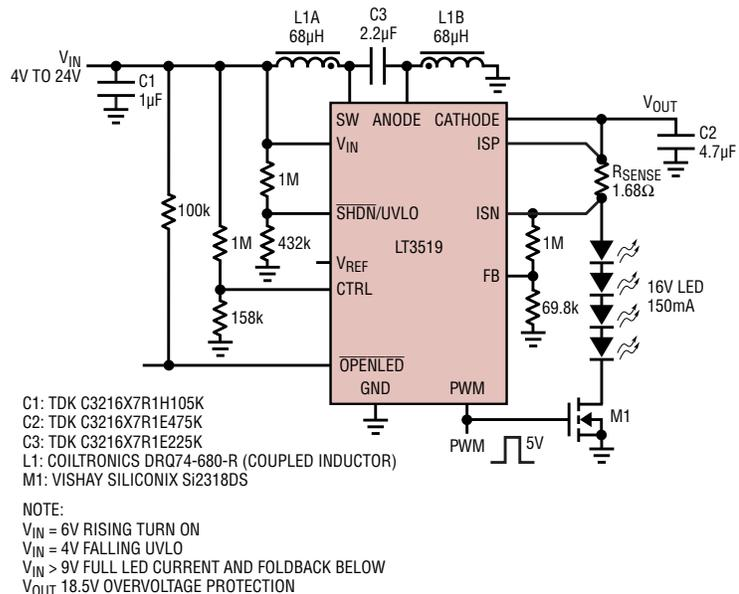
Figure 3. A SEPIC LED driver with short-circuit protection
