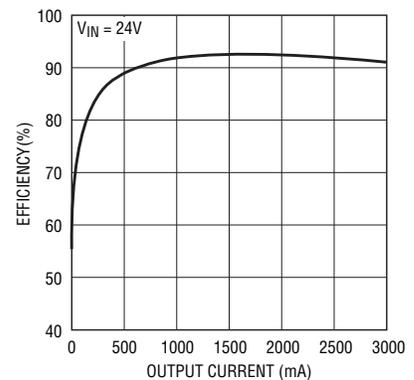
Figure 3. The LTM8025 boasts high efficiency.
