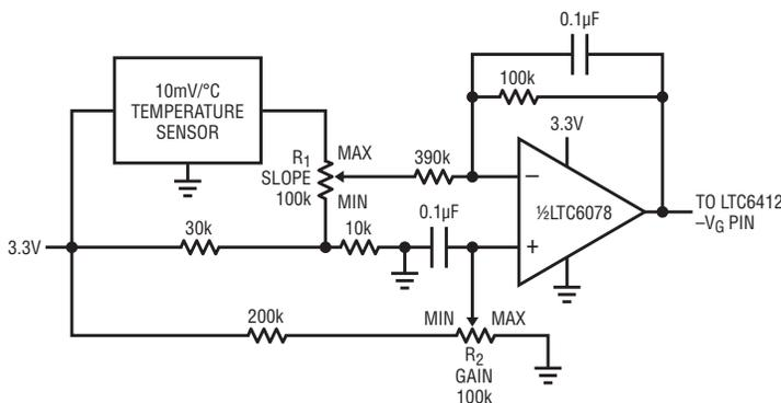
Figure 10. Application circuit for static gain adjust and temperature gain slope compensation using a PTAT temperature sensing IC. Adjust R1 and R2 as needed and route output to  $-V_G$  control terminal of the LTC6412.
