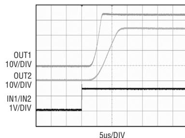
Figure 3. Turn-on delay and rise time for OUT1 and OUT2
