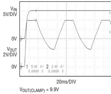
Figure 8. Overvoltage fault operation
