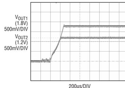
Figure 12. Start-up waveforms for the circuit in Figure 11
