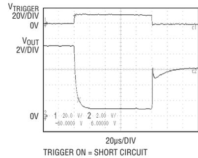
Figure 9. Overcurrent fault operation
