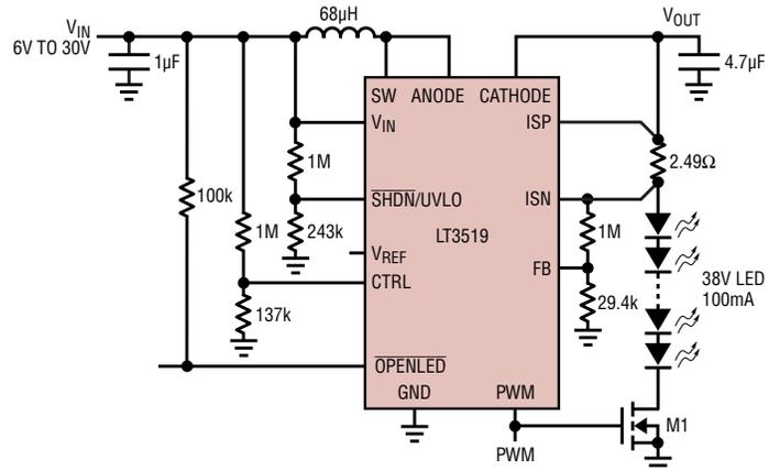
Figure 1. A 4W boost LED driver with 89% efficiency at 12V<sub>IN</sub>
