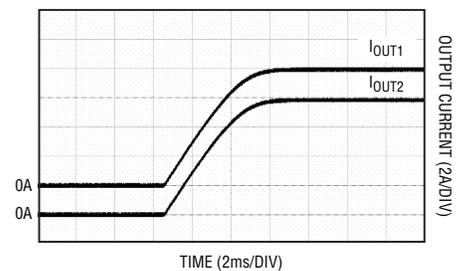
Figure 5. Balanced current sharing for even heat dissipation [5V<sub>IN</sub> to 1.8V<sub>OUT</sub> at 16A]
