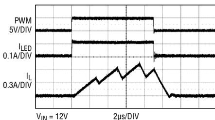
Figure 2. Integrated PWM dimming yields 1000:1 dimming at 120Hz
