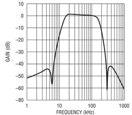
Figure 1. Filter response for a 15kHz-150kHz passband
