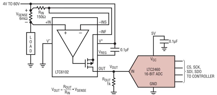
**Figure 1. A simple and compact high side current sensing solution that combines a high resolution  $\Delta\Sigma$  ADC (LTC2460) with a high precision current sensing amplifier (LTC6102).**
