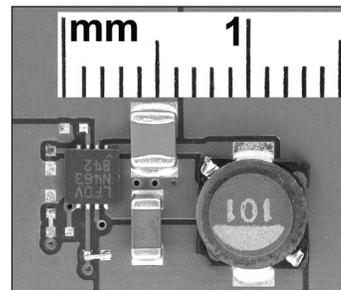
Figure 2. The solution size of LTC3642-3.3/5 in a 3mm × 3mm DFN package
