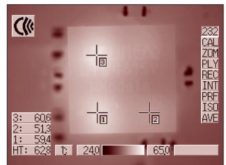
**Figure 10.** Top view thermal imaging of the unit at full load in an ambient temperature environment with no airflow. Cursors 1 and 3 mark the temperature hot spots on the unit for each of the two switching regulators. Both temperatures are fairly similar indicating balanced thermal conductivity.
