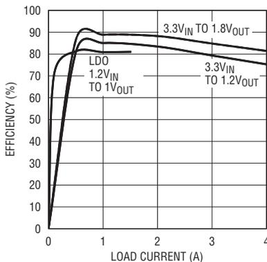
**Figure 8.** Efficiency of the circuit in Figure 7
