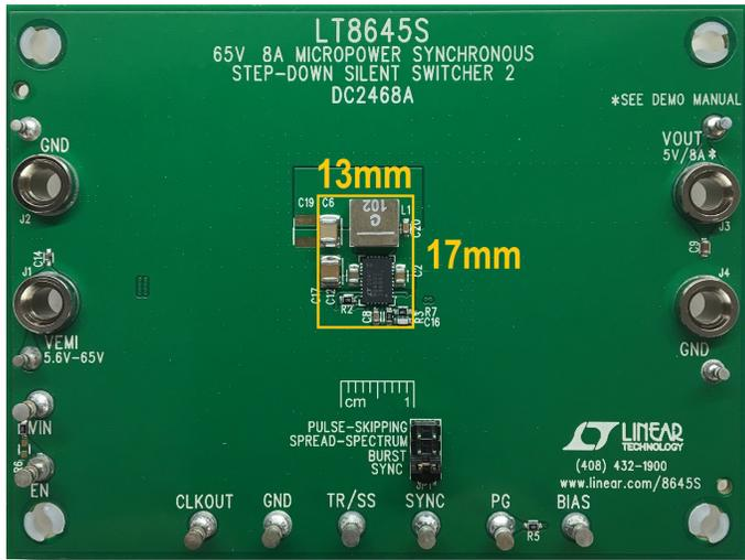
Figure 12. Small solution size of LT8645S demonstration circuit
