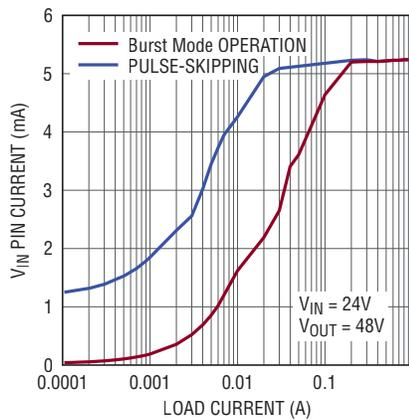
(b) Pulse-skipping and Burst Mode operation light load  $V_{IN}$  pin current
