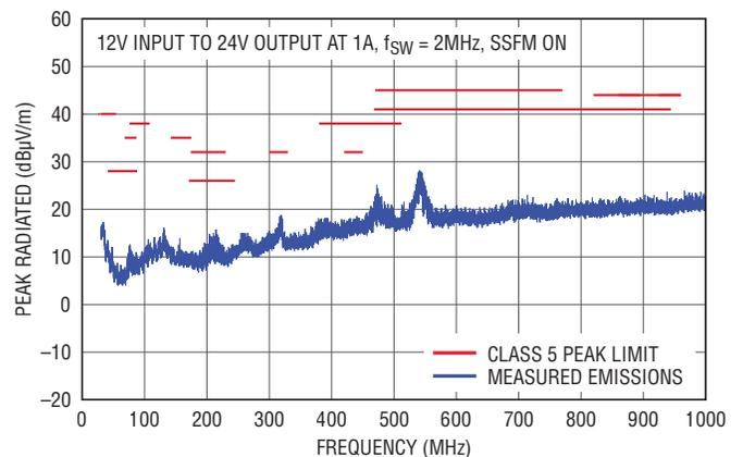
Until recently, selecting SSFM mode for low EMI meant using the less efficient pulse-skipping mode at light load. The LT836x family does not require this trade-off.
