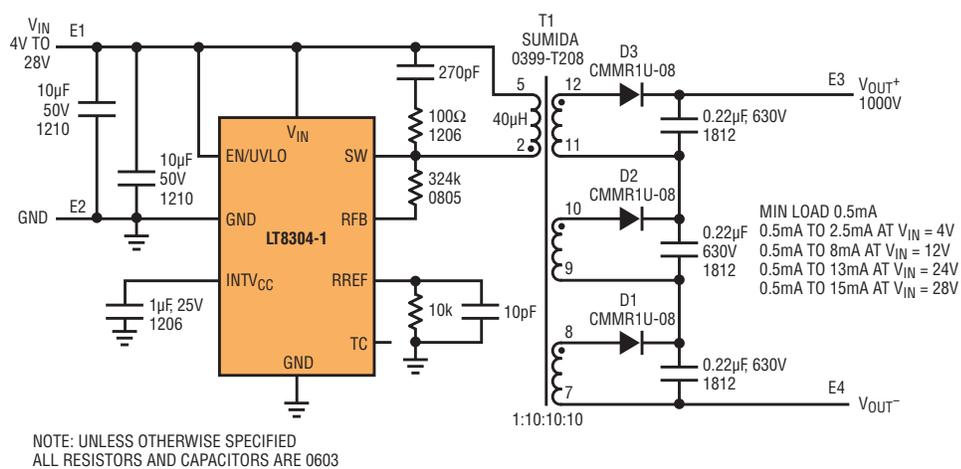
Figure 1. A complete 1000V/15mA isolated flyback converter from a 4V–28V input
