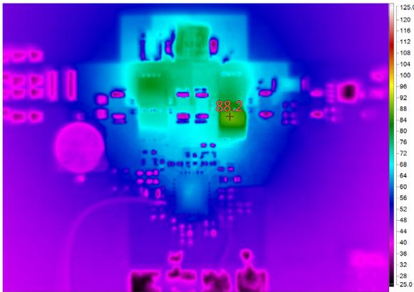
Figure 3. While generating 45W of output power, this small circuit's greatest temperature rise is only 65°C above ambient.
