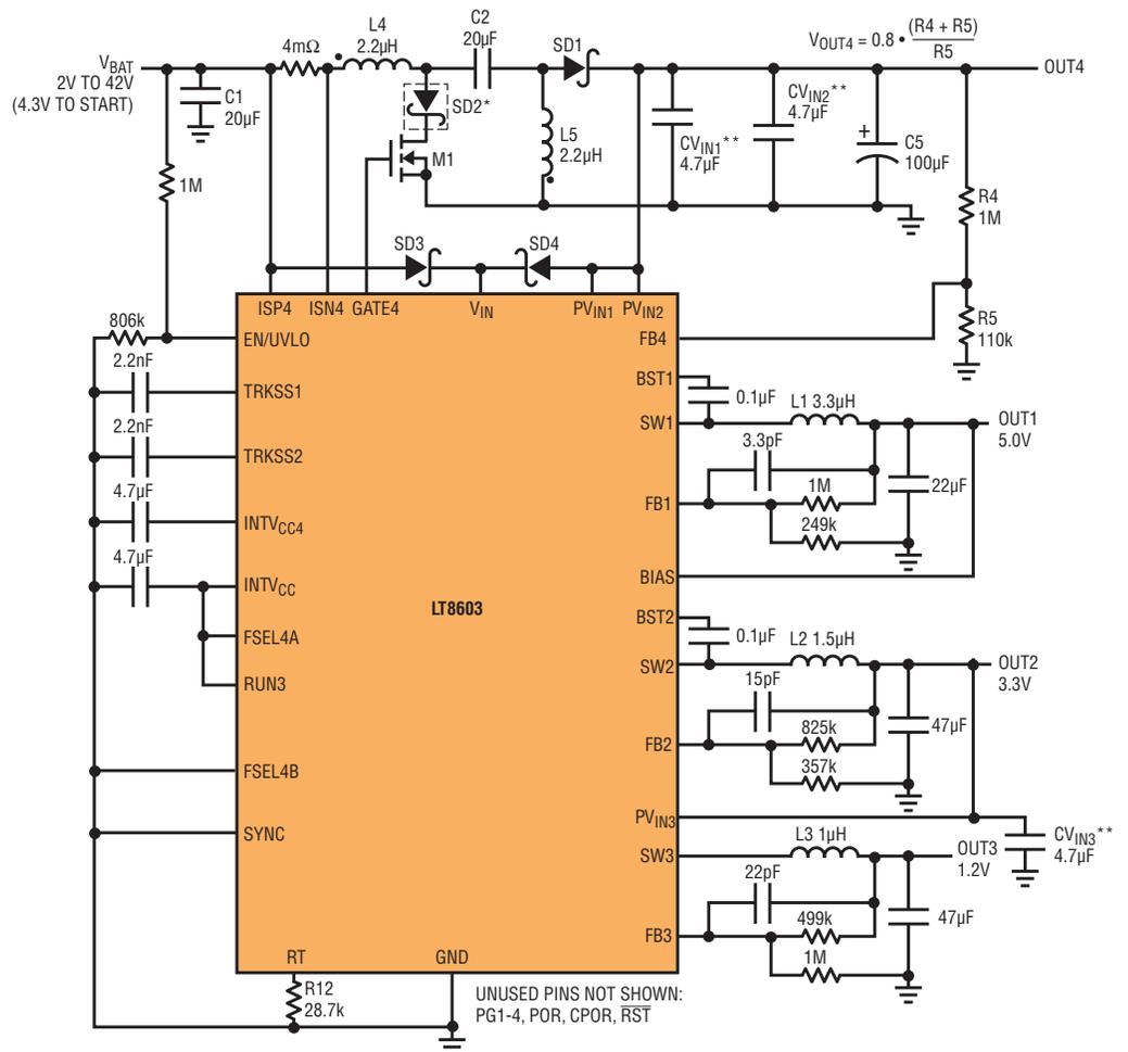
Figure 2. High voltage bucks optimized for efficiency; powered by a SEPIC
