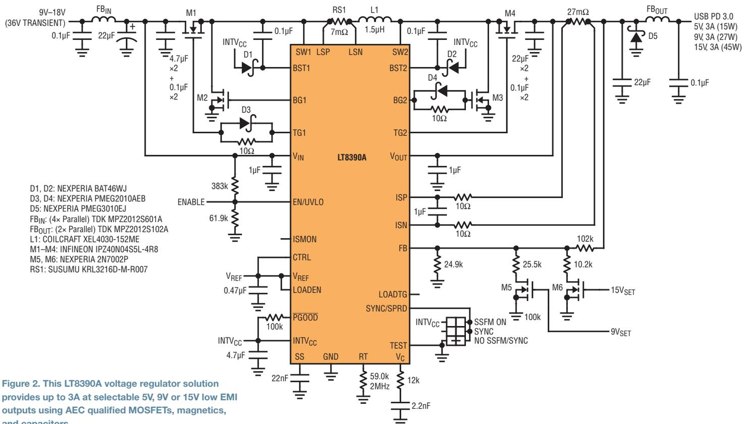
Figure 2. This LT8390A voltage regulator solution provides up to 3A at selectable 5V, 9V or 15V low EMI outputs using AEC qualified MOSFETs, magnetics, and capacitors.
