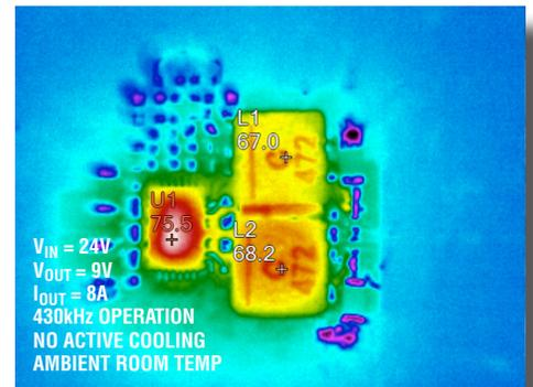
Figure 4. Thermal performance of the circuit in Figure 3
