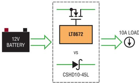
Figure 3. System configuration for thermal performance comparison
