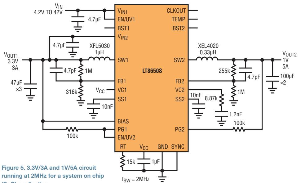
Figure 5. 3.3V/3A and 1V/5A circuit running at 2MHz for a system on chip (SoC) application
