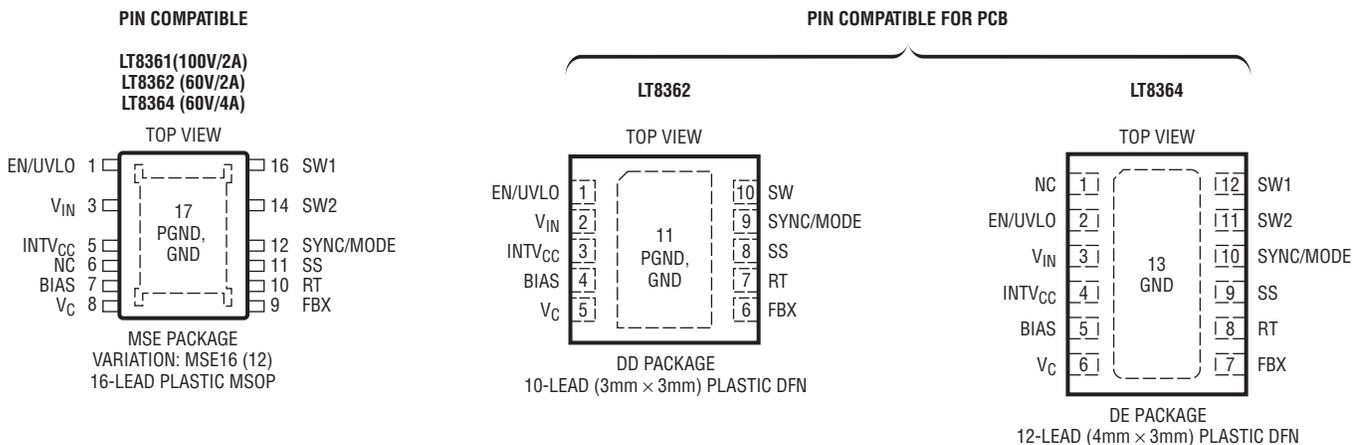
By offering a single FBX pin that allows for both positive and negative output voltages, all topologies are within reach. An inverting application is just as accessible as that of a boost or SEPIC, reducing design time and effort.
