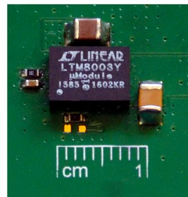
the regulator and the internal layout of the  $\mu$ Module are designed so that the input loop of the regulator is minimized. This significantly reduces the switching node ringing and the associated energy stored in the hot loop, even with very fast switching edges. This quiet switching offers excellent EMI performance, while minimizing the AC switching losses, allowing the regulator
