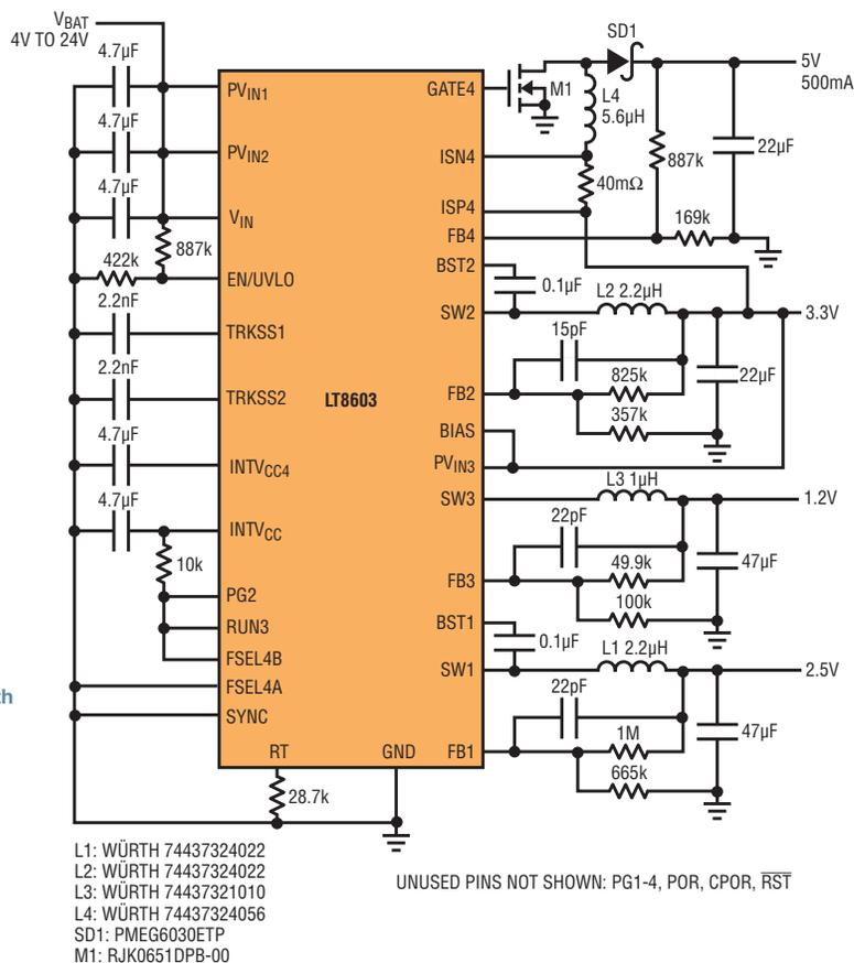
controller simply works as diode through. The high voltage bucks can handle  $V_{BAT}$  up to 42V. In Figure 1, the low voltage buck is powered from OUT2, providing 1.2V through the cold crank event.
