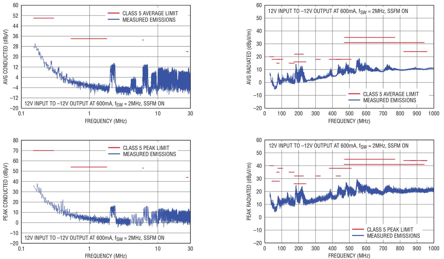
Figure 11. EMI test results for LT8362 inverting solution
