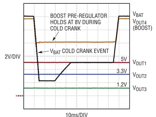
Figure 1. Cold crank tolerant automotive supply with three regulated outputs. Three bucks are powered with a boost pre-regulator ( $V_{OUT4}$ ), yielding precise regulation for all three outputs through a  $V_{BAT}$  cold crank event, also shown.
