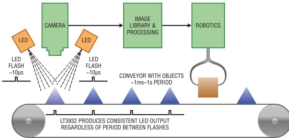
Figure 3. An example of machine vision on an industrial conveyor belt. Inspection systems move at many different speeds, yet the flash technology must be fast and crisp.
