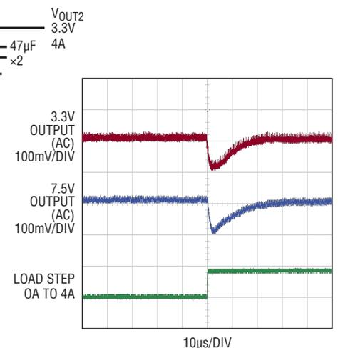
Figure 2. 0A to 4A transient responses of the circuit in Figure 1 (Burst Mode<sup>®</sup> operation)
