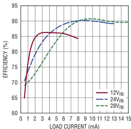
Figure 2. Efficiency of Figure 1 at various input voltages
