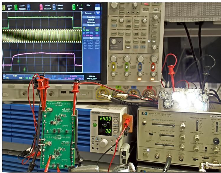
Figure 4. Two DC2286A LT3932 demo circuits are easily connected in parallel to create the 3A (to 4A) machine vision LED flash application shown in Figure 1.
