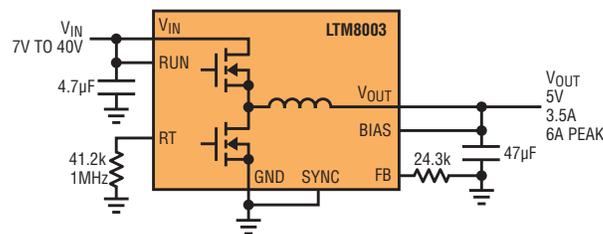
PINS NOT USED IN THIS CIRCUIT: TR/SS, PG
