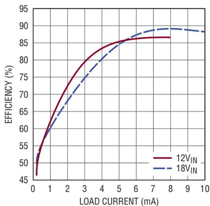
Figure 5. Efficiency of the solution in Figure 4 at various input voltages
