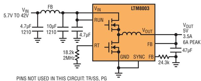
The internal regulator is capable of safely delivering up to 6A of peak output current, and no extra thermal management—airflow or heat sink—is required for the LTM8003 to continuously support a 3.5A load at 3.3V or 5V from a nominal 12V input. This meets the needs of the battery powered applications in industrial robotics, factory automation and automotive systems.
