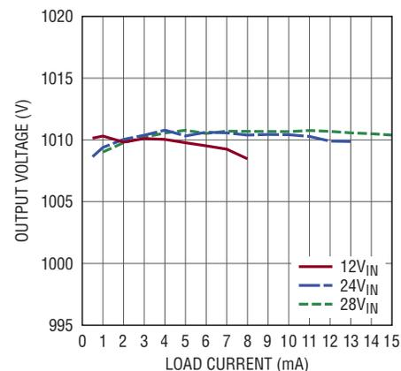
Figure 3. Load regulation of Figure 1 at various input voltages
