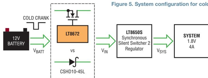
Figure 5. System configuration for cold crank test
