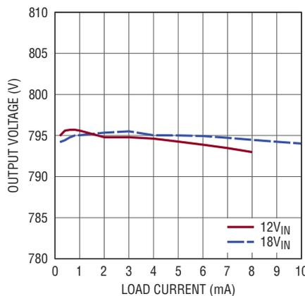
Figure 6. Load regulation of the solution in Figure 4 at various input voltages
