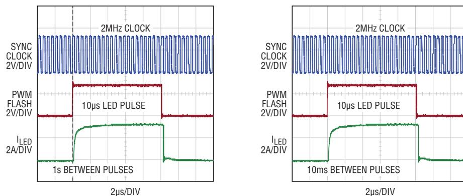
Figure 2. 3A camera flash waveform of Figure 1 parallel LED drivers looks the same regardless of the amount of PWM off-time. Waveforms show that a 10µs pulse looks the same after one second or 10ms. The LT3932 LED flash also looks the same after a day or longer of PWM off-time.
