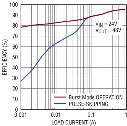
(a) Pulse-skipping and Burst Mode operation light load efficiency
