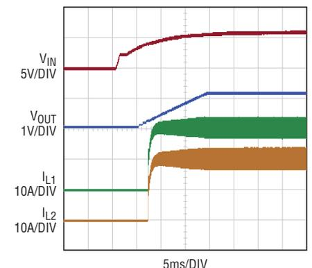
Figure 6. Inductor current waveforms for the parallel solution.
