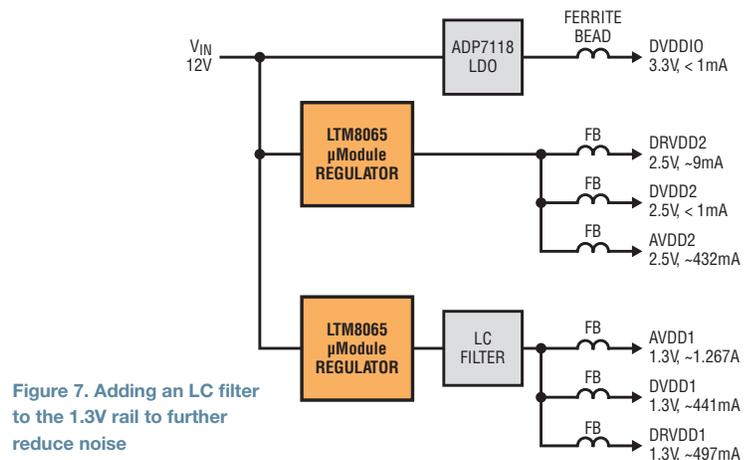
Figure 7. Adding an LC filter to the 1.3V rail to further reduce noise
