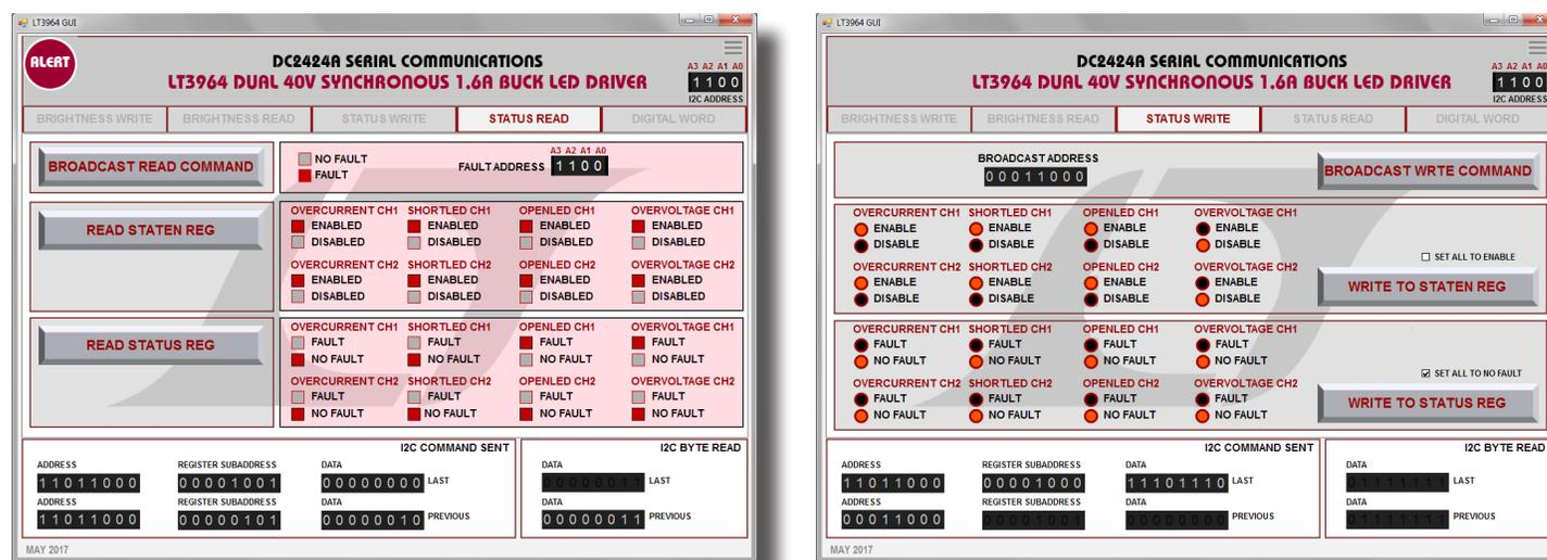
Figure 12. I<sup>2</sup>C registers include fault protection setting and reading. The LT3964 can report faults for each channel via its ALERT pin and I<sup>2</sup>C STATUS registers. The faults are only reported if the STATUS registers are individually enabled and a fault has occurred. Open LED, short LED, overcurrent, and overvoltage feedback faults for both channels can be enabled, reported, and read. They can also be disabled and ignored. .
