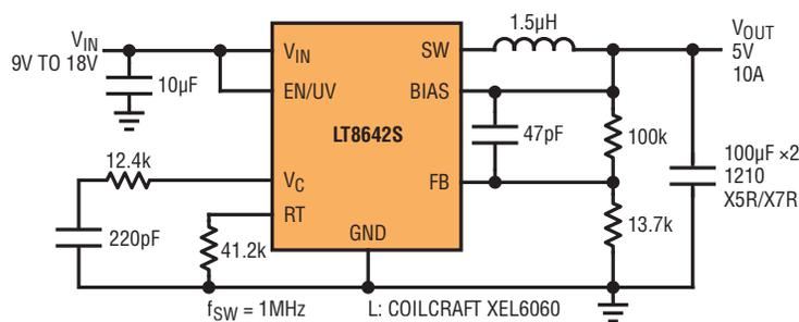
Figure 7. 50W (5V/10A) solution using the LT8642S
