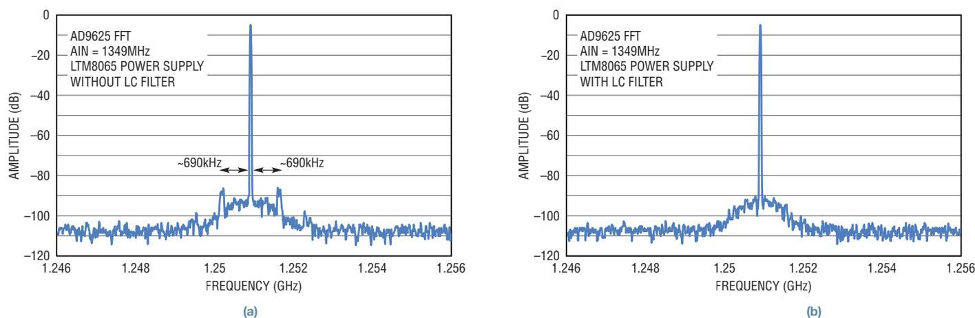
Figure 8. The effects of the LC filter on the modulation spurs around the 1349MHz carrier frequency can be seen by comparing AD9625 FFT results using two different power systems: a  $\mu$ Module regulator based power system without an LC filter (a) and one with the additional LC filter (b)
