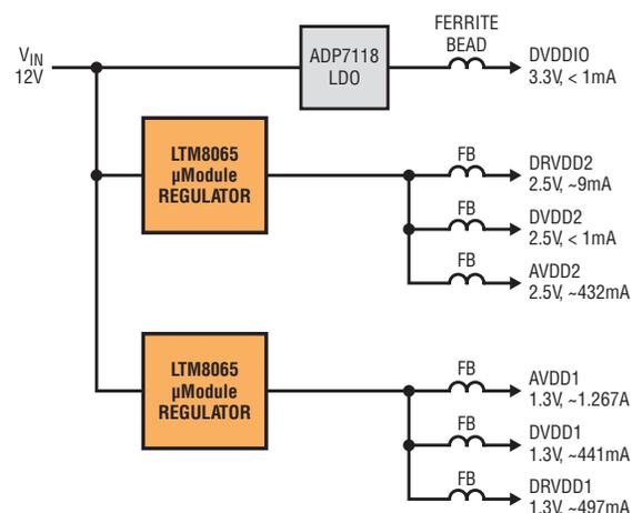
Figure 2. An alternative to the conventional switchers + LDOs power system shown in Figure 1. This design features two LTM8065  $\mu$ Module Silent Switcher regulators directly powering an AD9625. This design is quiet, more compact and more efficient. (LTM8065 unfiltered design)
