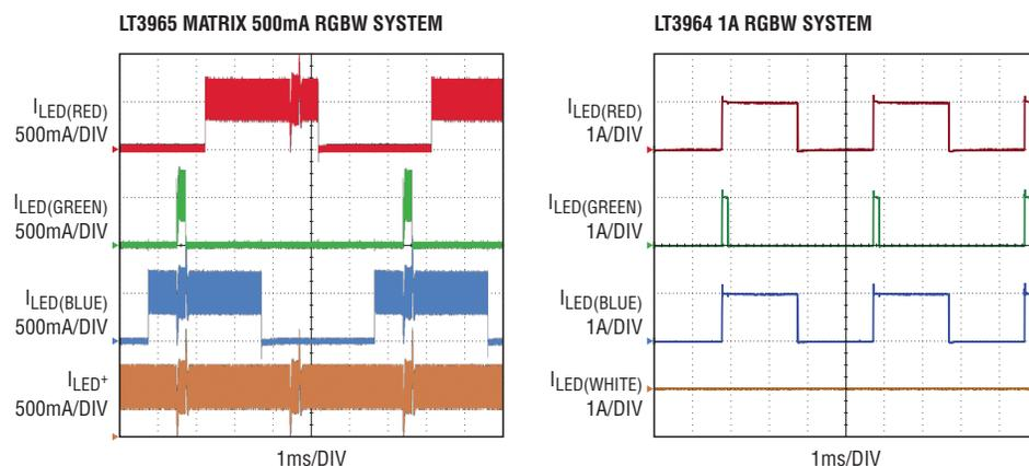
Figure 6. The 4-channel, two dual buck LED driver solution has low ripple current in contrast to the higher ripple matrix LED dimmer solution. The LT3964 presents a cleaner LED current waveform than the dimmer solution.
