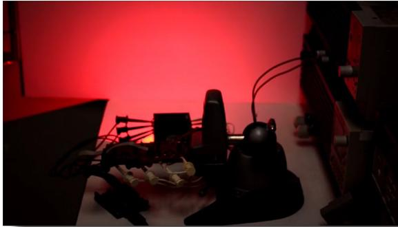
Complete digital control over high power RGBW LEDs using the LT3964 dual buck driver with I<sup>2</sup>C serial communications. Two LT3964s are enough to drive a single RGBW LED—or string of RGBW LEDs—at 1A with accurate and precise dimming to produce predictably repeatable color content.
