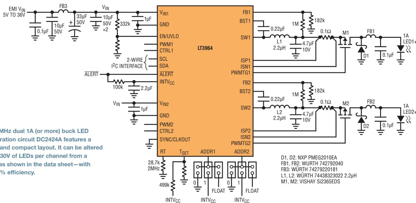
Figure 4. The 2MHz dual 1A (or more) buck LED driver demonstration circuit DC2424A features a high efficiency and compact layout. It can be altered to power up to 30V of LEDs per channel from a 34–36V input—as shown in the data sheet—with greater than 90% efficiency.
