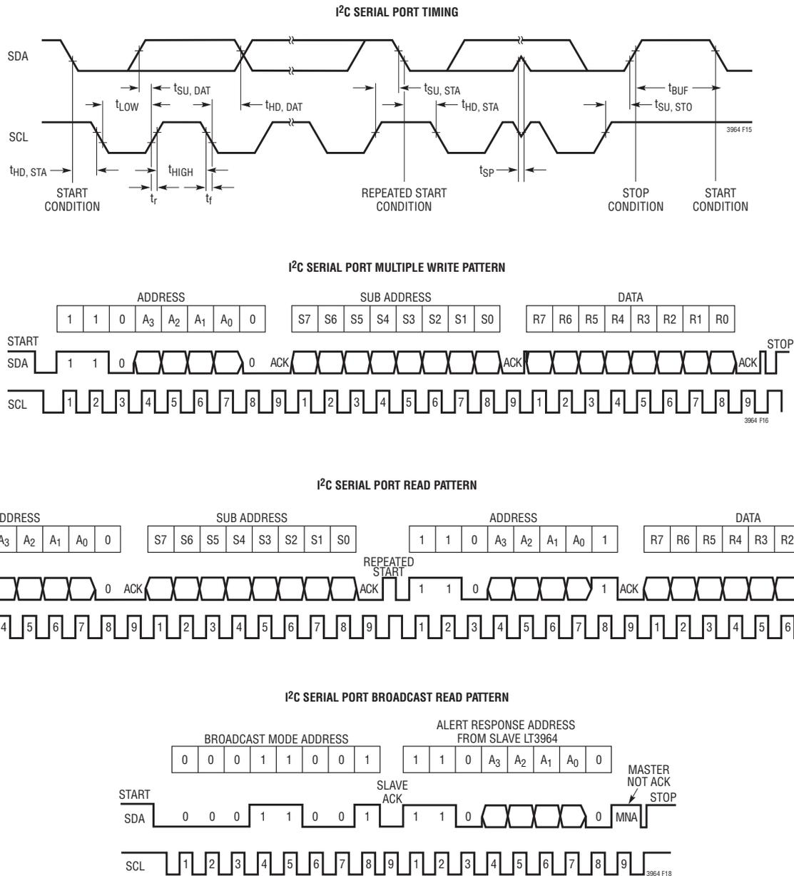
Figure 8. The LT3964 I<sup>2</sup>C serial communications use standard I<sup>2</sup>C WRITE and READ words.
