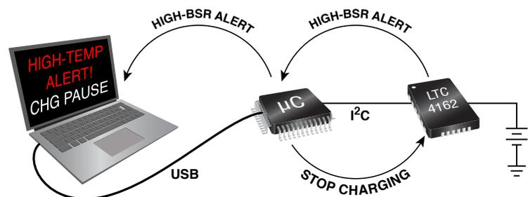
The LTC4162 enables customizable temperature dependent charging. For lithium-based chemistries (Li-ion and  $\text{LiFePO}_4$ ), the LTC4162 can employ JEITA temperature-controlled charging. Similarly, for lead-acid batteries, a temperature compensation algorithm linearly decreases the target voltage in each charging stage as temperature rises.
