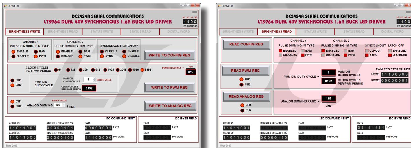
Figure 9. LT3964 features 13-bit (1:8192) PWM dimming capability with I<sup>2</sup>C. The PWM dimming duty cycle and frequency are set by writing to the two PWM dimming registers for each channel. Here, channel 2 is set to 1:8192 dimming while channel 1 is set to 128:256 analog dimming.
