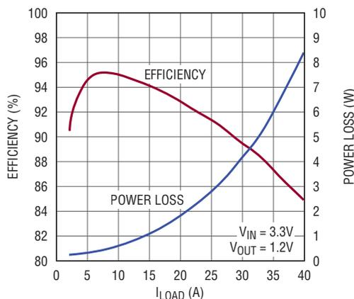
Figure 5. Efficiency of the 40A circuit in Figure 4.
