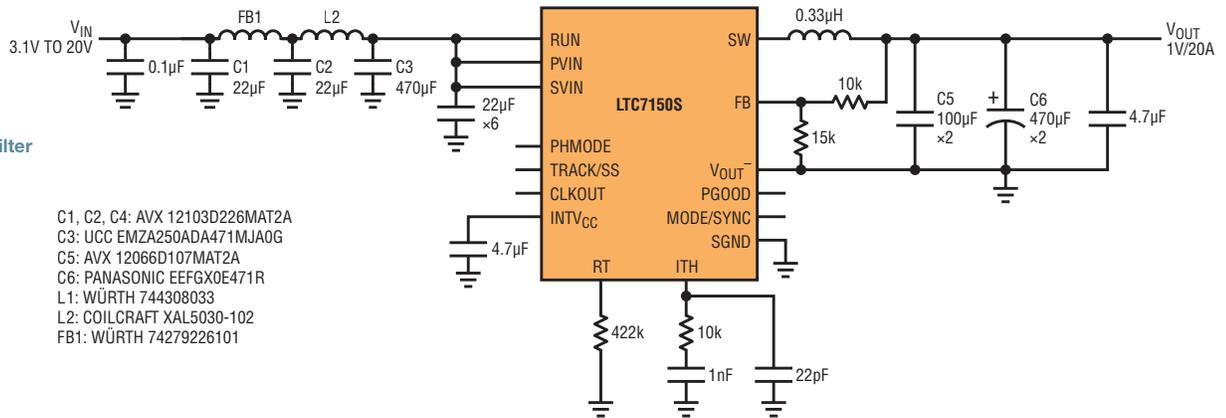
Figure 2. LTC7150S with EMI filter
