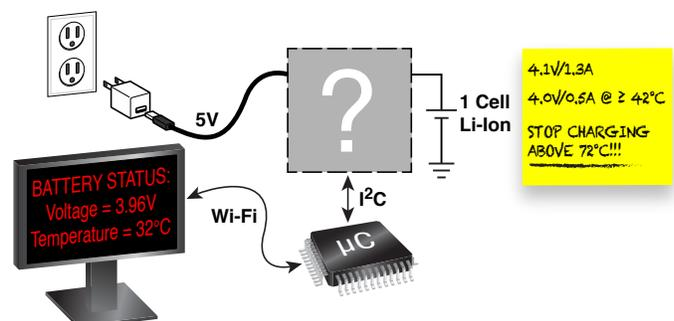
Although the LTC4162 can operate without a host controller, many aspects of charging can be monitored and controlled through the I<sup>2</sup>C port. An on-chip telemetry system reads system and battery voltages and currents in real time.
