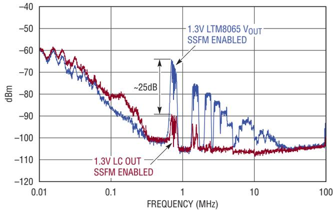
Figure 10. LTM8065 spectral content at the 1.3V rail with SSFM on and off
