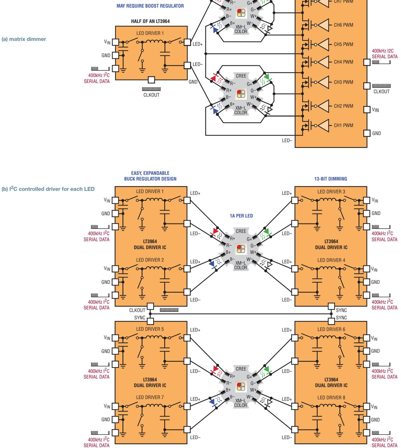
Lighting systems with a large number of RGBW LEDs require a substantial number of drivers, and synchronization of the control signals to those drivers. The highest performance approach is to directly control each component LED with its own high performance LED driver.
