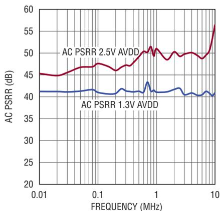
Figure 6. Power supply rejection ratio of the AD9625 analog power supply inputs
