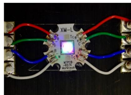
Figure 1. Cree XM-L RGBW high power LED can be driven by two LT3964 LED drivers for accurate 1:8192 per-channel dimming.
