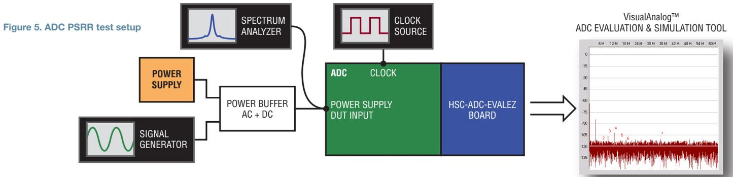
Calculating the AC PSRR at 1MHz using the equation 1 yields an AC PSRR of 41dB.
