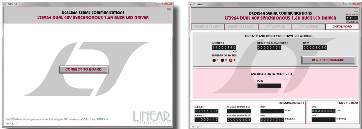
Figure 11. The LT3964 DC2424A demonstration circuit can be controlled with a free GUI through QuikEval. On each page, the register elements can be set and then I<sup>2</sup>C WRITE or READ commands can be sent with the press of a button through USB and a Linduino DC2026C demonstration circuit. The IC address bits can be set for any address and the GUI can communicate to many LT3964 ICs at once.
