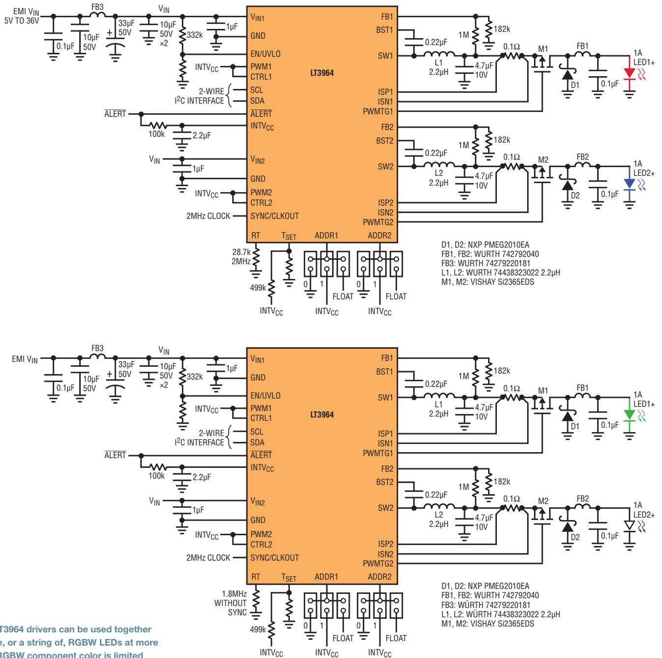
Figure 5. Two LT3964 drivers can be used together to drive a single, or a string of, RGBW LEDs at more than 1A. Each RGBW component color is limited by the dimming resolution, typically 1/256, or 8-bit resolution. Much higher resolution is available with a LT3964-based solution can accomplish up to 1/8192, or 13-bit PWM dimming for each channel combined with 1/10 analog dimming—all controlled by I<sup>2</sup>C.
