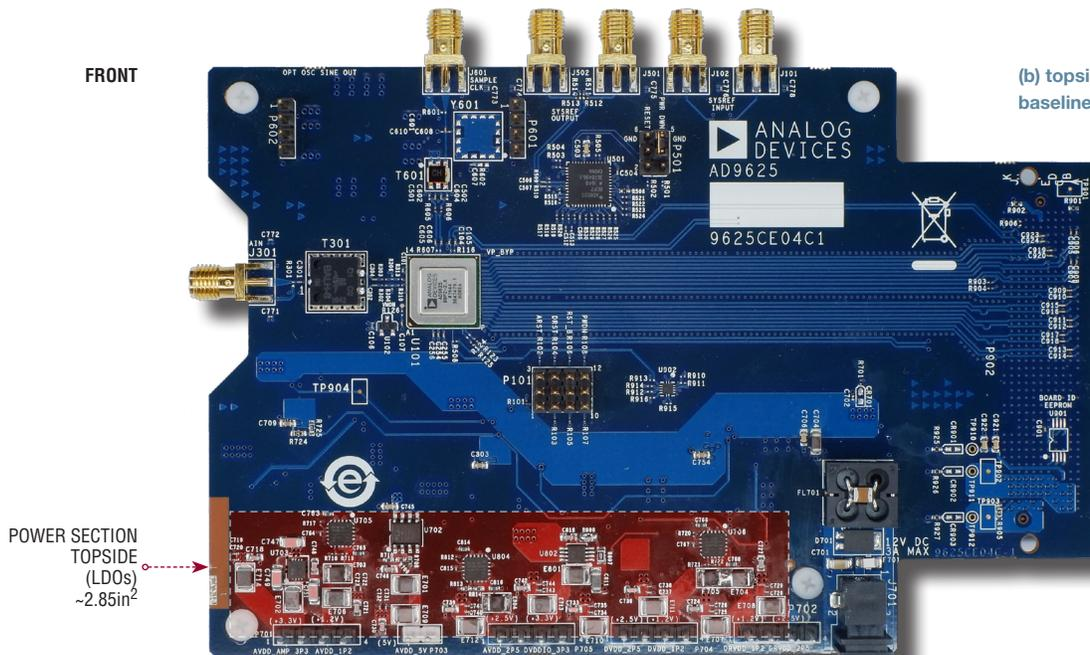
(b) topside and backside area required by baseline power supply design
