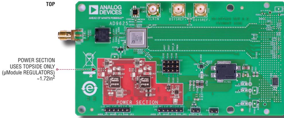
Figure 13. The area needed for a power supply is greatly reduced when using µModule Silent Switcher regulators in place of conventional controllers/regulators. The AD9625 revised demo board with LTM8065 (a) is compared to an off-the-shelf AD9625 evaluation board (b). The power supply sections of both systems are highlighted.
