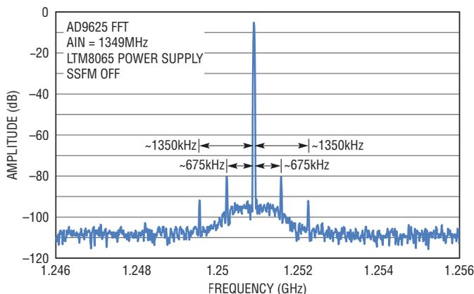
Figure 11. Detail of 1349MHz analog input carrier with SSFM disabled for the LTM8065 1.3V rail
