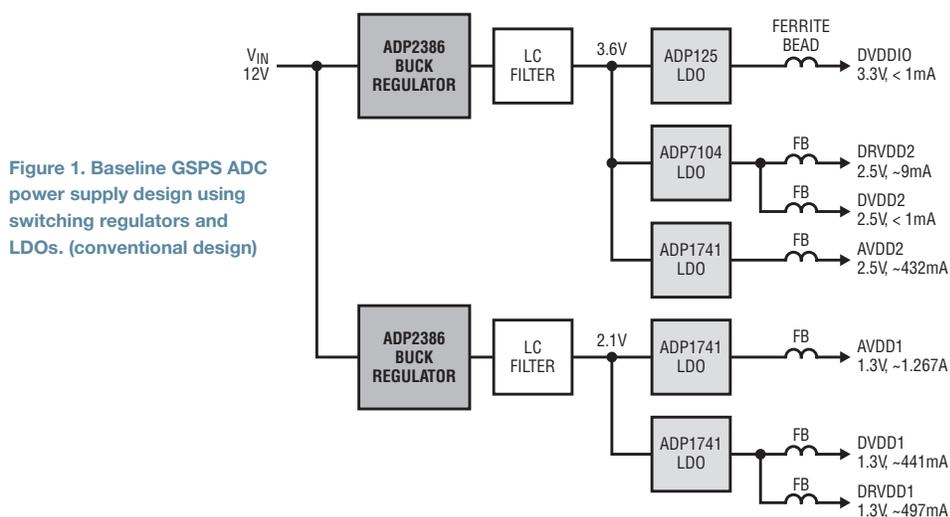
Figure 1. Baseline GSPS ADC power supply design using switching regulators and LDOs. (conventional design)
