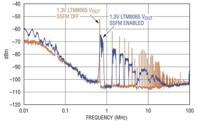
to those of the baseline power supply. The data shows that LTM8065 can directly power the AD9625 without the use of additional LDOs, greatly simplifying the overall solution.
