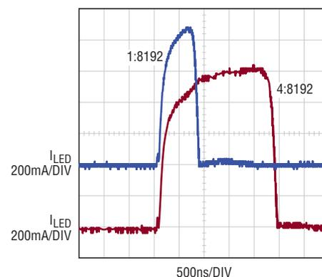
Figure 10. I<sub>LED</sub> waveform showing 1:8192 dimming
