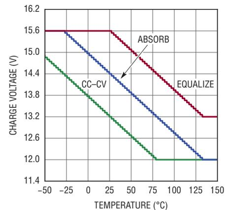
Figure 5. Default 12V lead-acid temperature profile.
