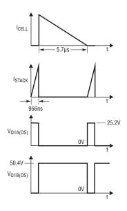
Figure 2. Discharge mode of a single cell in the stack
