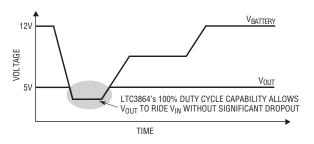
dropout during a cold crank condition. Figure 2 shows how the regulated 5v output drops out and recovers during a cold crank condition. The output simply tracks the input voltage under the output regulation voltage. The output quickly recovers to the regulated 5v once the cold crank condition is over.
