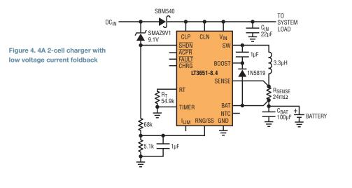
The LT3651 is a versatile, compact and easy-to-use solution for charging Li-ion batteries with up to 4A in current and from input supplies up to 32V (40V ride through). High efficiency, built in safety controls and compact size make it an easy fit in a wide variety of applications.
