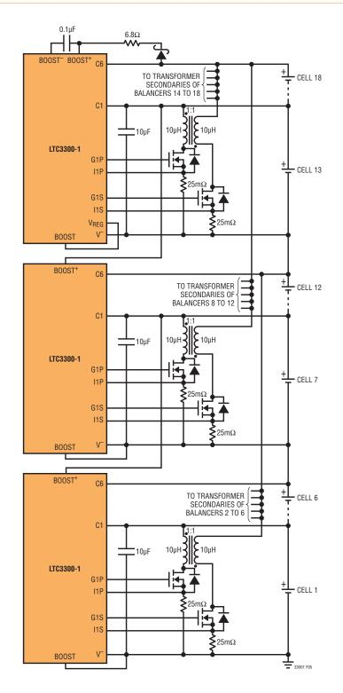
Figure 7. 18-cell active balancer
