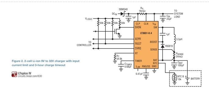
based on battery voltage. During constantcurrent operation, the maximum charge current provided to the battery is programmable via a sense resistor, up to a maximum of 4A and adjustable using the RNG/SS pin. Charge current is internally reduced as the battery approaches the fullcharge float voltage and the charger transitions to constant voltage charging mode.
