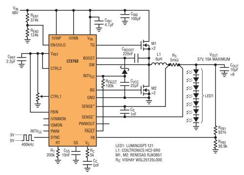
The LT3763 is a versatile step-down buck converter that integrates many complex features essential for LED drivers, solar harvesters and battery chargers. A PWM driver and current monitors are included with fault detection, current limiting, input and output voltage regulation.
