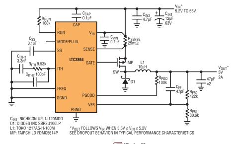
Figure 4. Typical 5V output automotive application
