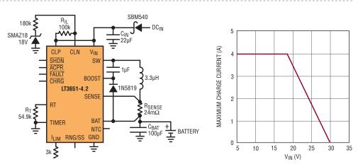
Figure 3. 4A single cell charger with high voltage current foldback
