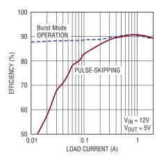
Figure 1. LTC3864 pulse-skip and Burst Mode efficiency
