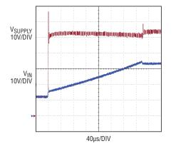
Figure 6. Fast  $V_{\text{SUPPLY}}\,\text{dV/dt}$  is blocked from  $V_{\text{IN}}$  by series MOSFET and gate network
