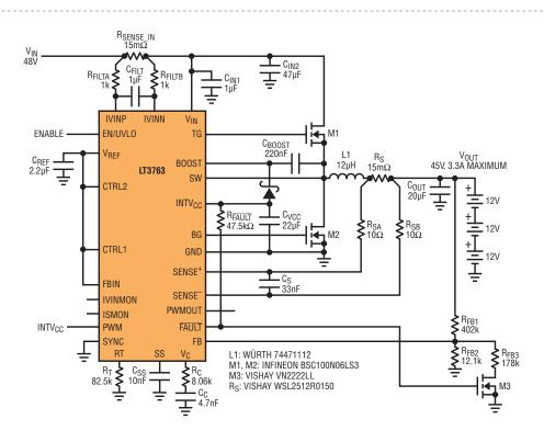
Figure 4. 3.3A, six-cell (36V) SLA battery charger
