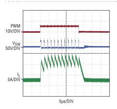
Figure 2. PWM dimming performance of the circuit in Figure 1
