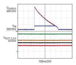
Figure 4. Overvoltage protection withstands 180V surge
