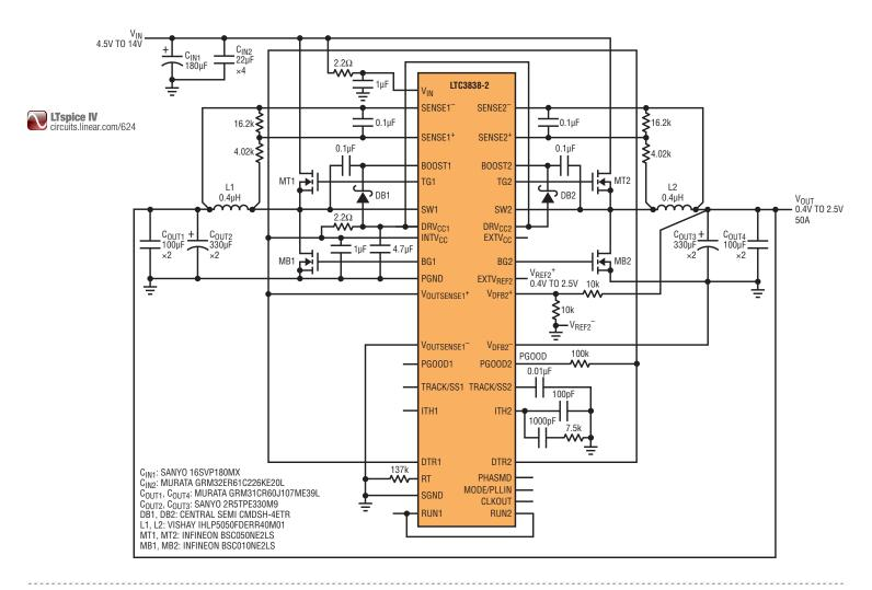
In addition to regulation accuracy, the LTC3838-2 offers widebandwidth tracking to a dynamic external reference. Tracking bandwidth is important in applications like dynamic voltage scaling because bandwidth determines how quickly the supply can respond to changes to the programmed external reference.
