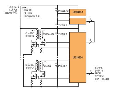
Figure 1. Simplified schematic of how the LTC3300-1 actively balances individual cells in a 12-cell battery stack With the LTC3300-1, all individual cell balancers can operate simultaneously, in any combination of discharge or charge modes, even when multiple LTC3300-1 devices are used. For instance for a stack of 12 cells, with two LTC3300-1 devices connected in series, charge can be transferred from cell 12 to cell 1 in a single time step by discharging cell 12 and charging cell 1.
